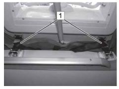
Fig. 188: Roof locking mechanisms
