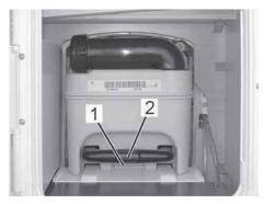
Fig. 193: Waste holding tank in the disposal shaft
