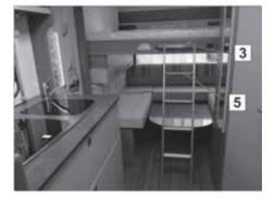
**4.** Position the ladder (5) and hook onto the pull-grip (3).
