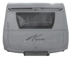
Fig. 73: Gas bottle locker, sealed
