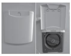
Fig. 90: Fresh water intake port
