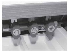
Fig. 78: Quick-closing valves
