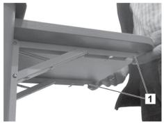
Fig. 182: Undoing the latching mechanism
