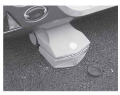
Fig. 110: Wheeled waste water tank
