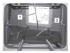
Fig. 186 Pulling rope (1), Expansion bellows (2)
