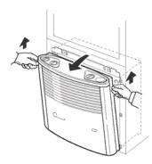
Fig. 130: Opening the heater grille
