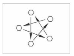
Fig. 210: Always tighten tyre nuts and bolts crosswise
