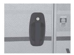
■ To open the entry door, unlock the door lock with the key, reach into the recessed grip and and pull the door to the outside.
