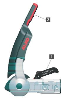
Fig. 5: Tow-ball coupling open
