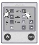
Fig. 162: Temperature setting
