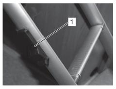
Fig. 185: Locking mechanism (1) of the access ladder
