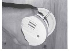
Fig. 216: Removing the housing
