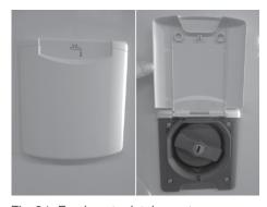
Fig. 21: Fresh water intake port
