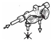
Fig. 79: Shut-off and release position
