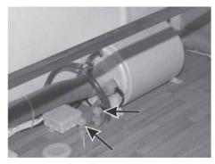
Fig. 97: TRUMA water heating and water drain valves
