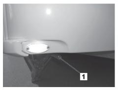
Fig. 10: Hexagon opening (1) for socket wrench
