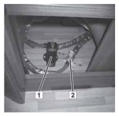
Fig. 106: TRUMA combination heater drain valves
