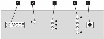
Fig. 207: Control elements on the refrigerator with automatic ignition
