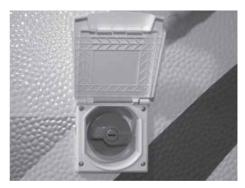
Fig. 91: Fresh water intake port
