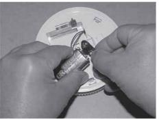
Fig. 217: Replacing the block battery
