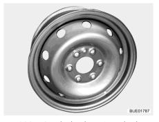
Fig. 299 Steel wheel rim (standard)
