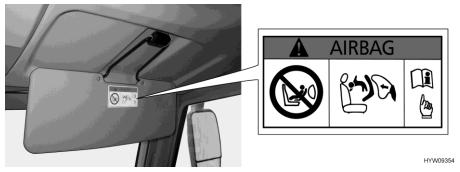
Fig. 20 Warning notice on child restraint system (front passenger's seat sun visor)
