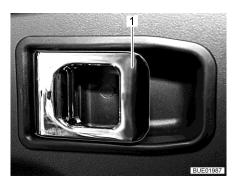
Fig. 71 Door lock (driver's door, inside)
