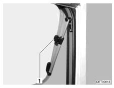
Fig. 114 Hinged window with rotary hinge
