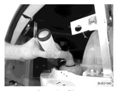
Fig. 55 Filler neck in filling position
