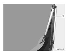
Fig. 115 Hinged window with automatic hinge
