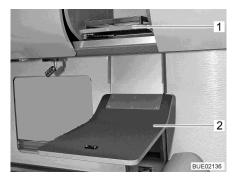
Fig. 92 Storage compartment with flap
