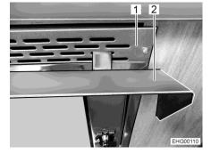
Fig. 230 Heat protection sheet (hooked in)
