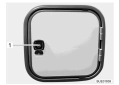
Fig. 265 Flap for sewage tank (alternative)
