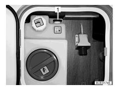
Fig. 253 Water tank with rotary handle in service unit
