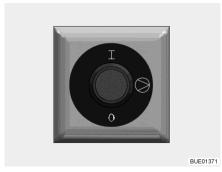
Fig. 216 Operating switch for auxiliary circulating pump
