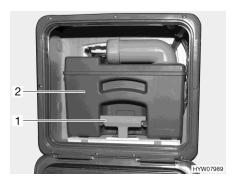
Fig. 275 Sewage tank (example)
