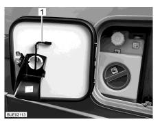
Fig. 261 Service flap with square spanner
