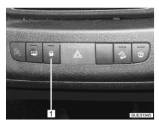
Fig. 69 Central locking system switch
