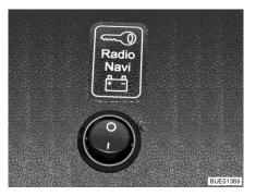
Fig. 178 Selector switch for operating behaviour
