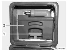
Fig. 266 Sewage tank (example)
