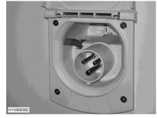
Fig. 189 230 V connection on the ve-
