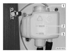
Fig. 280 Compensator reservoir without panel
