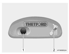
Fig. 271 Flush button/indicator lamp Thetford toilet
