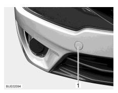
Fig. 59 Cover for the towing eye holder (example)
