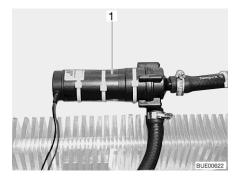
Fig. 215 Auxiliary circulating pump
