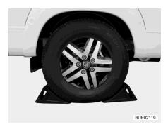
Fig. 303 Securing vehicle
