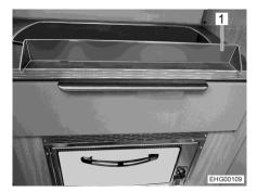
Fig. 229 Heat protection sheet (loose)
