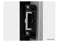
Fig. 242 Locking device in ventilation position
