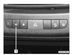
Fig. 43 External mirror heater switch
