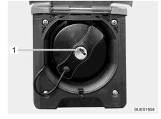
Fig. 56 Fuel filler neck external flap
