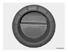
Fig. 204 Air outlet nozzle (hot-air heater)
