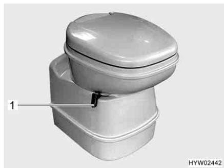
Fig. 177 Cuvette Thetford, orientable
