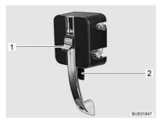
Fig. 44 Door lock of conversion door, inside
