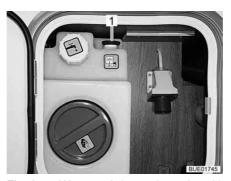
Fig. 247 Water tank (central supply unit)
