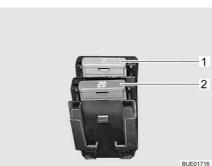
Fig. 179 Fuses for the pull-down bed
