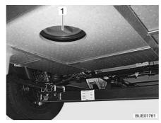
Fig. 268 Cleaning opening of the waste water tank
