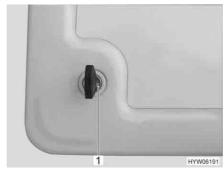
Fig. 52 Service flap push-button lock
