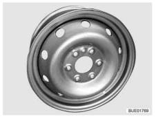
Fig. 279 Steel wheel rim (standard)
