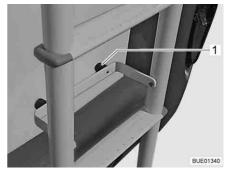
Fig. 1 Foldable ladder, ladder folded upwards
