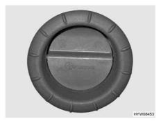
Fig. 192 Air outlet nozzle of the hot-air heater
