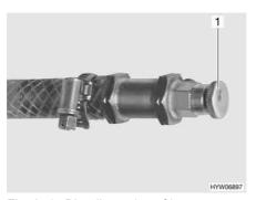
Fig. 271 Bleeding valve of hot-water heater
