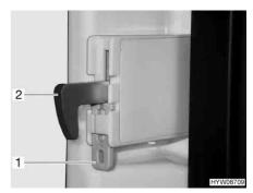
Fig. 233 Lock hook fixture
