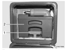
Fig. 257 Sewage tank (example)
