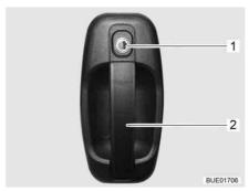
Fig. 46 Door lock of conversion door, outside
