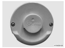
Fig. 207 Wall flue of the hot-air heater
