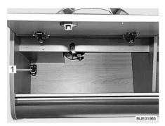
Fig. 182 Front pull-down bed fuse
