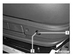
Fig. 27 Switch for seat heater
