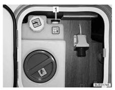
Fig. 246 Water tank (central supply unit)
