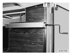
Fig. 120 Crank in the rear garage
