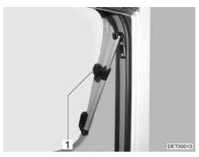
Fig. 80 Hinged window with rotary hinge
