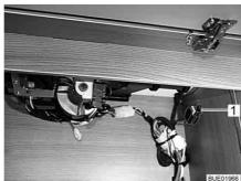
Fig. 183 Rear pull-down bed fuse
