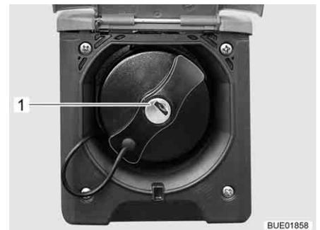
Fig. 49 Cap for the fuel filler neck
