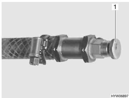
Fig. 262 Bleeding valve of hot-water heater
