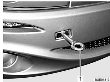
Fig. 51 Towing eye, mounted
