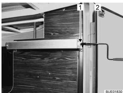
Fig. 147 Crank in the rear garage
