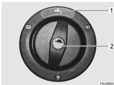
Fig. 77 Cap for the drinking water filler neck (Viseo)
