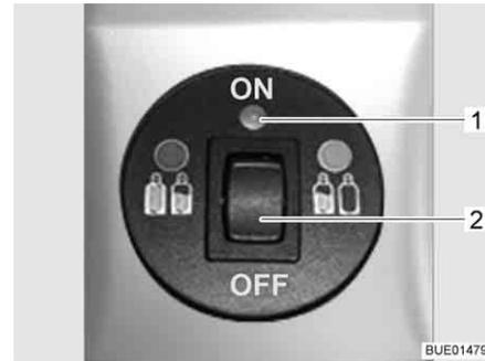
Fig. 157 Operating unit with remote display
