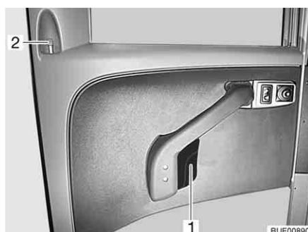
Fig. 65 Door lock of driver's door, inside (Viseo)
