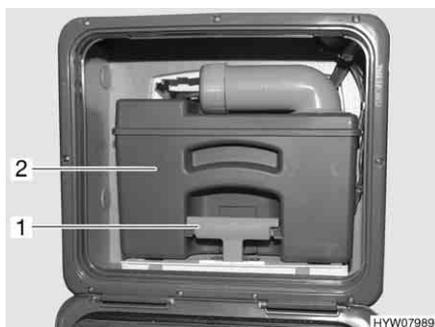
Fig. 256 Sewage tank (example)
