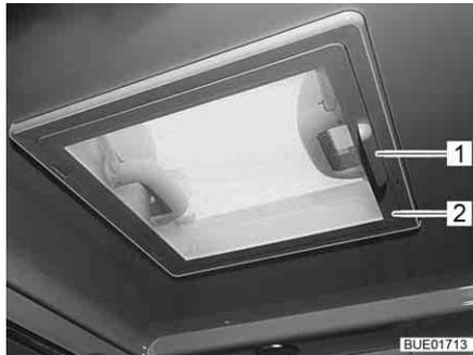
Fig. 129 Skylight with snap latch
