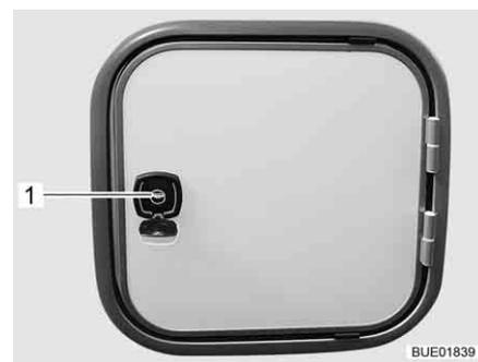
Fig. 246 Flap for sewage tank (alternative)
