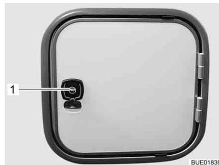
Fig. 255 Flap for sewage tank (alternative)
