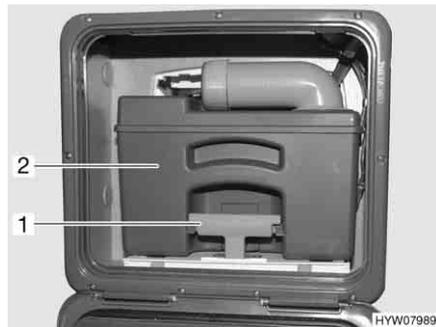
Fig. 247 Sewage tank (example)
