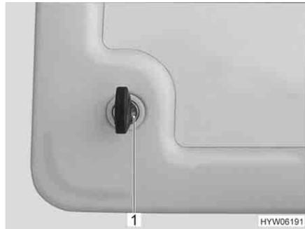
Fig. 74 Service flap push-button lock
