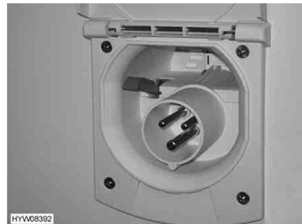
Fig. 168 230 V connection on vehicle
