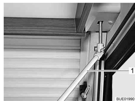
Fig. 124 Hand crank for emergency operation
