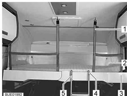
Fig. 142 Pull-down bed complete with applied safety net
