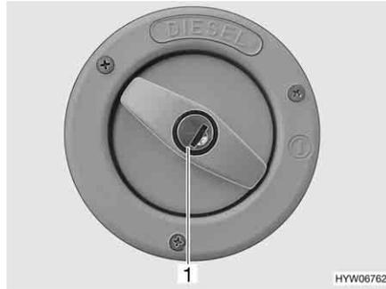
Fig. 47 Cap for the fuel filler neck
