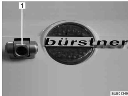
Fig. 22 Reversing camera with infrared illumination
