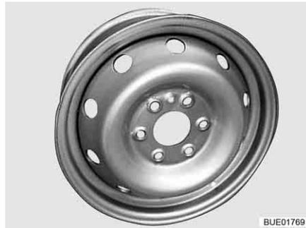
Fig. 278 Steel wheel rim (standard)
