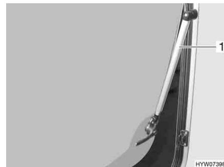
Fig. 110 Hinged window with automatic hinge
