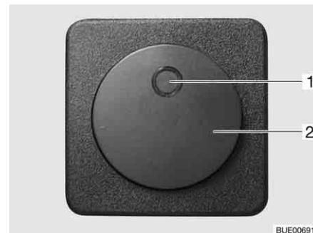
Fig. 203 Switch for electrical floor warming unit
