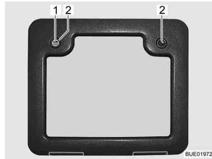
Fig. 75 Service flap push-button lock (alternative)
