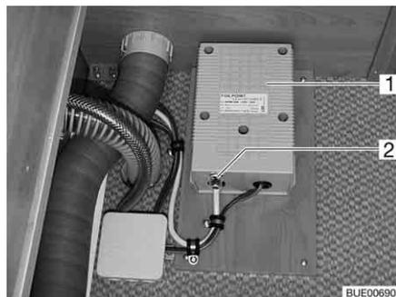
Fig. 202 Transformer for electrical floor warming unit
