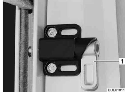
Fig. 21 Securing latch
