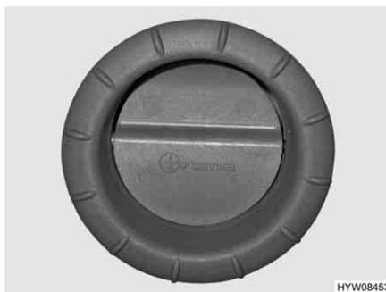
Fig. 184 Air outlet nozzle of the hot-air heater
