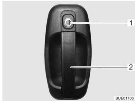
Fig. 67 Door lock of conversion door, outside
