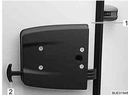
Fig. 72 Garage flap emergency release
