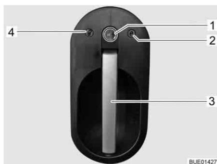
Fig. 64 Door lock of driver's door, outside
