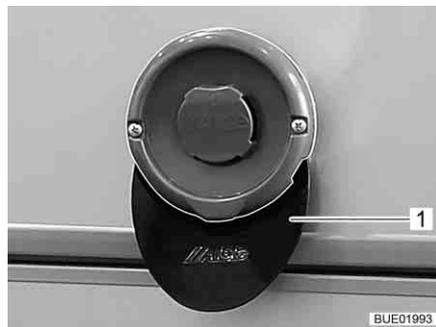
Fig. 201 Flue shield
