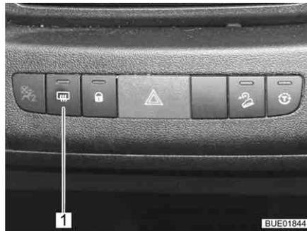
Fig. 38 Switch for the external mirror heater (Elegance)
