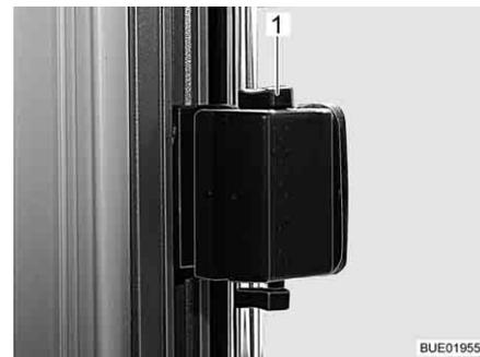
Fig. 114 Sliding window, unlocked
