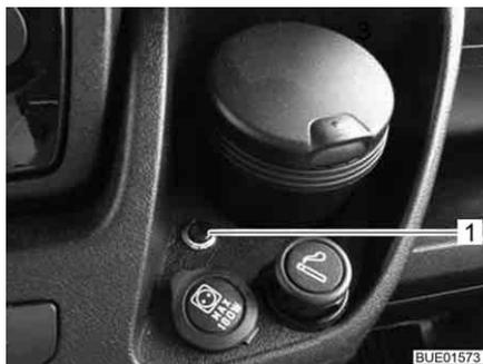
Fig. 55 Push-button to activate remote control
