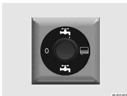
Fig. 241 Operating switch for electrically operated drainage valve (partially special equipment)
