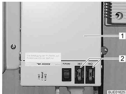
Fig. 173 Heater regulation for waste water pipes
