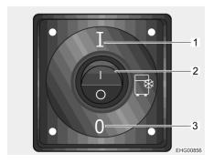
Fig. 54 On/Off switch for icebox
