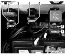
Fig. 45 Fuses for living area battery and other devices
