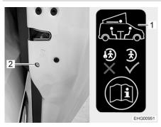
Fig. 5 Child safety lock on the sliding door
