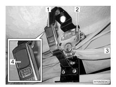
Fig. 26 Locking, elevating roof at the front (C 500)
