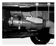
Fig. 61 Drain cock for waste water tank
