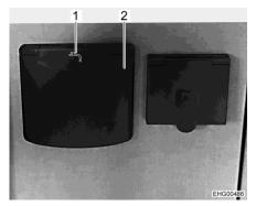
Fig. 59 Access flap to drinking water filler neck
