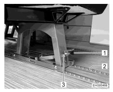
Fig. 7 Individual seat (locking device open)
