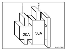
Fig. 46 Fuses for starter battery and charge booster
