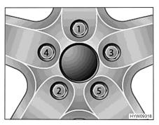
Fig. 67 Tightening the wheel nuts or wheel bolts cross-wise
