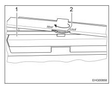
Fig. 56 Locking wheel on the refrigerator door
