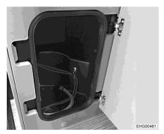
Fig. 39 Gas bottle compartment
