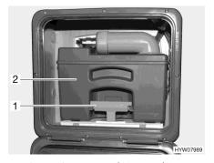
Fig. 65 Sewage tank (example)
