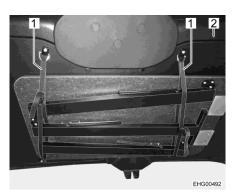
Fig. 14 Table (fastened to the rear flap) (C 500)
