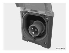
Fig. 43 230 V connection on the vehicle (CEE socket outlet)
