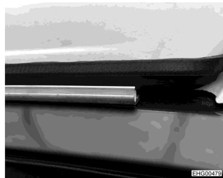
Fig. 9 Keder rail (detailed view)
