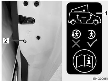
Fig. 5 Child safety lock on the sliding door
