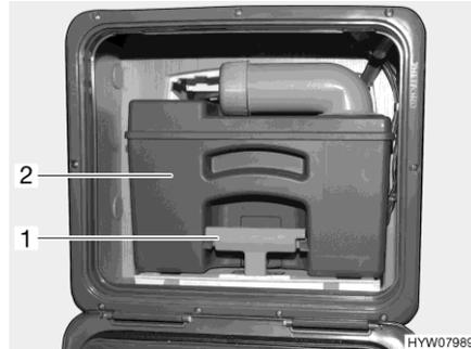
Fig. 65 Sewage tank (example)
