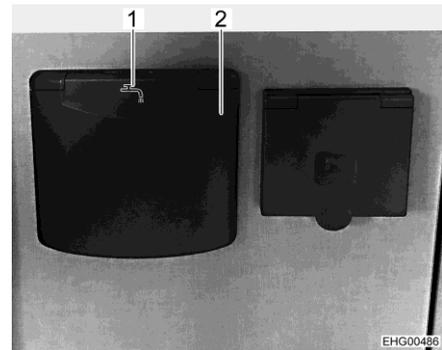
Fig. 59 Access flap to drinking water filler neck
