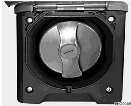
Fig. 58 Cap for the drinking water filler neck
