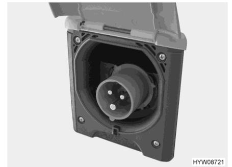
Fig. 43 230 V connection on the vehicle (CEE socket outlet)
