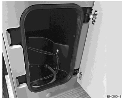
Fig. 39 Gas bottle compartment
