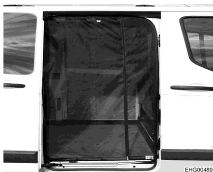
Fig. 10 Insect screen, sliding door
