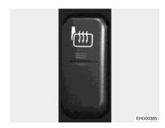
Fig. 28 External mirror heater switch
