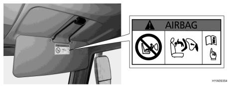
Fig. 14 Warning notice on child restraint system (front passenger's seat sun visor)
