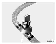
Fig. 148 Drain cock (with rocking lever)
