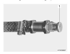
Fig. 157 Bleeding valve of hot-water heater
