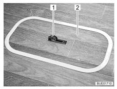
Fig. 65 Floor compartment cover (handle swung out)
