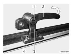
Fig. 82 Catch lever with safety knob in "continuous ventilation" position
