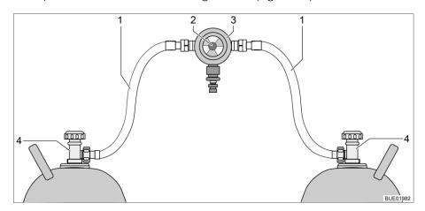
Fig. 102 Gas bottle switching facility
