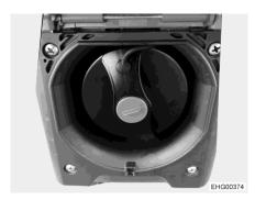
Fig. 59 Cap for the drinking water filler neck
