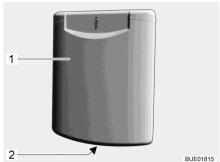
Fig. 58 Flap for the 230 V connection
