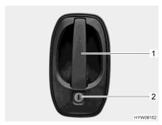
Fig. 49 Door lock (driver's door/conversion door, outside)
