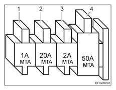
Fig. 114 Fuses (living area battery with charging booster)
