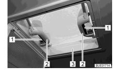
Fig. 91 Skylight with snap latch
