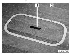
Fig. 64 Floor compartment cover (handle recessed)
