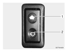
Fig. 25 Switch for electrical window winder
