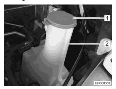
Fig. 37 Washer fluid container filler neck
