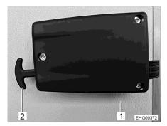
Fig. 55 Garage flap emergency release
