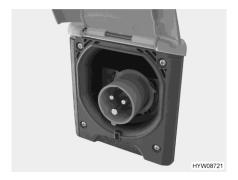
Fig. 111 230 V connection on the vehicle (CEE socket outlet)
