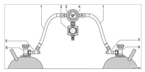
Fig. 11 Gas regulator with CPU and hose break guard
