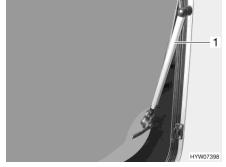
Fig. 81 Hinged window with automatic hinge
