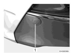
Fig. 40 Cover for the towing eye holder
