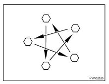
Fig. 168 Tighten the wheel nuts or wheel bolts cross-wise
