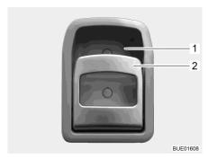
Fig. 51 Door lock (conversion door, inside)
