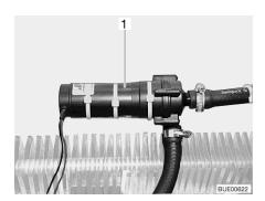
Fig. 128 Auxiliary circulating pump
