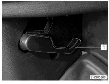
Fig. 35 Release lever for the bonnet (inside the vehicle)
