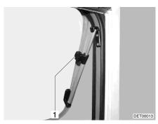
Fig. 80 Hinged window with rotary hinge
