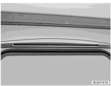
Fig. 67 Awning light (not when equipped with awning)
