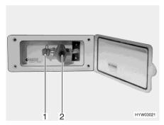
Fig. 101 External gas connection (gas isolator tap closed)
