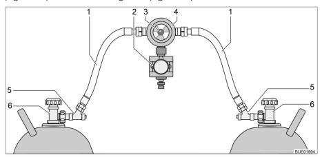
Fig. 103 Gas bottle switching facility with CPU
