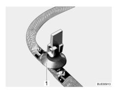
Fig. 147 Drain cock (with rocking lever)
