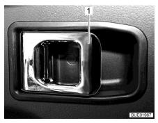
Fig. 50 Door lock (driver's door, inside)
