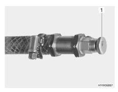
Fig. 200 Bleeding valve of hot-water heater
