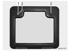
Fig. 46 Service flap push-button lock
