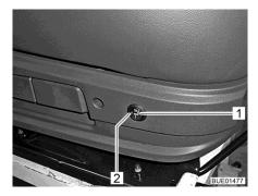
Fig. 28 Switch for seat heater
