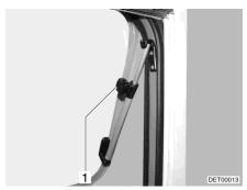
Fig. 71 Hinged window with rotary hinge
