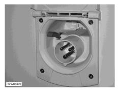
Fig. 124 230 V connection on the vehicle
