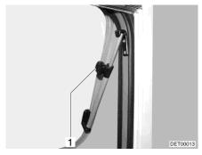
Fig. 95 Skylight with rotary hinges, open
