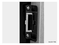
Fig. 167 Locking device in ventilation position
