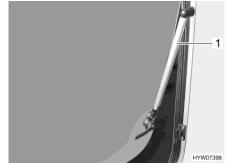
Fig. 72 Hinged window with automatic hinge
