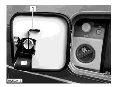
Fig. 184 Service flap with square spanner
