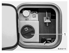
Fig. 197 Cleaning opening of the water tank (service unit)
