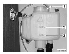
Fig. 199 Compensator reservoir without panel
