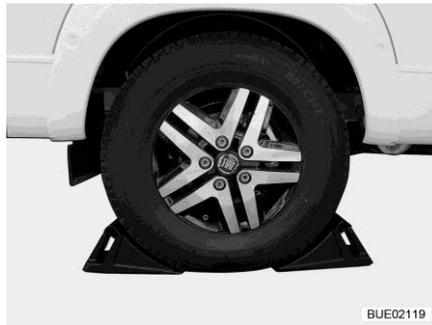
Fig. 172 Securing vehicle
