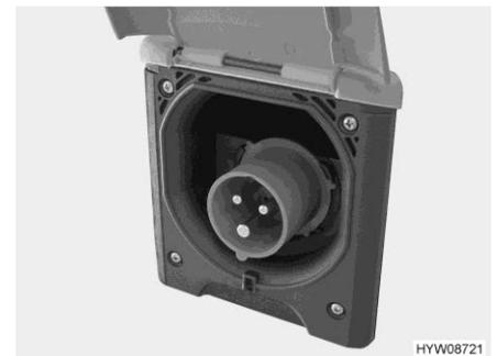
Fig. 101 230 V connection on the vehicle (CEE socket outlet)
