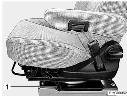
Fig. 18 Release lever for rotating
