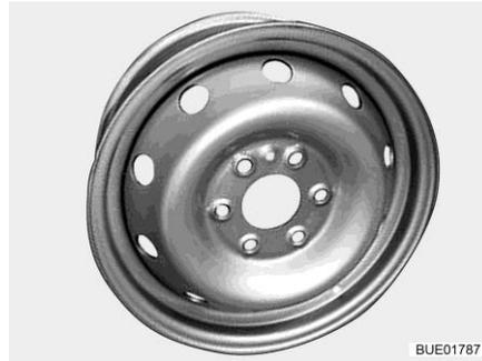
Fig. 170 Steel wheel rim (standard)
