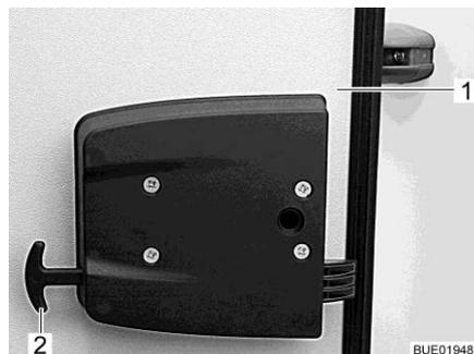
Fig. 38 Garage flap emergency release
