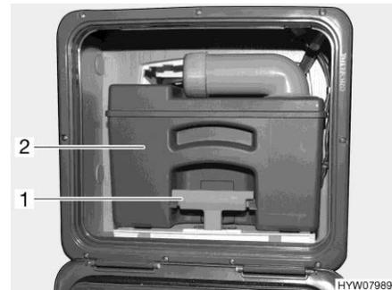
Fig. 153 Sewage tank (example)
