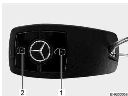
Fig. 32 Remote control for central locking system
