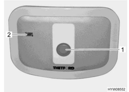
Fig. 157 Flush button/indicator lamp (Thetford toilet)
