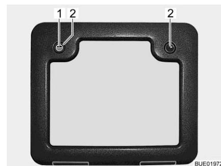
Fig. 40 Service flap push-button lock (alternative)
