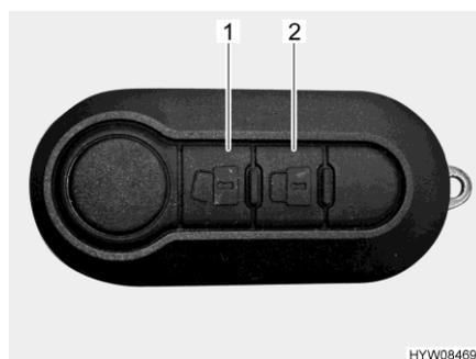
Fig. 49 Remote control for central locking system (2 buttons)
