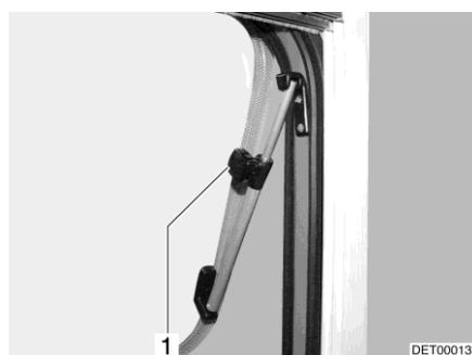
Fig. 123 Skylight with rotary hinges, open
