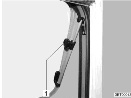
Fig. 99 Hinged window with rotary hinge
