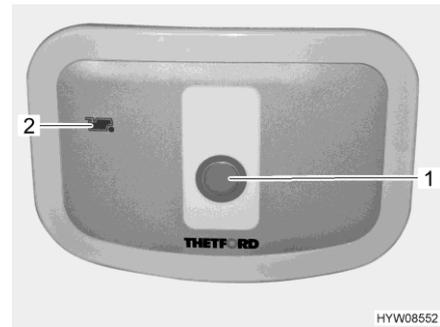
Fig. 298 Flush button/indicator lamp
