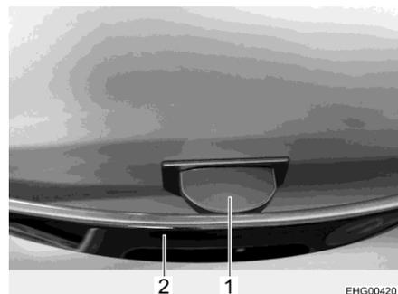
Fig. 67 Handle with release tab
