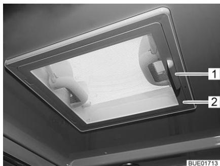
Fig. 112 Skylight with snap latch
