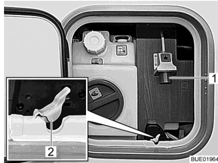
Fig. 207 230 V connection on the vehicle (with service unit)
