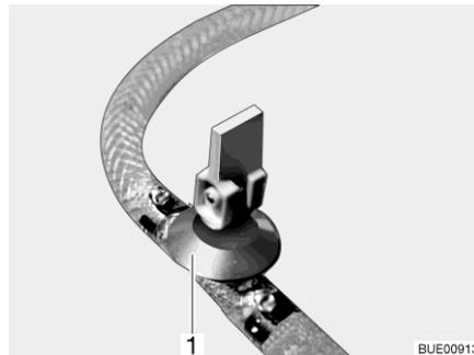
Fig. 273 Drain cock (with rocking lever)
