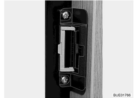
Fig. 270 Locking device in ventilation position
