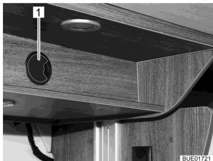
Fig. 150 Access to drive (behind access opening in panel)
