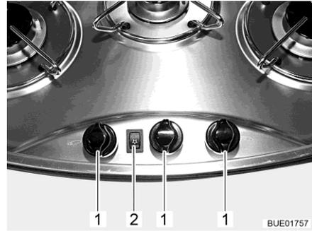
Fig. 253 Gas cooker, 3 burners
