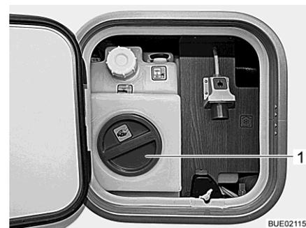
Fig. 307 Cleaning opening of the water tank (service unit)
