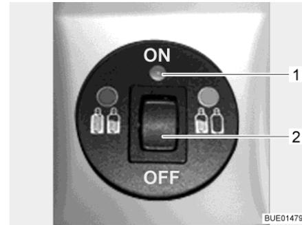
Fig. 197 Operating unit with remote display
