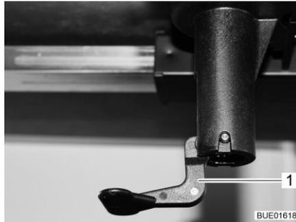
Fig. 128 Unlocking of the table top
