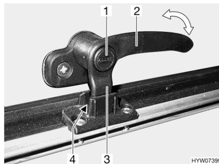
Fig. 101 Catch lever with safety knob in "continuous ventilation" position
