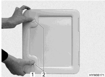
Fig. 289 Flap for sewage tank
