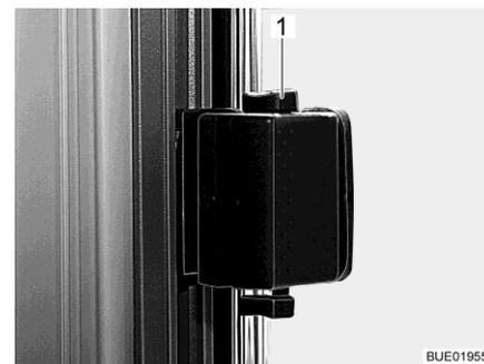
Fig. 104 Sliding window, unlocked
