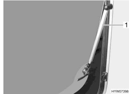
Fig. 100 Hinged window with automatic hinge
