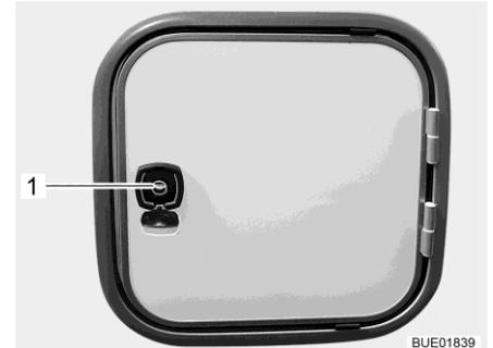
Fig. 302 Flap for the sewage tank (alternative)
