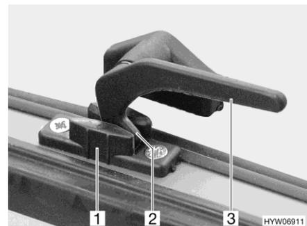
Fig. 102 Catch lever in "continuous ventilation" position
