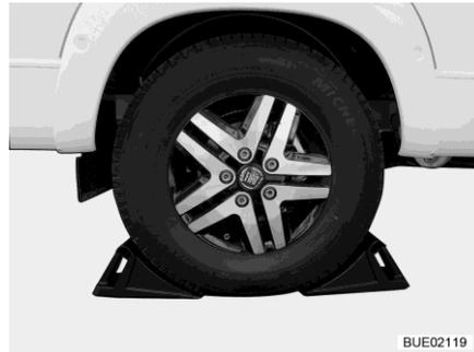
Fig. 325 Securing vehicle
