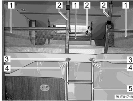
Fig. 148 Pull-down bed complete with applied safety net
