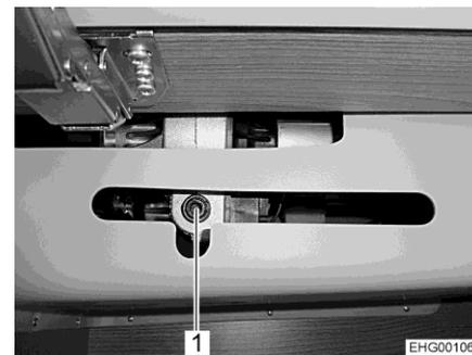
Fig. 151 Access to drive (behind panelling in the wall-mounted cupboard)
