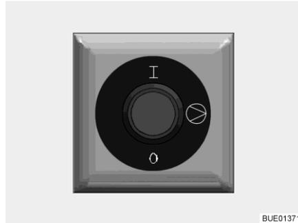
Fig. 240 Operating switch for auxiliary circulating pump
