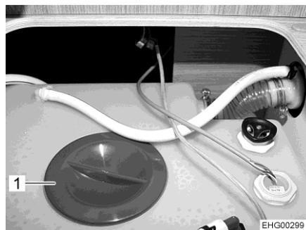
Fig. 306 Cleaning opening of the water tank
