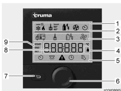
Fig. 230 Operating unit with displays
