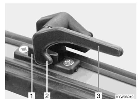
Fig. 98 Catch lever in "closed" position
