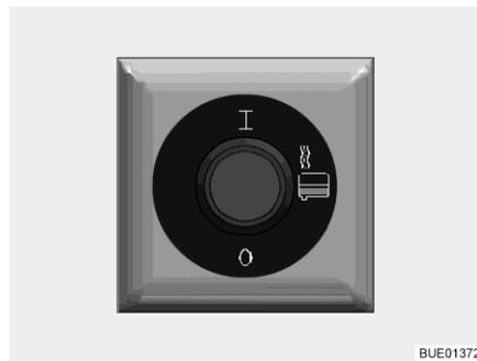
Fig. 287 Switch for waste water heating
