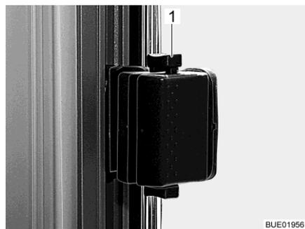
Fig. 103 Sliding window, locked
