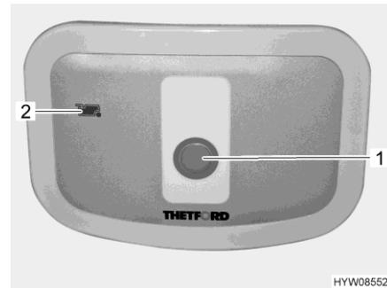
Fig. 298 Flush button/indicator lamp
