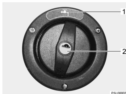
Fig. 271 Drinking water filler neck in the vehicle's side wall
