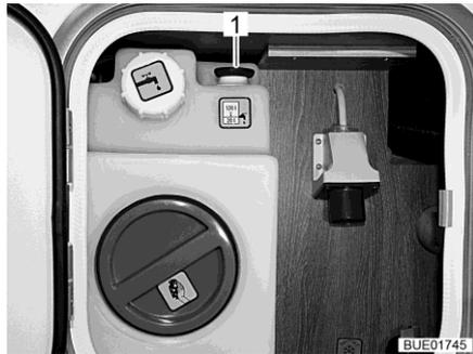
Fig. 279 Water tank (service unit)
