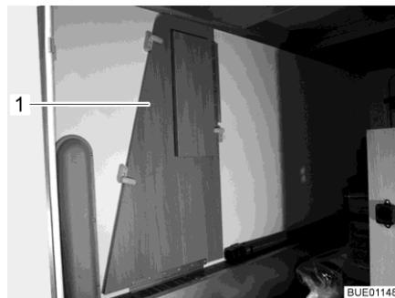
Fig. 12 Bed widening in the rear garage
