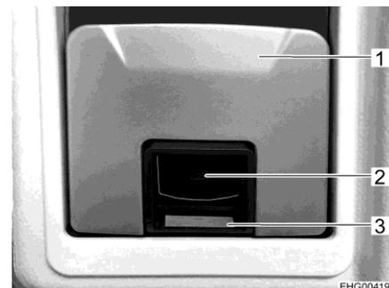
Fig. 54 Door lock, variant (conversion door, inside)
