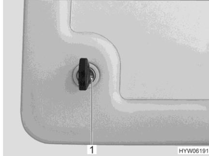
Fig. 59 Service flap push-button lock
