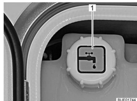
Fig. 272 Drinking water filler neck in service unit (alternative)
