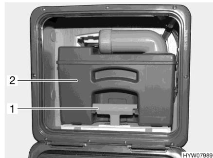
Fig. 292 Sewage tank (example)
