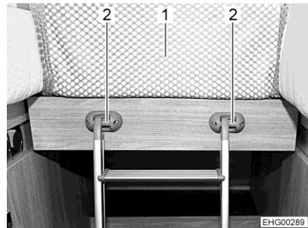
Fig. 187 Access ladder and safety net
