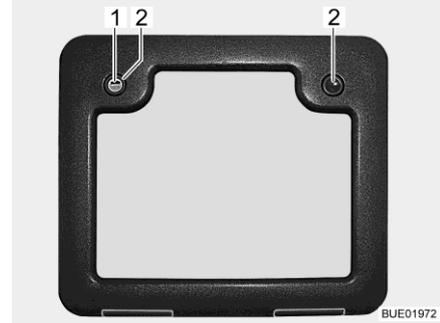
Fig. 60 Service flap push-button lock (alternative)
