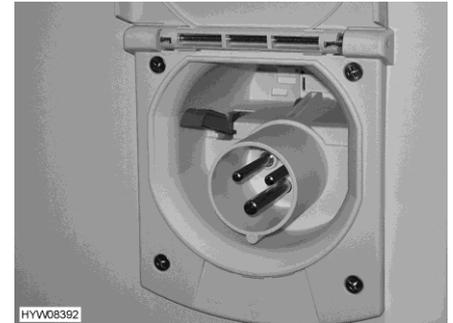
Fig. 208 230 V connection on the vehicle (without service unit)
