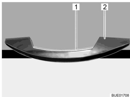
Fig. 66 Handle with unlocking bar (example)
