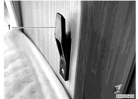
Fig. 189 Holder for fall out protection (bottom end)
