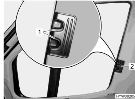
Fig. 41 Roman shade for the driver's / front passenger's window
