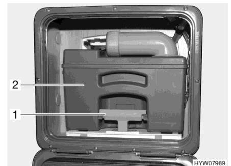
Fig. 304 Sewage tank (example)
