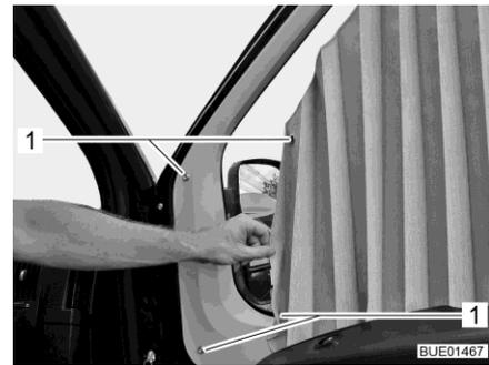
Fig. 108 Fixing of pleated shades
