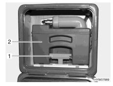
Fig. 176 Flap for sewage tank
