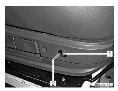
Fig. 19 Switch for seat heater
