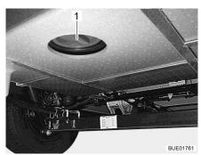
Fig. 185 Cleaning opening (waste water tank)
