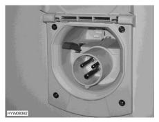
Fig. 123 230 V connection on the vehicle
