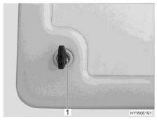
Fig. 42 Service flap push-button lock
