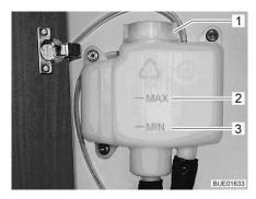
Fig. 186 Compensator reservoir without panel
