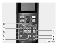
Fig. 151 Remote control with setting buttons (air conditioning unit)
