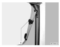
Fig. 70 Hinged window with rotary hinge
