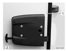
Fig. 40 Garage flap emergency release
