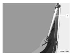
Fig. 71 Hinged window with automatic hinge
