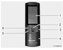
Fig. 149 Remote control (air conditioning unit)
