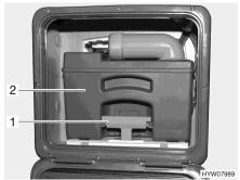
Fig. 182 Flap for the sewage tank
