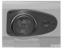
Fig. 193 LED light with switch
