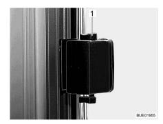
Fig. 100 Sliding window, unlocked
