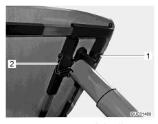
Fig. 128 Adjustment of lift-off table
