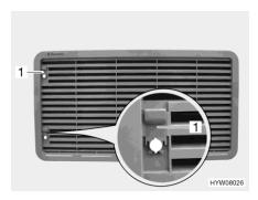
Fig. 250 Refrigerator ventilation grill (with sliding trap)
