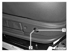
Fig. 36 Switch for seat heater
