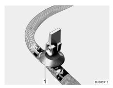
Fig. 269 Drain cock (with rocking lever)
