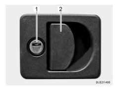
Fig. 57 Flap lock with recessed handle
