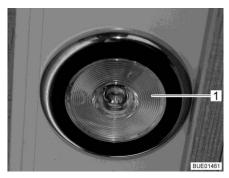
Fig. 80 Recessed light, light switch in the lamp.
