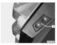
Fig. 258 Release button (refrigerator door, Dometic 8 series)
