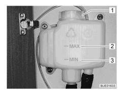
Fig. 305 Compensator reservoir without panel
