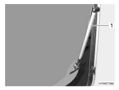
Fig. 96 Hinged window with automatic hinge
