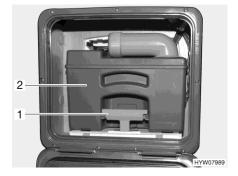
Fig. 300 Sewage tank (example)
