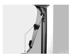
Fig. 119 Skylight with rotary hinges, open
