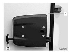
Fig. 58 Garage flap emergency release
