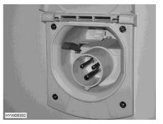
Fig. 194 230 V connection on the vehicle (without service unit)
