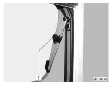
Fig. 95 Hinged window with rotary hinge
