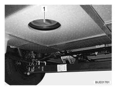
Fig. 304 Cleaning opening (waste water tank)
