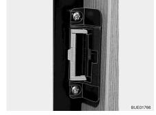
Fig. 266 Locking device in ventilation position
