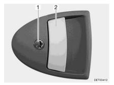
Fig. 53 Door lock, variant (conversion door, outside)
