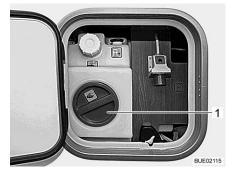
Fig. 303 Cleaning opening of the water tank (service unit)
