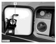
Fig. 282 Service flap with square spanner
