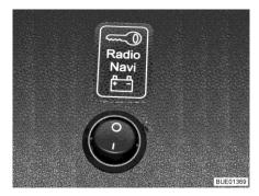
Fig. 185 Selector switch for power supply
