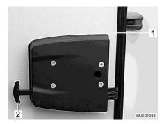
Fig. 73 Garage flap emergency release
