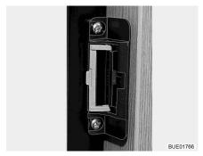
Fig. 245 Locking device in ventilation position
