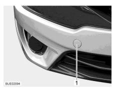
Fig. 57 Cover for the towing eye holder (example)
