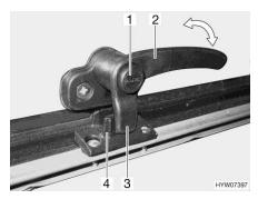
Fig. 109 Catch lever with safety knob in "closed" position
