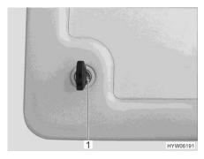
Fig. 78 Service flap push-button lock
