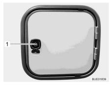
Fig. 277 Flap for sewage tank (alternative)
