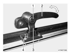
Fig. 113 Catch lever with safety knob in "continuous ventilation" position
