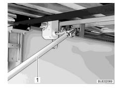
Fig. 151 Crank in the rear garage
