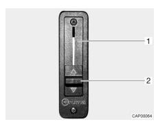
Fig. 37 Sliding regulator for branch block
