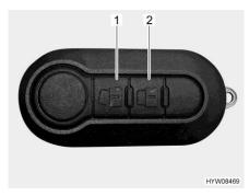
Fig. 63 Remote control for central locking system (2 buttons)
