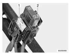
Fig. 191 Fuses on the starter battery
