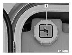
Fig. 250 Drinking water filler neck in service unit (alternative)
