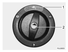
Fig. 81 Cap for the drinking water filler neck
