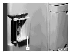
Fig. 247 Locking device in normal position
