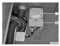
Fig. 223 Transformer for electrical floor warming unit
