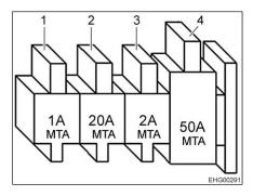
Fig. 193 Fuses (living area battery with charging booster)
