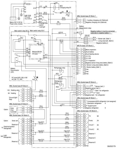
Fig. 201 Circuit diagram, interior (EBL 119)
