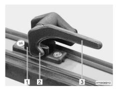
Fig. 110 Catch lever in "closed" position
