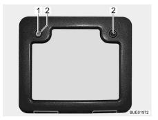
Fig. 79 Service flap push-button lock (alternative)
