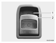
Fig. 69 Door lock (conversion door, inside)
