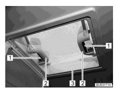
Fig. 123 Skylight with snap latch
