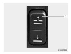
Fig. 45 Switch (electric operation of the Roman shade)
