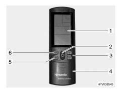
Fig. 225 Remote control (air conditioning unit)
