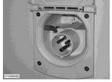
Fig. 189 230 V connection on the vehicle (without service unit)
