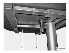
Fig. 132 Lever for moving the table top
