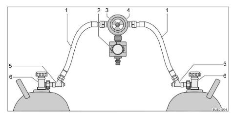
Fig. 16 Gas regulator with CPU and hose break guard
