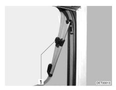
Fig. 111 Hinged window with rotary hinge
