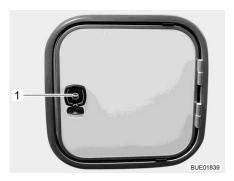
Fig. 268 Flap for sewage tank (alternative)
