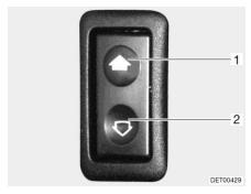
Fig. 38 Switch for electrical window winder
