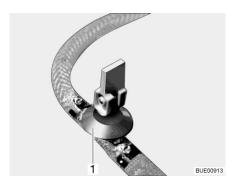
Fig. 251 Drain cock (with rocking lever)
