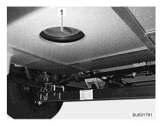
Fig. 282 Cleaning opening (waste water tank)
