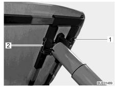
Fig. 129 Adjustment of lift-off table
