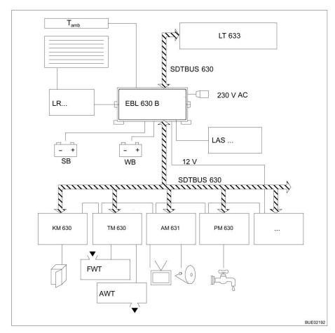
Fig. 202 Block diagram for energy supply of transformer/rectifier EBL 630
