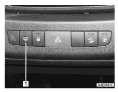
Fig. 41 External mirror heater switch
