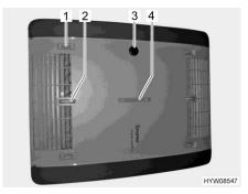
Fig. 226 Function display and air distribution (air conditioning unit)
