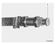
Fig. 284 Bleeding valve of hot-water heater
