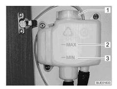
Fig. 283 Compensator reservoir without panel
