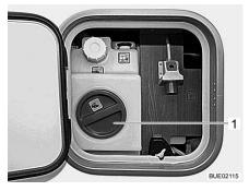
Fig. 281 Cleaning opening of the water tank (service unit)
