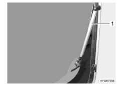
Fig. 112 Hinged window with automatic hinge
