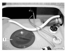
Fig. 280 Cleaning opening of the water tank
