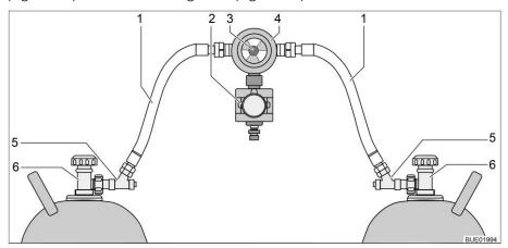
Fig. 173 Gas bottle switching facility with CPU
