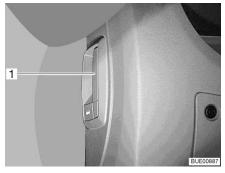
Fig. 48 Release lever for the bonnet (inside the vehicle)
