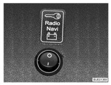
Fig. 180 Selector switch for power supply
