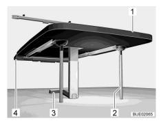
Fig. 135 Suspension table as bed foundation
