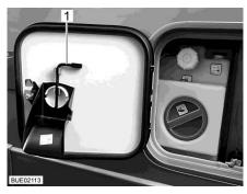
Fig. 264 Service flap with square spanner
