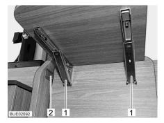
Fig. 28 Catches on the folding table
