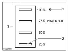
Fig. 185 Status indicator, solar charge regulator
