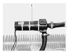
Fig. 218 Auxiliary circulating pump
