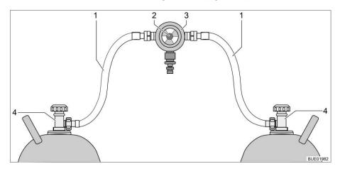
Fig. 172 Gas bottle switching facility
