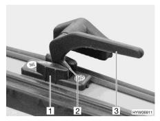
Fig. 114 Catch lever in "continuous ventilation" position
