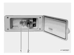
Fig. 171 External gas connection (gas isolator tap closed)
