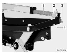
Fig. 142 Drive for the pull-down bed
