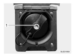
Fig. 55 Cap for the fuel filler neck
