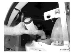
Fig. 53 Filler neck in filling position
