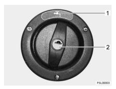
Fig. 249 Drinking water filler neck in the vehicle's side wall
