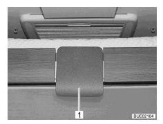
Fig. 138 Release plate on the pull-down bed (Ixeo I)
