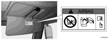
Fig. 18 Warning notice on child restraint system (front passenger's seat sun visor)
