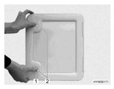
Fig. 267 Flap for sewage tank
