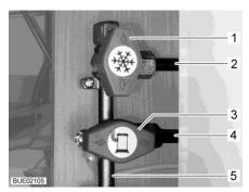
Fig. 170 Gas isolator taps position (example)
