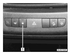
Fig. 65 Central locking system switch
