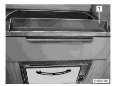
Fig. 232 Heat protection sheet (loose)
