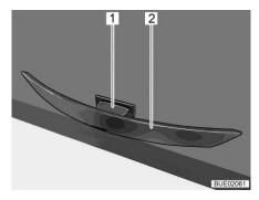
Fig. 84 Handle with release button
