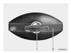
Fig. 74 Flap lock (elliptical-shaped, closed)
