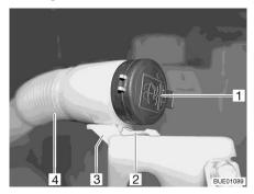
Fig. 52 Washer fluid container filler neck
