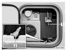
Fig. 188 230 V connection on the vehicle (with service unit)
