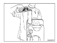
Fig. 270 Turning drainage neck
