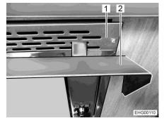
Fig. 233 Heat protection sheet (hooked in)
