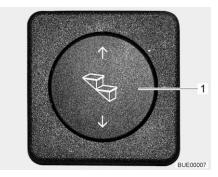
Fig. 10 Rocker button for entrance step
