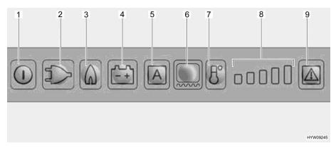
Fig. 243 LED operating panel (Dometic refrigerator)
