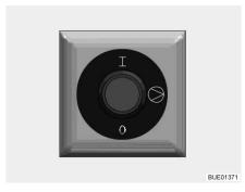
Fig. 219 Operating switch for auxiliary circulating pump
