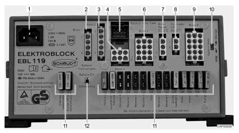
Fig. 181 Transformer/rectifier (EBL 119)
