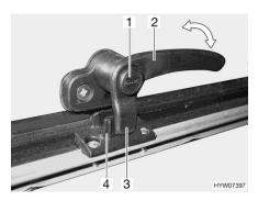
Fig. 68 Catch lever with safety knob in "closed" position
