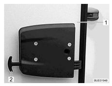
Fig. 38 Garage flap emergency release
