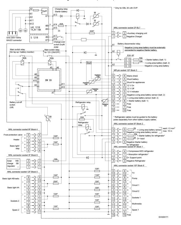
Fig. 111 Circuit diagram, interior (EBL 30)
