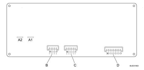
Fig. 112 Connection diagram, panel (LT 96)
