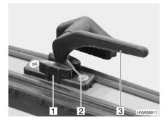
Fig. 72 Catch lever in "continuous ventilation" position
