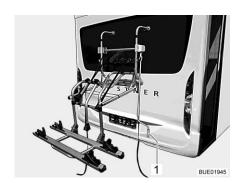
Fig. 2 Bike rack, folded upwards
