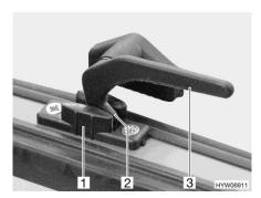
Fig. 56 Catch lever ("continuous ventilation" position)
