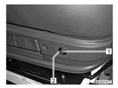
Fig. 20 Switch for seat heater
