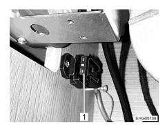
Fig. 106 Pull-down bed fuse (Ixeo T)
