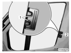
Fig. 25 Roman shade for the driver's / front passenger's window
