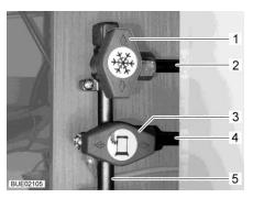
Fig. 88 Gas isolator taps position (example)
