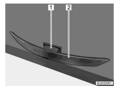
Fig. 43 Handle with release button
