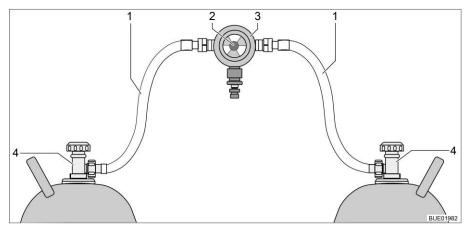
Fig. 90 Gas bottle switching facility
