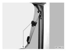
Fig. 70 Skylight with rotary hinges, open
