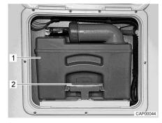
Fig. 160 Flap for the sewage tank
