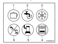
Fig. 87 Possible symbols for the gas isolator taps
