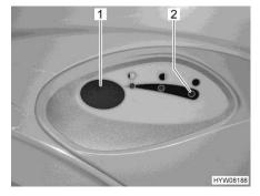
Fig. 159 Flush button/indicator lamp (Thetford toilet)
