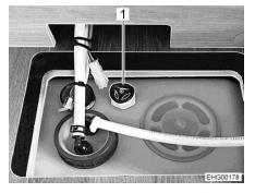
Fig. 142 Water tank with rotary handle
