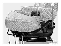
Fig. 18 Release lever for rotating
