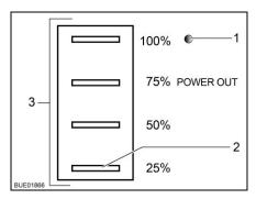
Fig. 99 Status indicator, solar charge regulator
