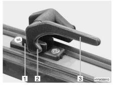
Fig. 69 Catch lever in "closed" posi-
