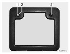
Fig. 40 Service flap push-button lock (alternative)
