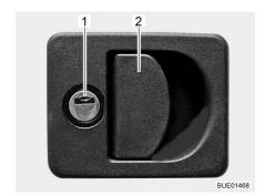
Fig. 37 Flap lock with recessed handle
