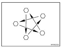
Fig. 169 Tighten the wheel nuts or wheel bolts cross-wise
