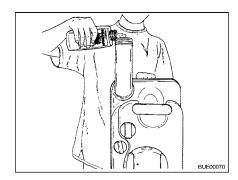
Fig. 155 Filling with sanitary liquid
