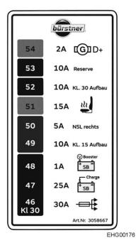
Fig. 103 Fuses in the seat console of the driver's seat
