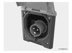
Fig. 101 230 V connection on the vehicle (CEE socket outlet)
