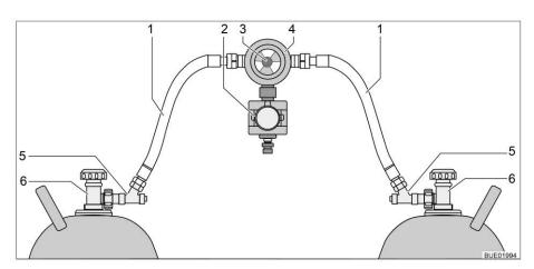
Fig. 13 Gas regulator with CPU and hose break guard
