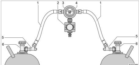
Fig. 91 Gas bottle switching facility with CPU
