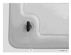
Fig. 39 Service flap push-button lock
