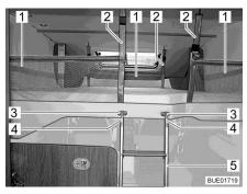
Fig. 78 Pull-down bed complete with applied safety net
