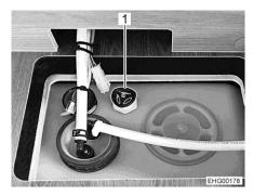
Fig. 143 Water tank with rotary handle
