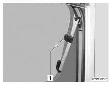
Fig. 54 Hinged window with rotary hinges (open)
