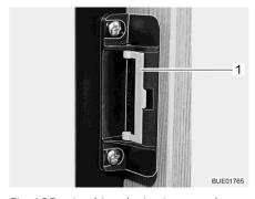
Fig. 135 Locking device in normal position
