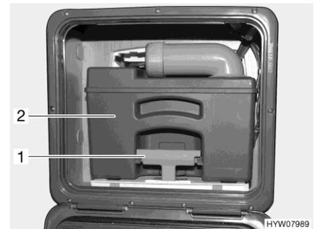
Fig. 290 Sewage tank (example)
