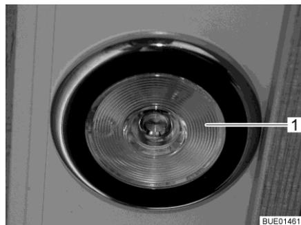
Fig. 78 Recessed light, light switch in the lamp.
