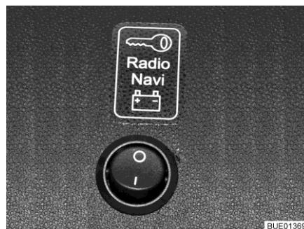
Fig. 181 Selector switch for operating behaviour
