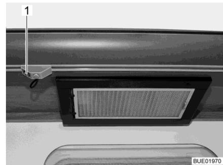
Fig. 242 Recirculating extractor hood
