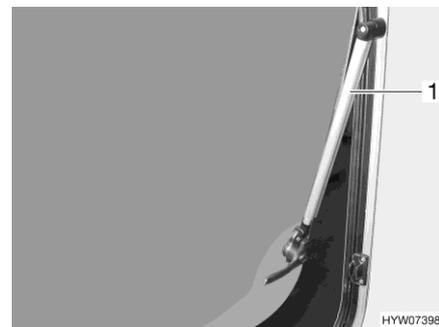
Fig. 92 Hinged window with automatic hinge
