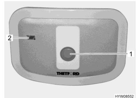
Fig. 284 Flush button/indicator lamp Thetford toilet (alternative)
