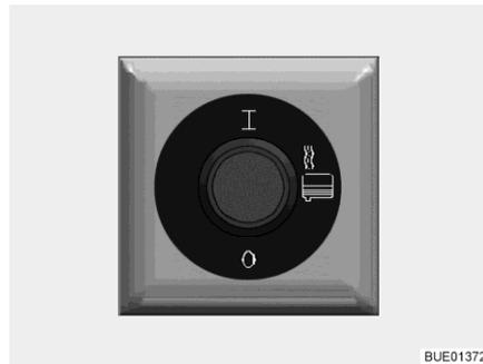
Fig. 273 Switch for waste water heating
