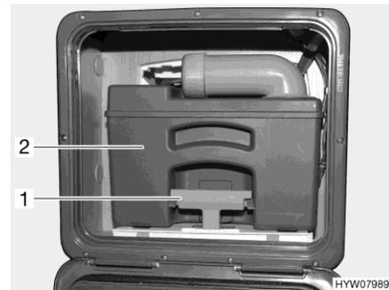
Fig. 278 Sewage tank (example)
