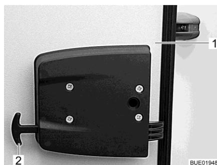
Fig. 55 Garage flap emergency release
