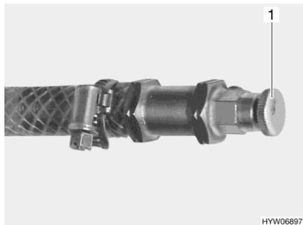
Fig. 293 Bleeding valve of hot-water heater
