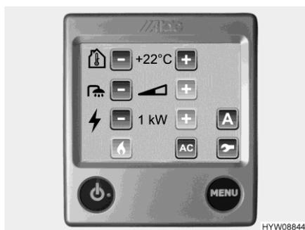
Fig. 217 Adjustment menu (operating unit)
