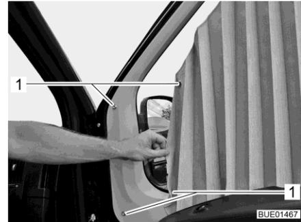
Fig. 100 Fixing of pleated shades
