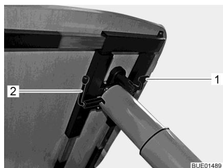
Fig. 124 Adjustment of lift-off table
