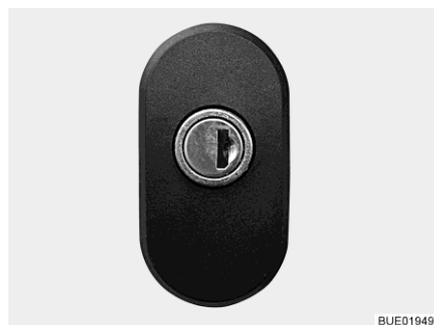
Fig. 58 Flap lock, locked
