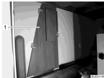
Fig. 14 Bed widening in the rear garage
