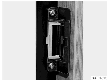
Fig. 259 Locking device in ventilation position
