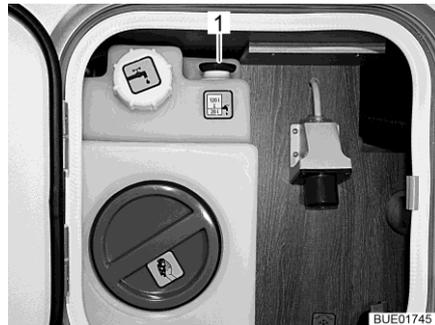
Fig. 266 Water tank (central supply unit)
