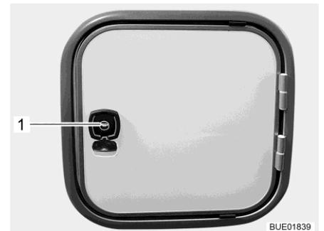
Fig. 276 Flap for sewage tank (alternative)
