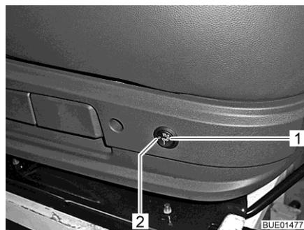
Fig. 32 Switch for seat heater
