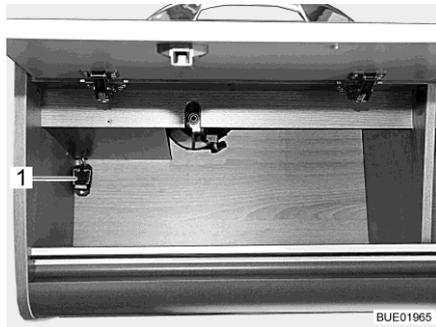
Fig. 197 Front pull-down bed fuse
