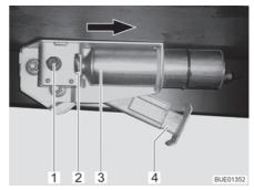
Fig. 51 Electrical steady leg on vehicle
