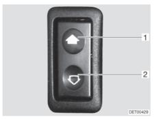
Fig. 32 Switch for electrical window winders
