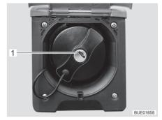
Fig. 44 Fuel filler neck external flap
