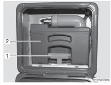
Fig. 201 Sewage tank (example)
