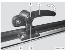
Fig. 97 Catch lever with safety knob in "continuous ventilation" posi-
