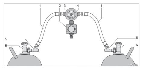
Fig. 132 Gas bottle switching facility with CPU
