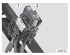
Fig. 144 Fuses on the starter battery
