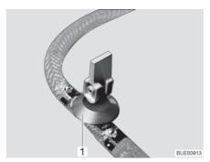
Fig. 190 Drain cock (with rocking lever)
