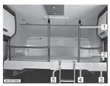
Fig. 120 Pull-down bed complete with applied safety net
