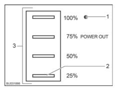
Fig. 140 Status indicator, solar charge regulator
