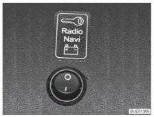
Fig. 137 Selector switch for operating behaviour
