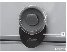
Fig. 165 Flue shield
