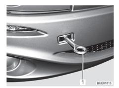
Fig. 47 Towing eye, mounted
