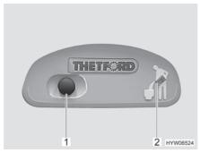
Fig. 206 Flush button/indicator lamp Thetford toilet
