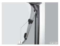
Fig. 95 Hinged window with rotary hinge
