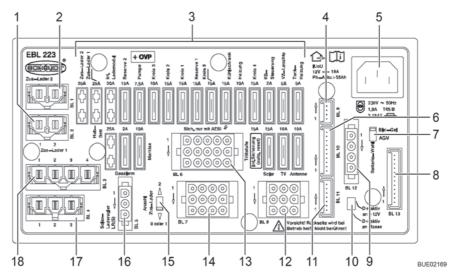
Fig. 138 Transformer/rectifier (EBL 223)
