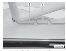
Fig. 109 Heki skylight in ventilation position
