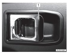
Fig. 62 Door lock of driver's door, inside
