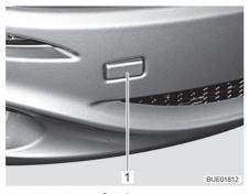
Fig. 46 Cover for the towing eye holder (example)
