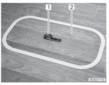
Fig. 76 Floor compartment cover (handle swung out)
