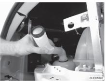
Fig. 43 Filler neck in filling position
