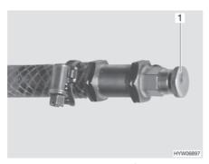
Fig. 213 Bleeding valve of hot-water heater
