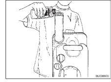
Fig. 202 Turning drainage neck
