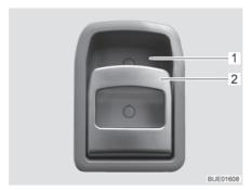
Fig. 63 Door lock of conversion door, inside
