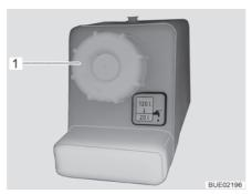
Fig. 189 Cap for the drinking water filler neck
