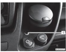
Fig. 50 Push-button to activate remote control
