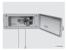
Fig. 130 External gas connection (gas isolator tap closed)
