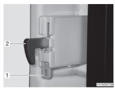
Fig. 186 Fixture (lock hook)
