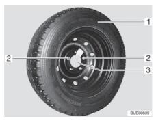
Fig. 229 Spare wheel support in the rear garage
