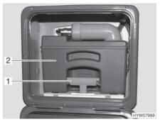
Fig. 209 Sewage tank (example)
