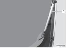
Fig. 96 Hinged window with automatic hinge
