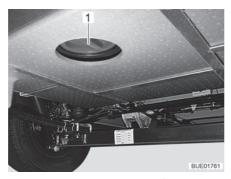
Fig. 211 Cleaning opening of the waste water tank
