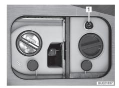
Fig. 193 Water tank with rotary handle
