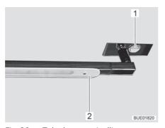
Fig. 82 Tube lamp, swivelling
