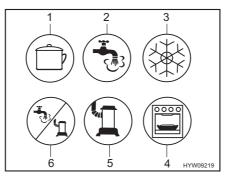
Fig. 128 Possible symbols for the gas isolator taps
