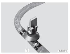
Fig. 194 Drain cock (with rocking lever)
