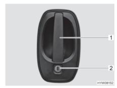
Fig. 61 Door lock (driver's door/conversion door, outside)
