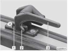
Fig. 94 Catch lever in "closed" position
