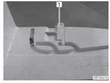
Fig. 110 Ventilation position locking mechanism
