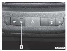
Fig. 60 Central locking system switch
