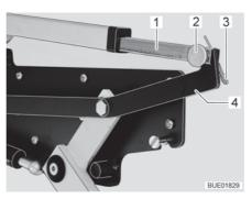
Fig. 123 Drive for the pull-down bed
