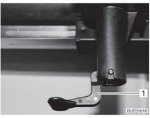
Fig. 116 Unlocking of the table top
