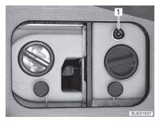
Fig. 192 Water tank with rotary handle
