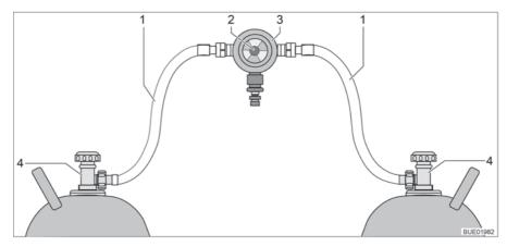
Fig. 131 Gas bottle switching facility
