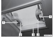
Fig. 111 Skylight with snap latch
