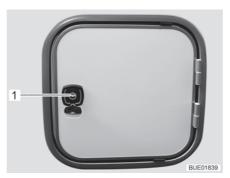
Fig. 208 Flap for sewage tank
