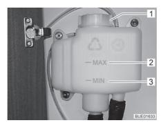
Fig. 212 Compensator reservoir without panel
