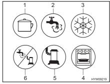
Fig. 183 Symbols for the gas isolator taps
