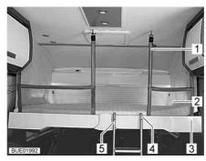
Fig. 142 Pull-down bed complete with applied safety net
