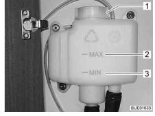
Fig. 261 Compensator reservoir without panel
