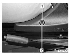
Fig. 30 Seat heater switch
