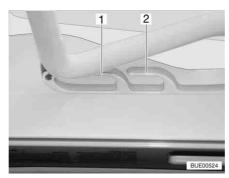
Fig. 127 Heki skylight in ventilation position
