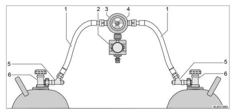
Fig. 155 Gas bottle switching facility with CPU
