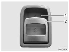
Fig. 68 Door lock of conversion door, inside
