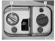
Fig. 258 Water tank with handle (Viseo)
