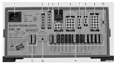
Fig. 162 Transformer/rectifier (EBL 99)
