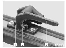
Fig. 108 Catch lever in "closed" position
