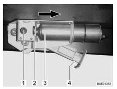
Fig. 56 Electrical steady leg on vehicle
