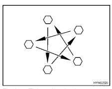
Fig. 277 Tighten the wheel nuts or wheel bolts cross-wise
