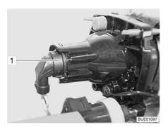
Fig. 265 Low beam/main beam/parking light
