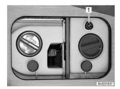
Fig. 233 Water tank with handle (Viseo)
