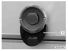
Fig. 14 Flue shield
