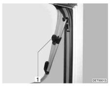
Fig. 109 Hinged window with rotary hinge
