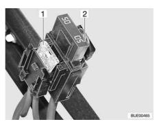
Fig. 170 Fuses on the starter battery
