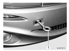
Fig. 50 Cover for the towing eye holder
