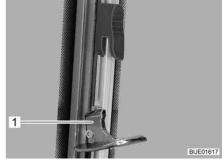
Fig. 116 Sliding window with swivel lock (locked)
