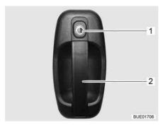
Fig. 67 Door lock of conversion door, outside
