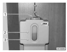
Fig. 260 Compensator reservoir with panel
