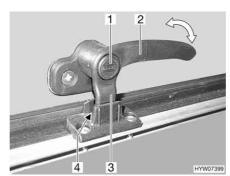
Fig. 111 Catch lever with safety knob in "continuous ventilation" posi-
