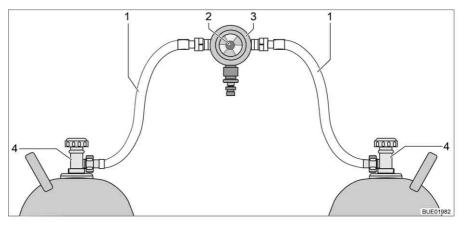
Fig. 154 Gas bottle switching facility
