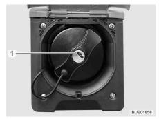
Fig. 49 Cap for the fuel filler neck
