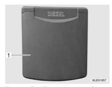
Fig. 48 Fuel filler neck external flap
