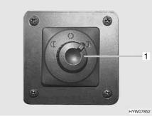
Fig. 37 External mirror adjustment switch
