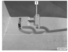
Fig. 128 Ventilation position locking mechanism
