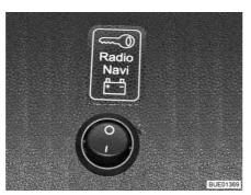
Fig. 161 Selector switch for operating behaviour
