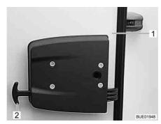
Fig. 72 Garage flap emergency release
