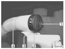
Fig. 45 Washer fluid container filler neck
