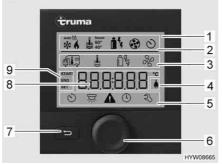
Fig. 186 Operating unit with displays
