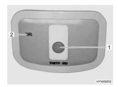
Fig. 253 Flush button/indicator lamp Thetford toilet (alternative)
