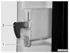
Fig. 222 Lock hook fixture
