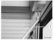
Fig. 124 Hand crank for emergency operation
