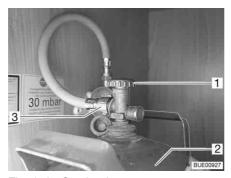
Fig. 158 Gas bottle compartment
