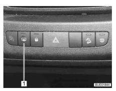
Fig. 38 Switch for the external mirror heater (Elegance)
