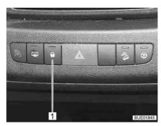
Fig. 63 Switch for the central locking system (Elegance)
