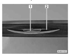
Fig. 82 Handle with unlocking bar
