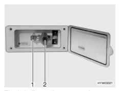
Fig. 153 External gas connection, gas isolator tap closed
