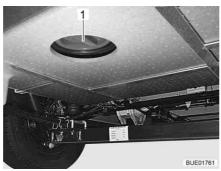
Fig. 257 Cleaning opening of the waste water tank
