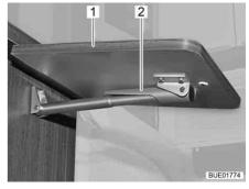
Fig. 138 Folding worktop, unlocked
