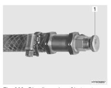
Fig. 262 Bleeding valve of hot-water heater
