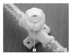
Fig. 227 Drain cock (with rocking lever)
