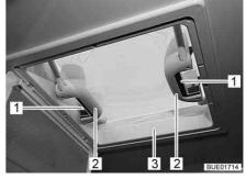
Fig. 129 Skylight with snap latch
