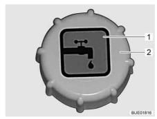
Fig. 226 Cap for the drinking water filler neck
