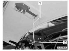
Fig. 42 Release lever for the bonnet (inside the vehicle)
