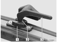
Fig. 112 Catch lever in "continuous ventilation" position
