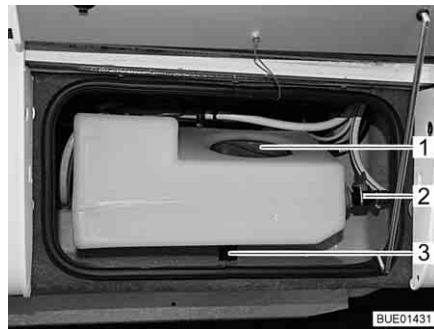
Fig. 203 Auxiliary water tank
