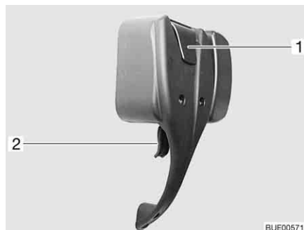
Fig. 42 Door lock of conversion door, inside, locked
