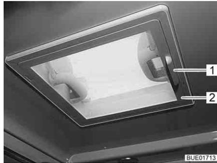
Fig. 77 Skylight with snap latch
