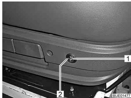
Fig. 25 Switch for seat heater
