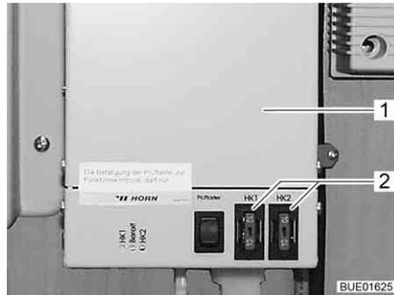
Fig. 150 Heater regulation for waste water pipes
