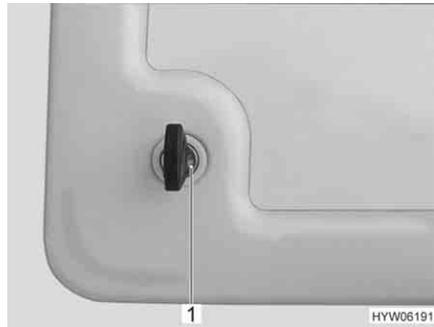
Fig. 46 Push-button lock service flap
