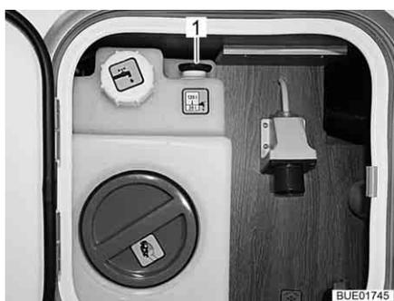
Fig. 209 Water tank (central supply unit)
