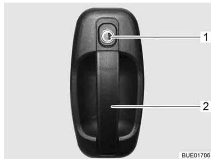
Fig. 40 Door lock of conversion door, outside
