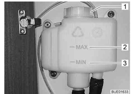
Fig. 233 Compensator reservoir without panel
