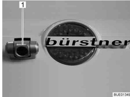
Fig. 20 Reversing camera with infrared illumination
