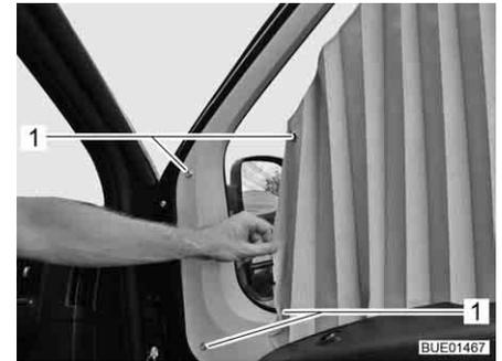
Fig. 74 Fixing of pleated shades
