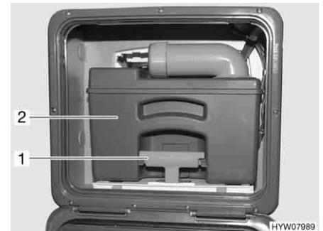
Fig. 219 Sewage tank (example)
