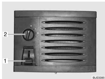
Fig. 177 Operating controls for auxiliary heat exchanger
