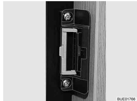
Fig. 205 Locking device in ventilation position
