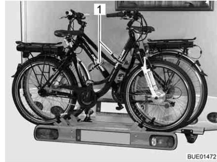
Fig. 6 Positioning of e-bikes
