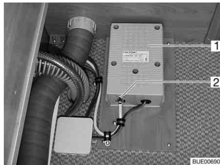
Fig. 178 Transformer for electrical floor warming unit
