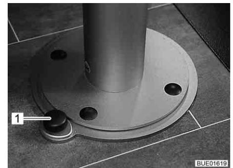
Fig. 94 Unlocking the table leg
