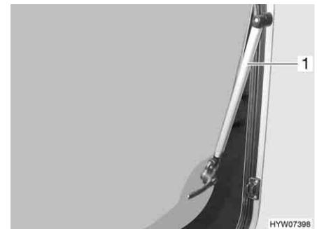
Fig. 68 Hinged window with automatic hinge
