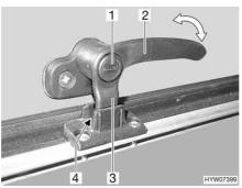
Fig. 69 Catch lever with safety knob in "continuous ventilation" position
