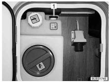
Fig. 210 Water tank (central supply unit)
