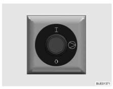
Fig. 175 Operating switch for auxiliary circulating pump
