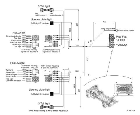
Fig. 161 Circuit diagram, exterior
