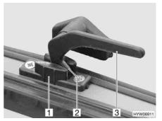
Fig. 70 Catch lever in "continuous ventilation" position
