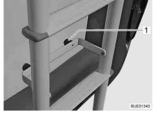
Fig. 1 Foldable ladder, ladder folded upwards
