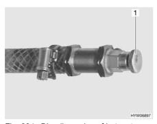
Fig. 234 Bleeding valve of hot-water heater
