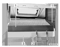
Fig. 106 Pull-down bed with safety plates
