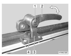
Fig. 87 Catch lever with safety knob in "closed" position
