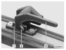
Fig. 66 Catch lever in "closed" position
