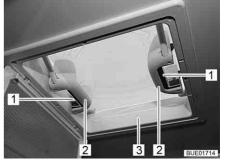
Fig. 77 Skylight with snap latch
