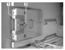
Fig. 199 Locking device in normal position
