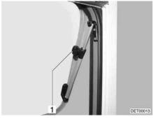
Fig. 89 Skylight with rotary hinges, open
