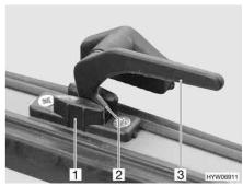
Fig. 91 Catch lever in "continuous ventilation" position
