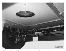
Fig. 230 Cleaning opening on the waste water tank
