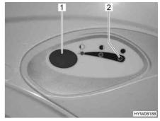
Fig. 227 Flush button/indicator lamp Thetford toilet
