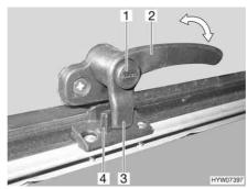
Fig. 65 Catch lever with safety knob in "closed" position
