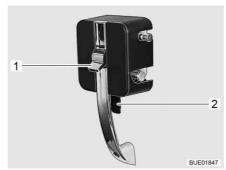
Fig. 39 Door lock of conversion door, inside
