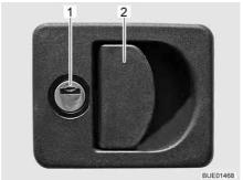
Fig. 44 Flap lock with recessed handle
