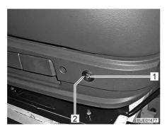
Fig. 25 Switch for seat heater
