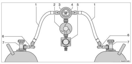
Fig. 133 Crash protection unit switching facility
