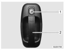
Fig. 40 Door lock of conversion door, outside
