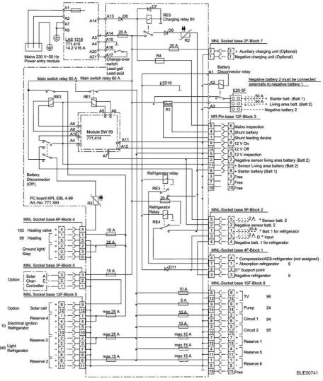
Fig. 158 Circuit diagram, interior (EBL 99)
