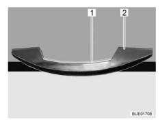
Fig. 50 Handle with unlocking bar (example)
