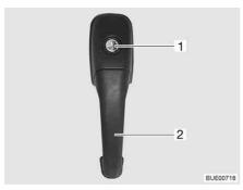
Fig. 38 Door lock of conversion door, outside
