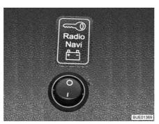
Fig. 138 Selector switch for operating behaviour
