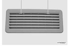
Fig. 191 Refrigerator ventilation grill (Thetford large)
