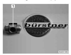
Fig. 20 Reversing camera with infrared illumination
