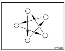
Fig. 242 Tighten the wheel nuts or wheel bolts cross-wise
