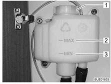
Fig. 233 Compensator reservoir without panel
