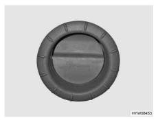
Fig. 163 Air outlet nozzle of the hot air distribution
