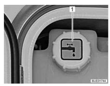
Fig. 206 Cap for drinking water filler neck (central supply unit)
