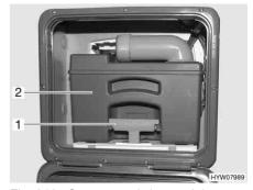
Fig. 219 Sewage tank (example)
