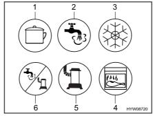
Fig. 162 Symbols for the gas isolator taps
