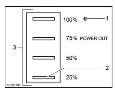
Fig. 142 Status indicator, solar charge regulator
