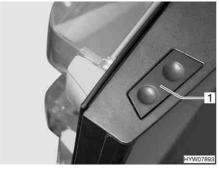
Fig. 197 Release button of the refrigerator door (Dometic 8 series)
