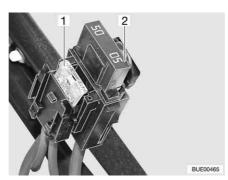
Fig. 146 Fuses on the starter battery
