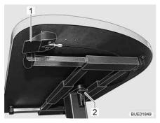
Fig. 100 Adjustment of lift-off table
