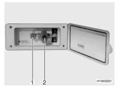
Fig. 132 External gas connection, gas isolator tap closed
