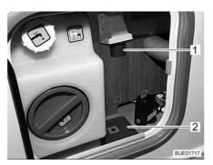
Fig. 144 230 V connection on vehicle
