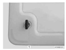
Fig. 46 Push-button lock service flap
