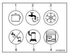
Fig. 130 Possible symbols for the gas isolator taps
