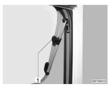
Fig. 67 Hinged window with rotary hinge
