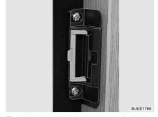
Fig. 205 Locking device in ventilation position
