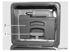
Fig. 228 Flap for the sewage tank
