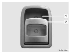
Fig. 41 Door lock of conversion door, inside
