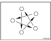
Fig. 268 Tighten the wheel nuts or wheel bolts cross-wise
