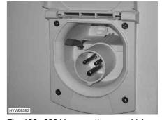
Fig. 162 230 V connection on vehicle
