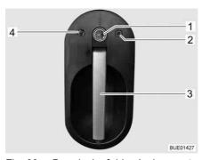
Fig. 60 Door lock of driver's door, outside
