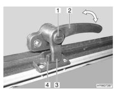
Fig. 101 Catch lever with safety knob in "closed" position
