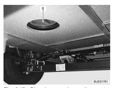
Fig. 247 Cleaning opening on the waste water tank
