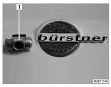
Fig. 19 Reversing camera with infrared illumination
