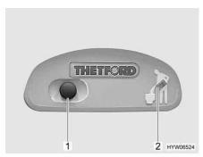
Fig. 242 Flush button/indicator lamp Thetford toilet
