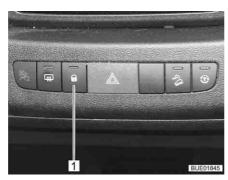
Fig. 59 Switch for the central locking system (Elegance)
