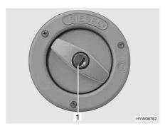
Fig. 45 Cap for the fuel filler neck
