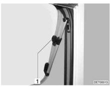
Fig. 103 Hinged window with rotary hinge
