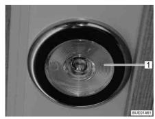
Fig. 90 Recessed light, light switch in the lamp
