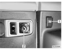
Fig. 34 External mirror adjustment and heater switch (Viseo)
