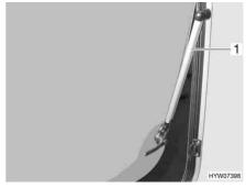
Fig. 104 Hinged window with automatic hinge
