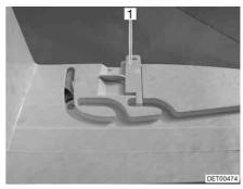
Fig. 119 Ventilation position locking mechanism
