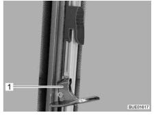
Fig. 109 Sliding window with swivel lock (unlocked)
