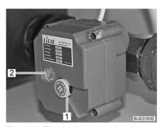
Fig. 230 Electrically operated drainage valve
