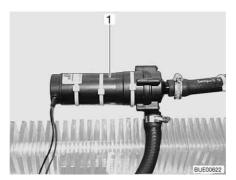
Fig. 189 Auxiliary circulating pump
