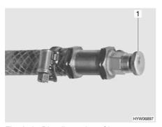
Fig. 253 Bleeding valve of hot-water heater
