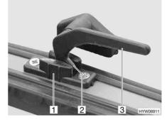
Fig. 106 Catch lever in "continuous ventilation" position
