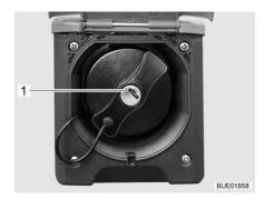
Fig. 46 Fuel filler neck external flap
