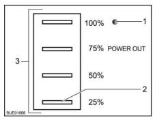
Fig. 160 Status indicator, solar charge regulator
