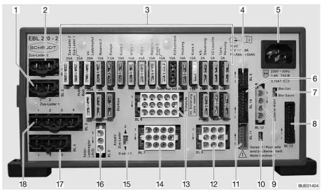
Fig. 157 Transformer/rectifier (EBL 220)
