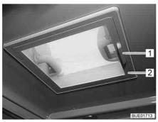
Fig. 120 Skylight with snap latch
