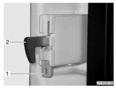
Fig. 212 Lock hook fixture
