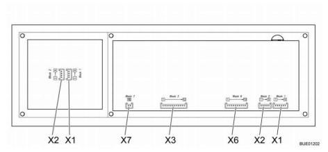
Fig. 175 Block diagram, panel (LT 511)
