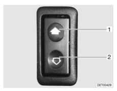
Fig. 32 Switch for electrical window winders
