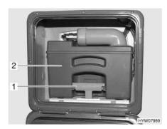
Fig. 246 Sewage tank (example)
