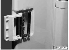
Fig. 217 Locking device in ventilation position
