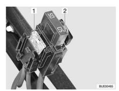
Fig. 164 Fuses on the starter battery
