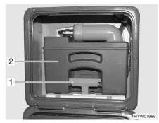
Fig. 237 Sewage tank (example)
