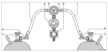
Fig. 150 Crash protection unit switching facility
