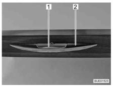
Fig. 76 Handle with unlocking bar
