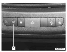
Fig. 36 Switch for the external mirror heater (Elegance)
