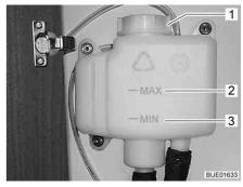
Fig. 252 Compensator reservoir without panel
