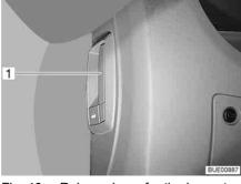
Release lever for the bonnet Fig. 40 (inside the vehicle)
