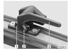
Fig. 102 Catch lever in "closed" position
