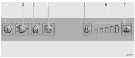
Fig. 209 Operating controls for the refrigerator
