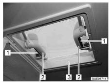
Fig. 121 Handles with snap latches
