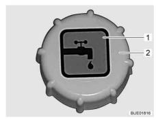
Fig. 219 Cap for the drinking water filler neck
