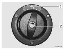
Fig. 71 Cap for the drinking water filler neck (Viseo)
