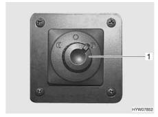
Fig. 35 External mirror adjustment switch
