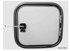
Fig. 236 Flap for sewage tank (alternative)
