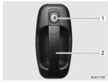
Fig. 63 Door lock of conversion door, outside
