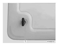
Fig. 69 Push-button lock service flap
