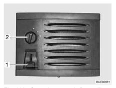
Fig. 192 Operating controls for auxiliary heat exchanger
