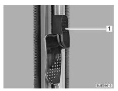
Fig. 108 Sliding window with swivel lock (locked)
