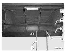
Fig. 136 Pull-down bed complete with applied safety net
