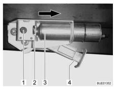
Fig. 54 Electrical steady leg on vehicle
