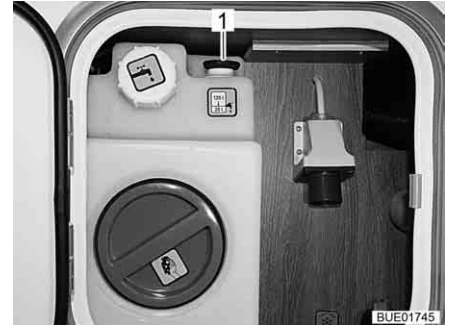
Fig. 234 Water tank (central supply unit)
