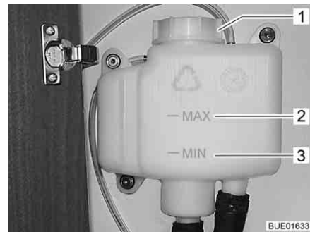
Fig. 259 Compensator reservoir without panel
