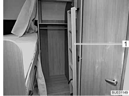
Fig. 17 Access ladder in the wardrobe
