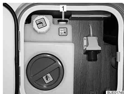
Fig. 232 Water tank (central supply unit)
