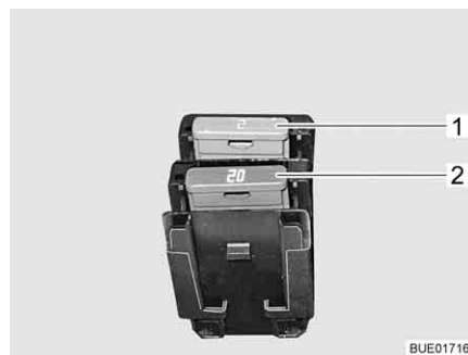
Fig. 168 Fuses for the pull-down bed
