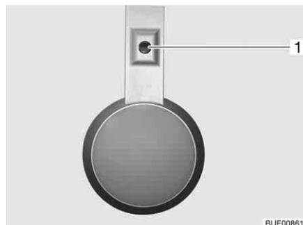
Fig. 61 Lamp, switch mounted directly on the lamp
