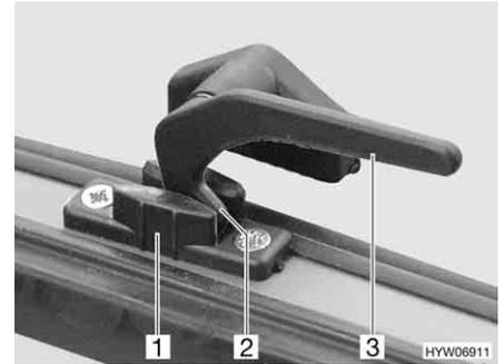
Fig. 78 Catch lever in the "continuous ventilation" position
