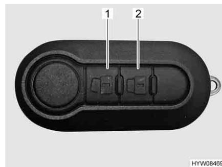
Fig. 42 Remote control for central locking system
