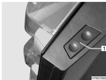
Fig. 195 Release button of the refrigerator door (Dometic 8 series)
