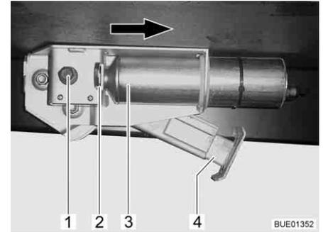
Fig. 38 Electrical steady leg on vehicle
