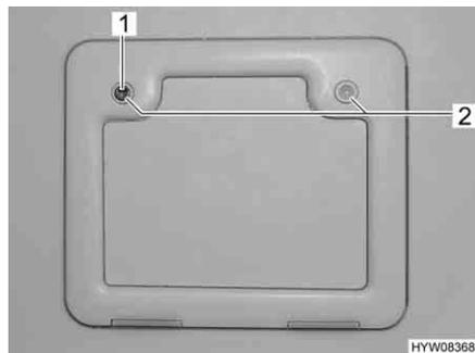
Fig. 224 Flap for the sewage tank
