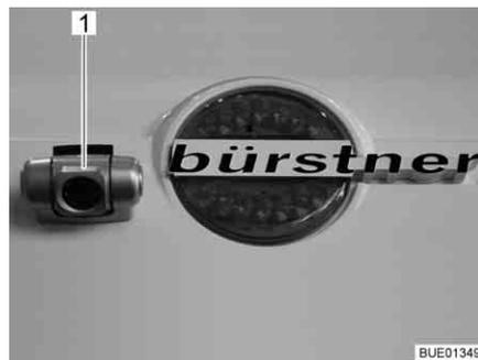
Fig. 20 Reversing camera with infrared illumination (Waeco)
