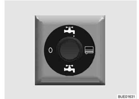
Fig. 205 Operating switch for electrically operated drainage valve
