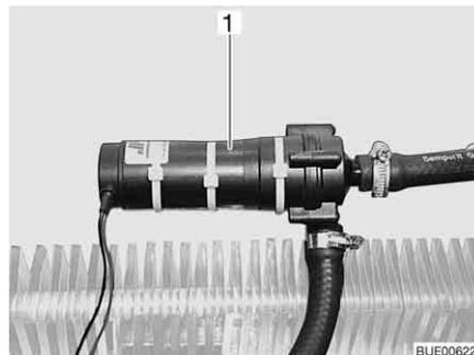
Fig. 171 Auxiliary circulating pump
