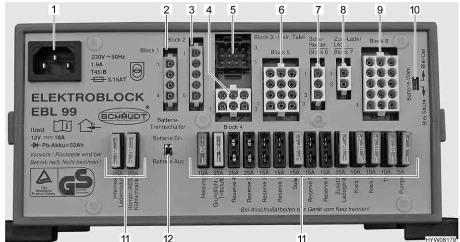
Fig. 133 Transformer/rectifier (EBL 99)
