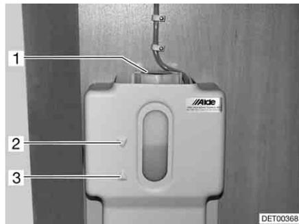
Fig. 227 Compensator reservoir with panel
