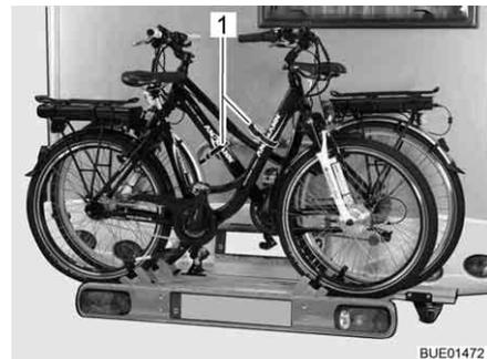
Fig. 6 Positioning of e-bikes
