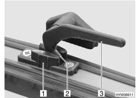
Fig. 83 Catch lever in the "continuous ventilation" position
