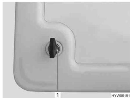
Fig. 51 Push-button lock service flap
