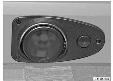
Fig. 236 LED light with switch
