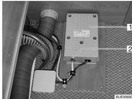
Fig. 174 Transformer for electrical floor warming unit
