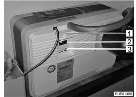
Fig. 138 Connector panel of the fuel cell
