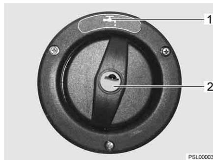
Fig. 53 Cap for the drinking water filler neck
