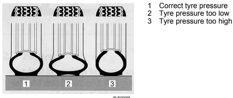
Fig. 251 Contact surface of the tyre
