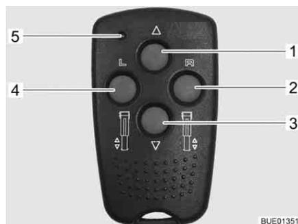
Fig. 36 Remote control for electrical steady legs
