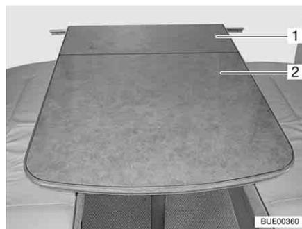
Fig. 104 Insertable table extension
