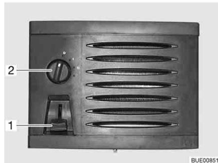
Fig. 173 Operating controls for auxiliary heat exchanger
