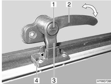
Fig. 77 Catch lever with safety knob in "continuous ventilation" position
