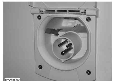
Fig. 143 230 V connection on vehicle
