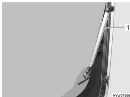
Fig. 81 Hinged window with automatic hinges
