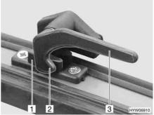
Fig. 57 Catch lever with safety knob in "closed" position
