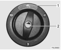
Fig. 149 Cap for the drinking water filler neck
