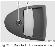
Fig. 31 Door lock of conversion door, outside
