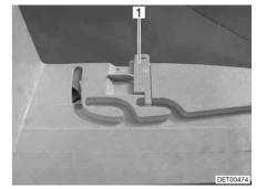
Fig. 69 Heki skylight in ventilation position
