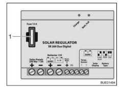
Fig. 117 Solar charge regulator fuse 100 W
