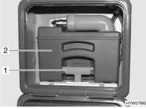
Fig. 172 Flap for the sewage tank
