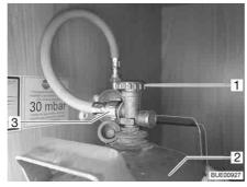
Fig. 96 Gas bottle compartment
