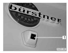
Fig. 12 Reversing camera with infrared illumination (Waeco)
