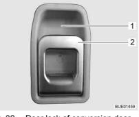
Fig. 32 Door lock of conversion door, inside
