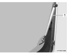
Fig. 59 Hinged window with automatic hinges
