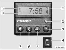
Fig. 133 Operating unit for independent vehicle heater
