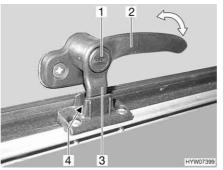
Fig. 60 Catch lever with safety knob in "continuous ventilation" position
