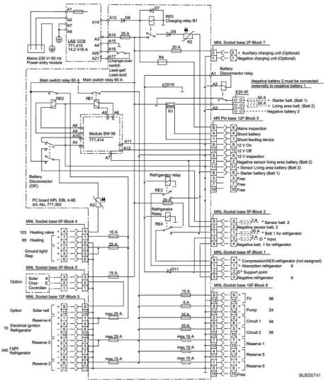
Fig. 123 Circuit diagram, interior (EBL 99)
