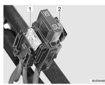
Fig. 112 Fuses on the starter battery
