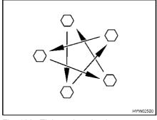
Fig. 183 Tighten the wheel nuts or wheel bolts cross-wise
