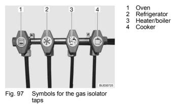
A gas isolator tap (Fig. 97) for every gas device is built into the vehicle.
