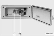
Fig. 98 External gas connection, gas isolator tap closed
