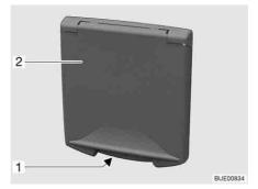
Fig. 39 Flap for the 230 V connection
