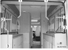
Fig. 83 Bed widening, secured
