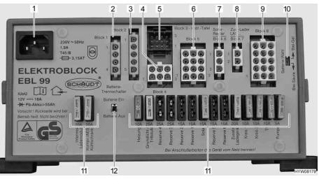
Fig. 105 Transformer/rectifier (EBL 99)
