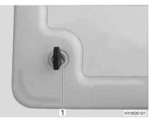
Fig. 38 Push-button lock service flap
