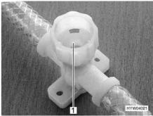
Fig. 158 Drain cock (with rocking lever)
