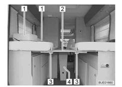
Fig. 85 Bed widening, fitted
