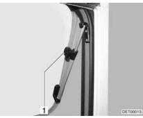
Fig. 54 Hinged window with rotary hinges
