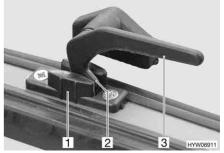
Fig. 56 Catch lever in the "continuous ventilation" position
