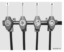
Fig. 126 Symbols for the gas isolator taps
