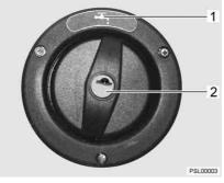
Fig. 40 Cap for the drinking water filler neck
