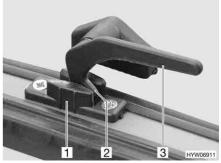
Fig. 77 Catch lever in the "continuous ventilation" position
