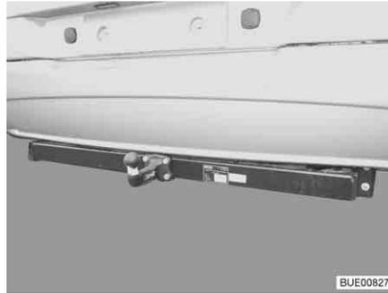
Fig. 10 Engate do reboque
