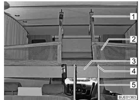
Fig. 115 Pull-down bed complete with applied safety net
