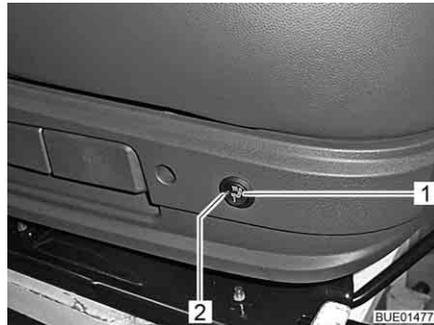
Fig. 25 Switch for seat heater
