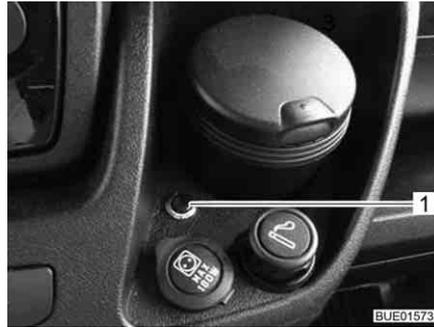
Fig. 35 Push-button to activate remote control
