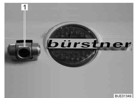
Fig. 22 Reversing camera with infrared illumination (Waeco)
