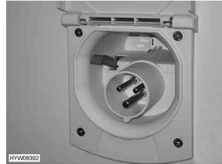
Fig. 179 230 V connection on vehicle
