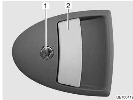
Fig. 43 Door lock of conversion door, outside
