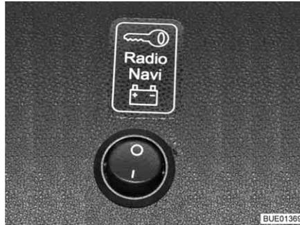
Fig. 169 Selector switch for operating behaviour
