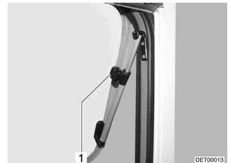
Fig. 92 Skylight with rotary hinges, open
