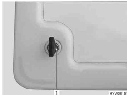
Fig. 48 Push-button lock service flap
