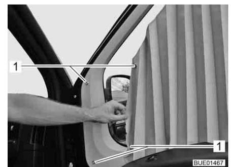
Fig. 81 Fixing of pleated shades
