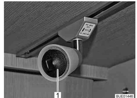
Fig. 300 Suction cup for replacing the lamp
