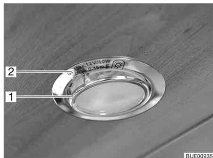
Fig. 296 Recessed halogen light (flat)
