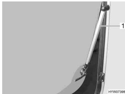
Fig. 75 Hinged window with automatic hinges
