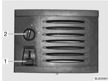
Fig. 210 Operating controls for auxiliary heat exchanger
