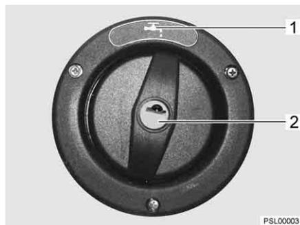
Fig. 50 Cap for the drinking water filler neck
