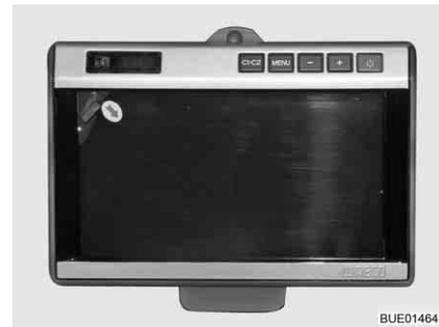
Fig. 24 LCD monitor for reversing camera (Waeco)
