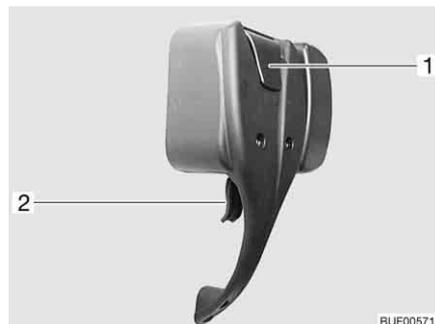
Fig. 42 Door lock of conversion door, inside, locked
