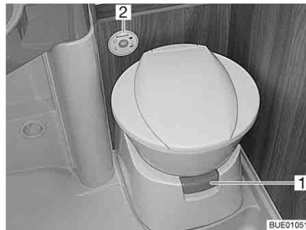
Fig. 285 Toilet bowl with control and operating unit
