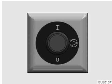
Fig. 209 Operating switch for auxiliary circulating pump
