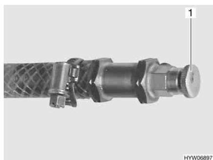
Fig. 290 Bleeding valve of hot-water heater
