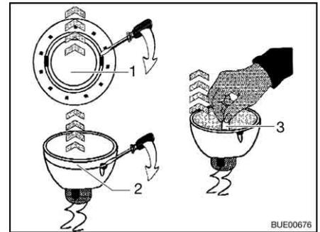
Fig. 298 Changing the halogen bulb
