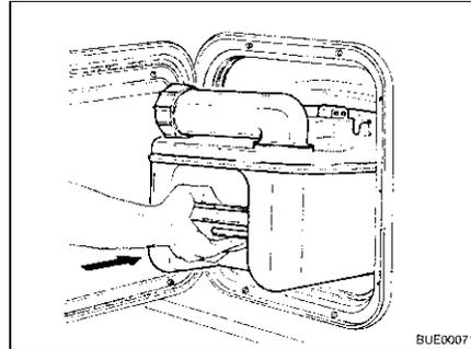
Fig. 272 Inserting the Thetford cassette
