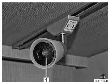
Fig. 303 Suction cup for replacing the lamp
