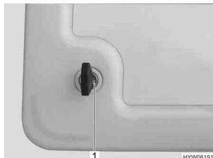
Fig. 64 Push-button lock service flap
