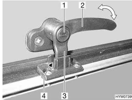
Fig. 91 Catch lever with safety knob in "continuous ventilation" position
