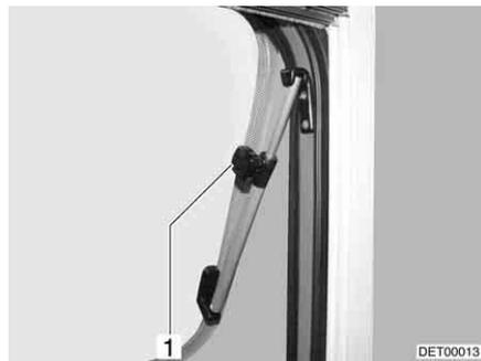
Fig. 90 Hinged window with rotary hinges
