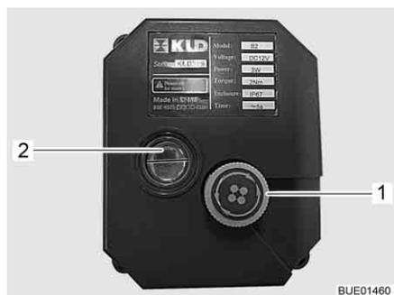
Fig. 236 Electrically operated drainage valve
