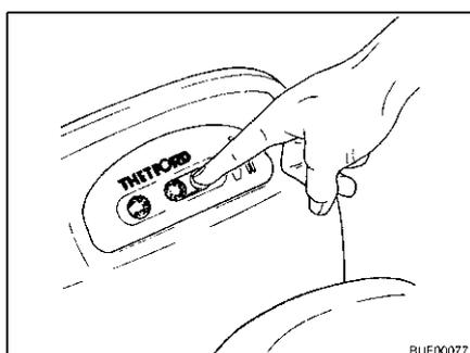
Fig. 254 Closing the sliding trap
