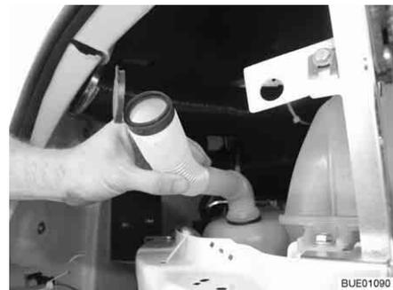
Fig. 43 Filler neck in filling position
