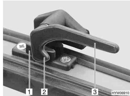
Fig. 89 Catch lever in "closed" position
