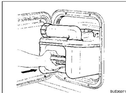
Fig. 259 Inserting the Thetford cassette
