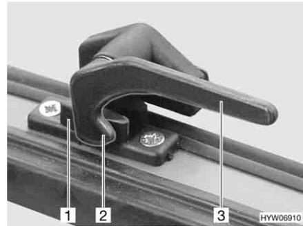
Fig. 94 Catch lever in "closed" position
