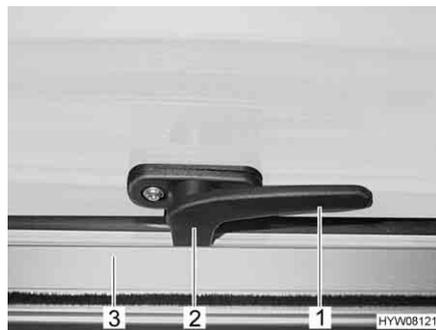
Fig. 99 Catch lever in "closed" position
