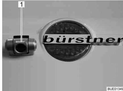
Fig. 16 Reversing camera with infrared illumination (Waeco)
