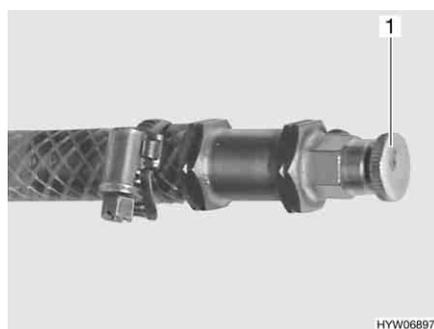
Fig. 282 Bleeding valve of hot-water heater
