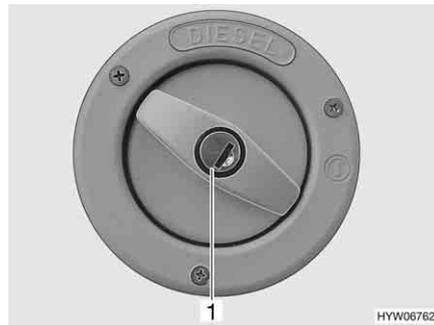
Fig. 44 Cap for the fuel filler neck
