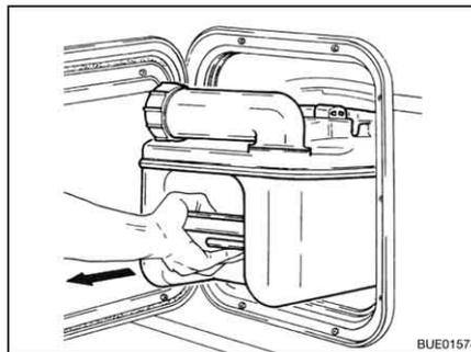
Fig. 244 Removing the Thetford cassette
