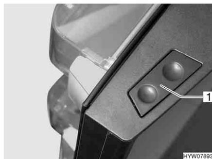
Fig. 225 Release button of the refrigerator door (Dometic 8 series)
