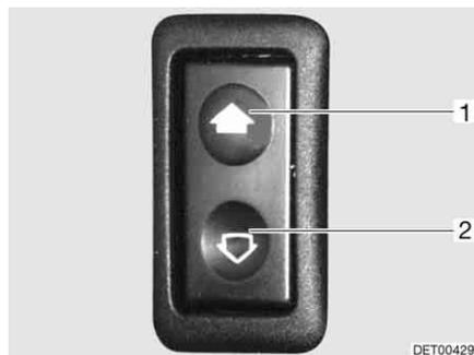
Fig. 28 Switch for electrical window winders
