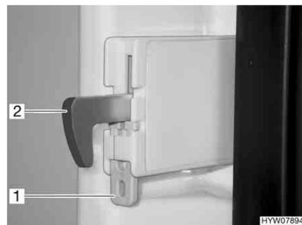
Fig. 226 Lock hook fixture
