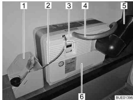
Fig. 160 Fuel cell with tank cartridge
