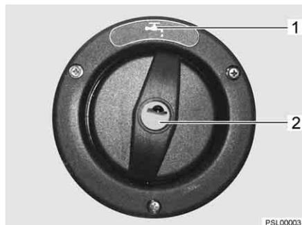
Fig. 66 Cap for the drinking water filler neck
