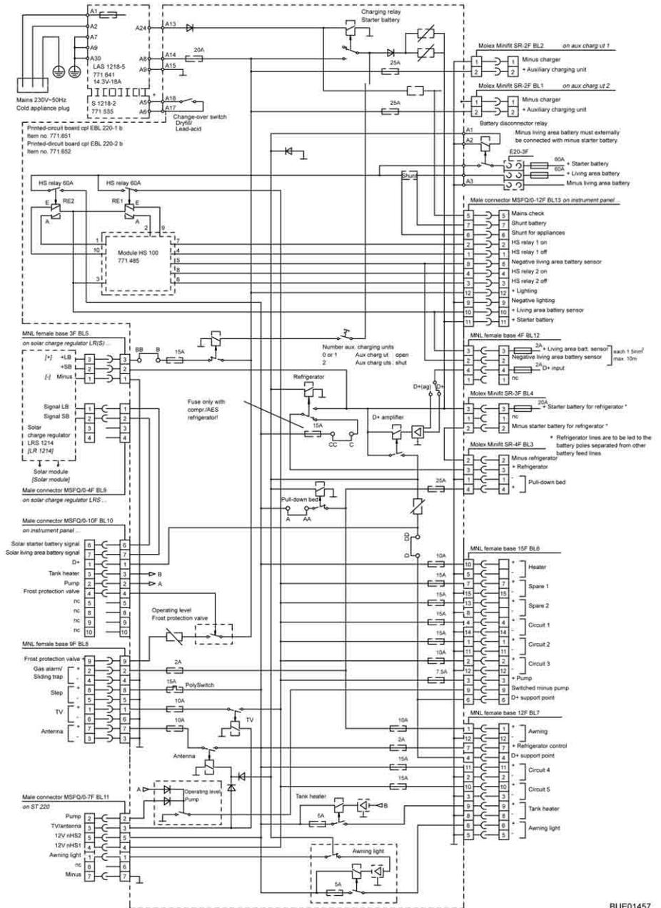
Fig. 181 Circuit diagram, interior (EBL 220)
