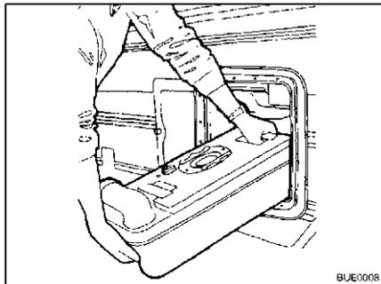
Fig. 261 Removing the Thetford cassette
