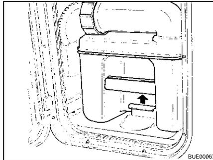
Fig. 260 Pulling the retaining clip
