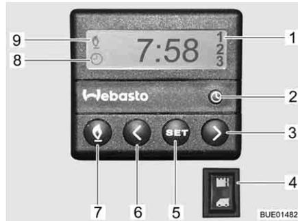
Fig. 201 Operating unit for independent vehicle heater
