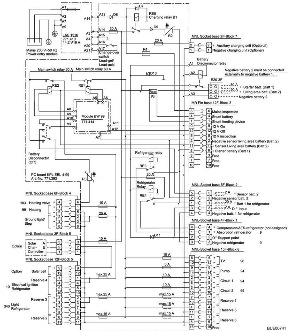
Fig. 180 Circuit diagram, interior (EBL 99)
