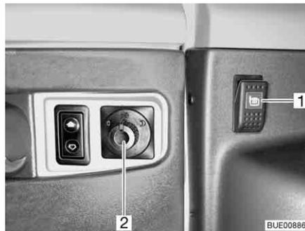
Fig. 31 External mirror adjustment and heater switch
