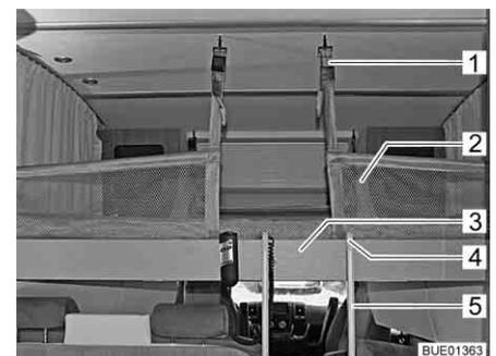
Fig. 125 Pull-down bed complete with applied safety net
