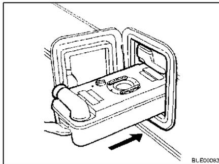
Fig. 264 Inserting the Thetford cassette
