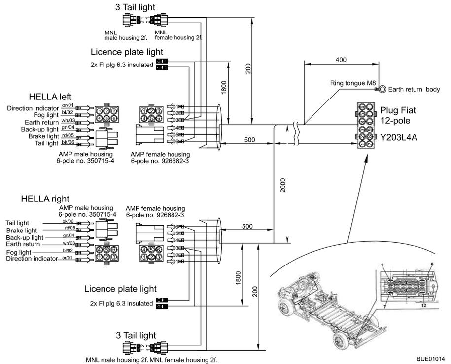
Fig. 186 Circuit diagram, exterior
