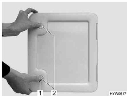
Fig. 273 Flap for sewage tank
