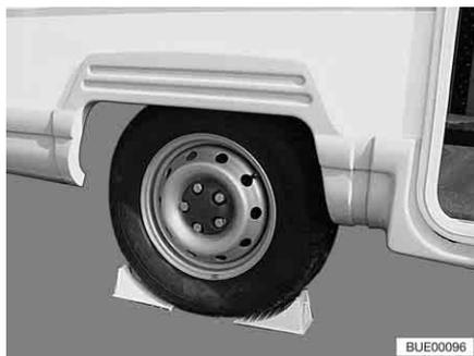
Fig. 310 Securing vehicle
