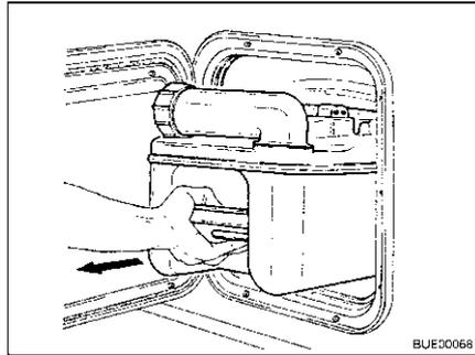
Fig. 269 Removing the Thetford cassette
