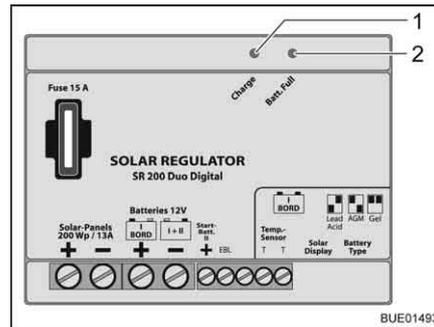
Fig. 164 Solar charge regulator 200 W
