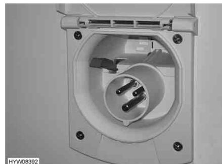
Fig. 166 230 V connection on vehicle
