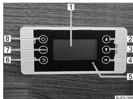
Fig. 162 Operating unit fuel cell
