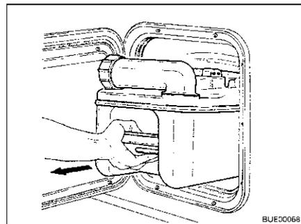
Fig. 256 Removing the Thetford cassette
