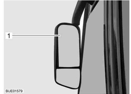
Fig. 30 External mirror (suspended)
