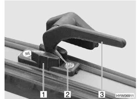
Fig. 92 Catch lever in the "continuous ventilation" position
