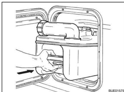
Fig. 247 Inserting the Thetford cassette
