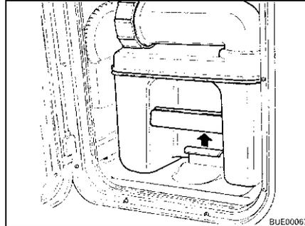
Fig. 243 Pulling the retaining clip
