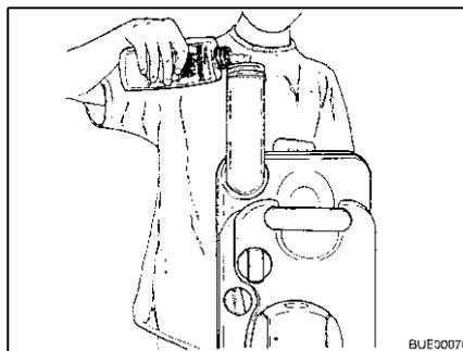
Fig. 276 Filling with sanitary liquid
