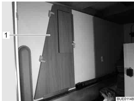
Fig. 15 Bed extension in the rear garage
