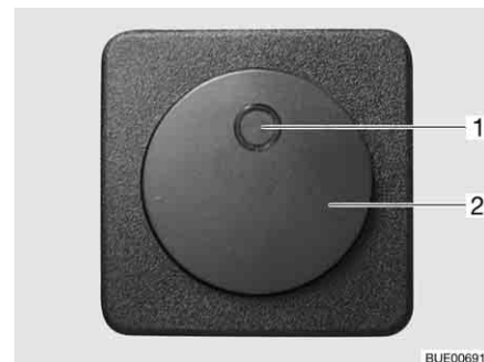
Fig. 169 Switch for electrical floor warming unit
