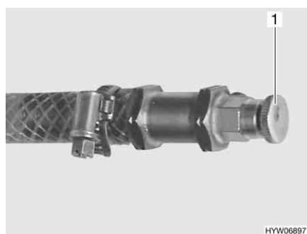
Fig. 251 Bleeding valve of hot-water heater
