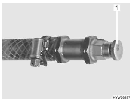
Fig. 278 Bleeding valve of hot-water heater
