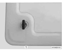
Fig. 35 Push-button lock service flap
