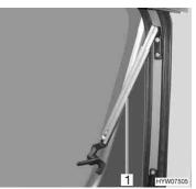
Fig. 59 Catch lever in "closed" position
