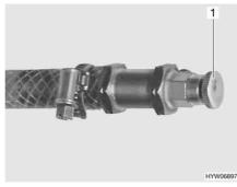
Fig. 197 Bleeding valve of hot-water heater
