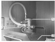
Fig. 97 Gas bottle compartment
