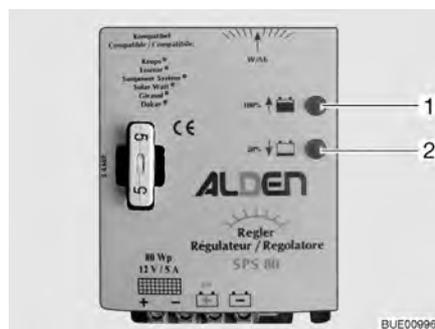
Fig. 108 Solar charge regulator
