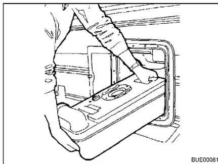
Fig. 176 Removing the Thetford cassette
