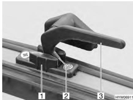
Fig. 59 Catch lever in the "continuous ventilation" position
