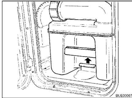
Fig. 175 Pulling the retaining clip
