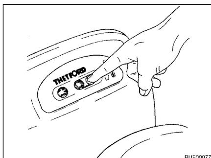
Fig. 186 Closing the sliding trap
