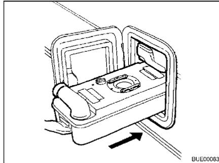
Fig. 179 Inserting the Thetford cassette
