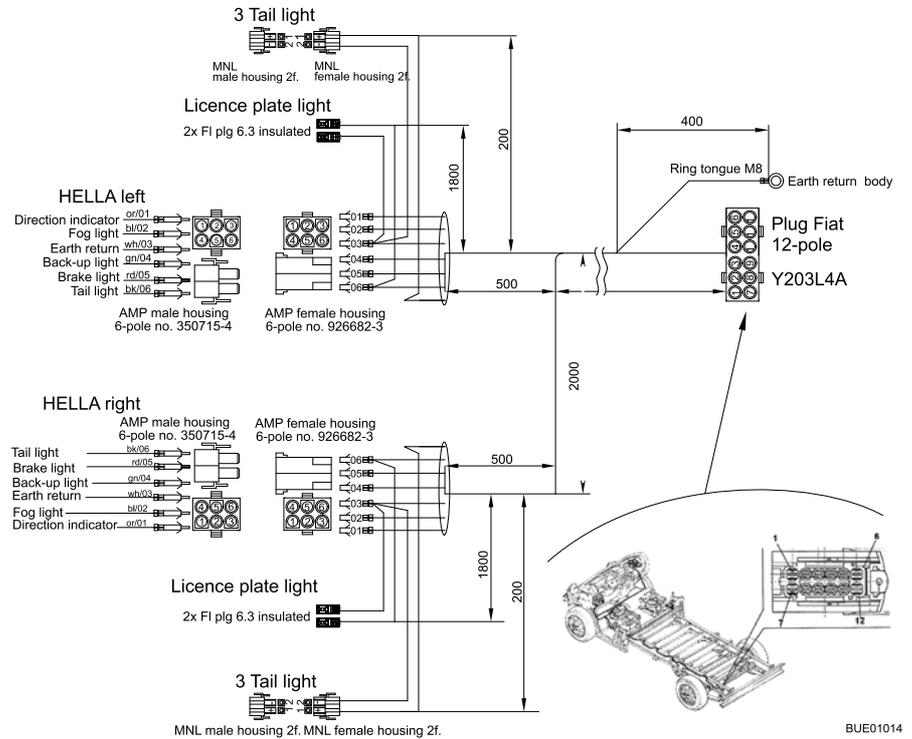
**Fig. 126 Circuit diagram, exterior**
