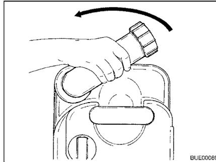
Fig. 177 Turning drainage neck
