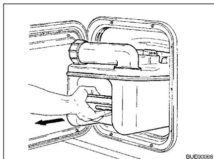
Fig. 187 Removing the Thetford cassette
