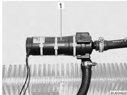
Fig. 135 Auxiliary circulating pump
