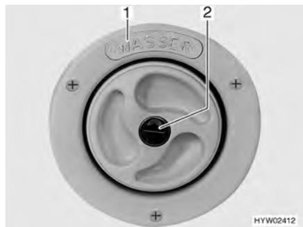
Fig. 34 Cap for the drinking water filler neck
