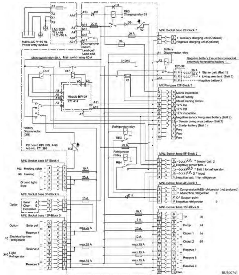
Fig. 121 Circuit diagram, interior (EBL 99)
