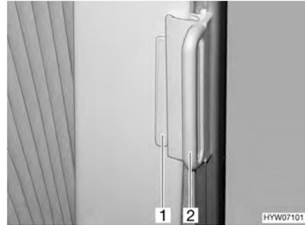
Fig. 63 Roman shades for driver's window and front passenger's window
