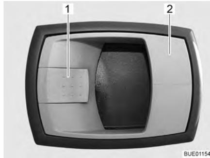
Fig. 27 Door lock of conversion door, inside
