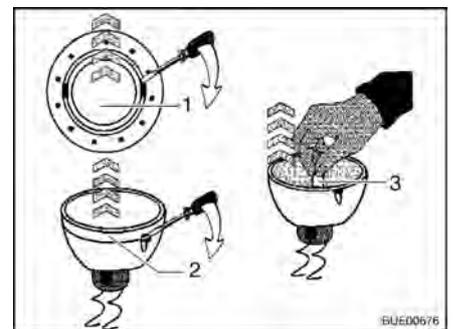
Fig. 203 Changing the halogen bulb
