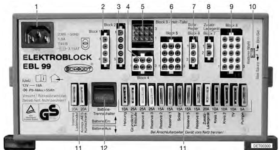
Fig. 102 Transformer/rectifier (EBL 99)
