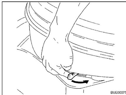
Fig. 183 Operating the sliding trap
