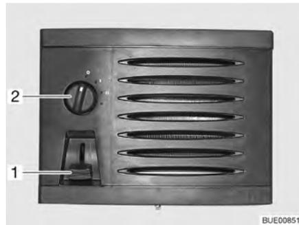
Fig. 139 Operating controls for auxiliary heat exchanger
