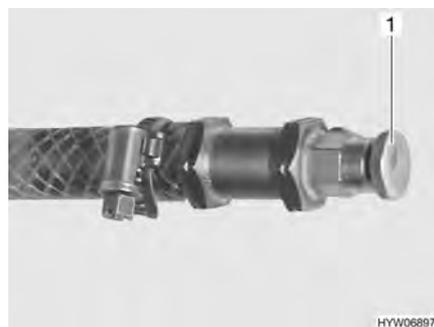
Fig. 197 Bleeding valve of hot-water heater
