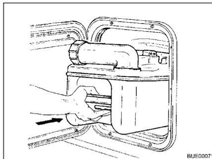
Fig. 190 Inserting the Thetford cassette
