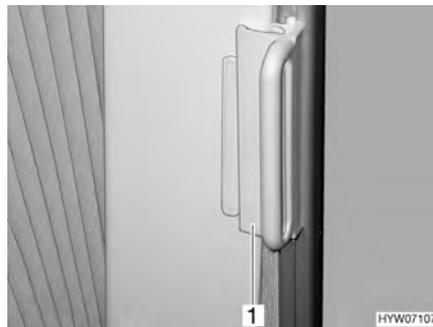
Fig. 21 Locking mechanism for Roman shade on driver's/front passenger's windows
