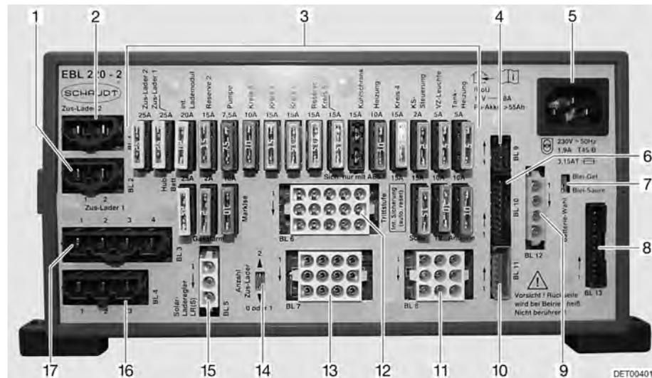
Fig. 103 Transformer/rectifier (EBL 220)
