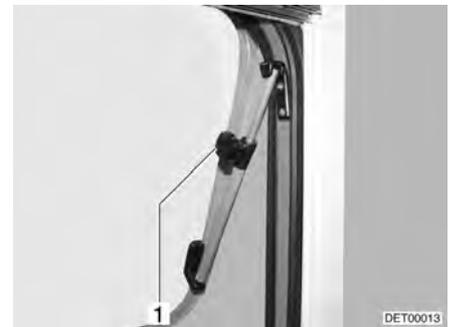
Fig. 55 Hinged window with rotary hinges, open
