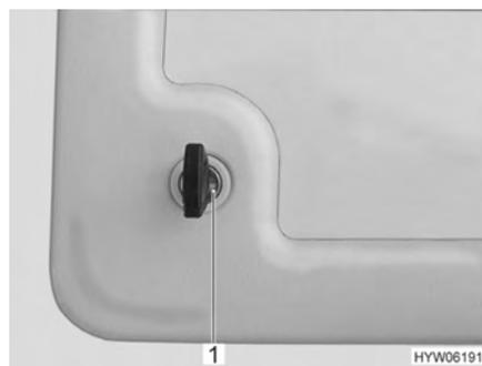
Fig. 32 Push-button lock service flap
