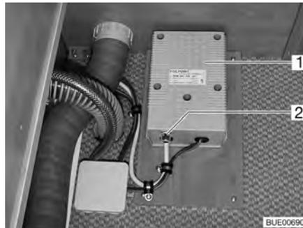
Fig. 137 Transformer for electrical floor warming unit
