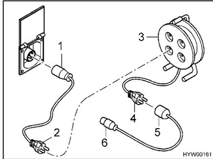
Fig. 109 Connection possibilities 230 V connection
