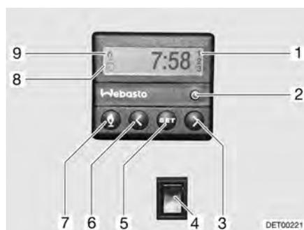
Fig. 140 Operating unit for independent vehicle heater
