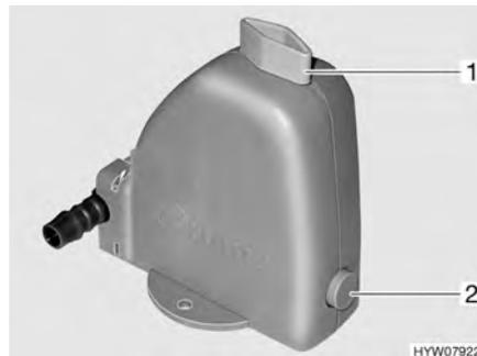
Fig. 146 Safety/drainage valve of the boiler
