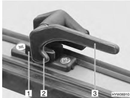
Fig. 57 Catch lever in "closed" position
