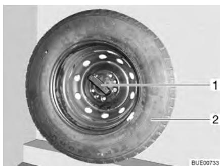
Fig. 213 Spare wheel support in the rear garage
