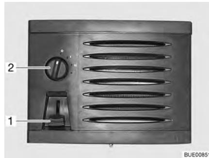
Fig. 143 Operating controls for auxiliary heat exchanger
