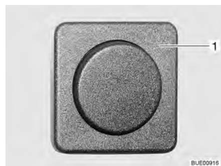
Fig. 53 Toilet compartment lighting, light switch separate from the lamp
