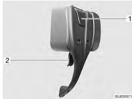
Fig. 37 Door lock of conversion door, inside, locked
