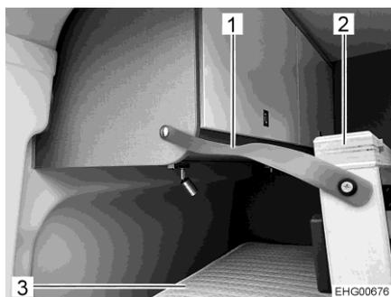
Fig. 35 Bed base retaining strap
