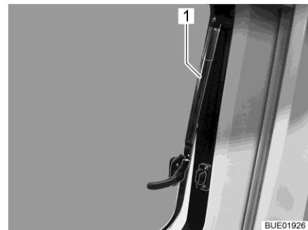
Fig. 13 Hinged window with automatic hinges, open
