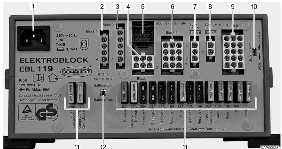
Fig. 45 Transformer/rectifier (EBL 119)
