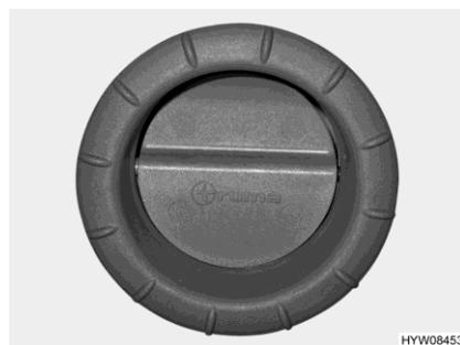
Fig. 54 Air outlet nozzle (hot-air heater)
