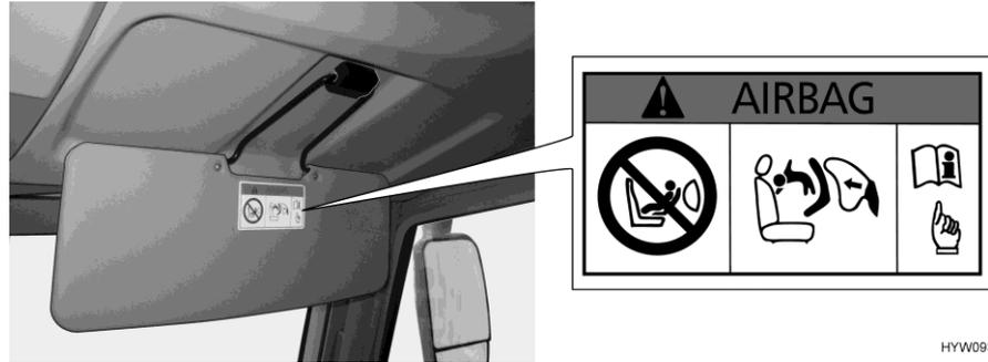
Fig. 5 Warning notice on child restraint system (front passenger's seat sun visor)
