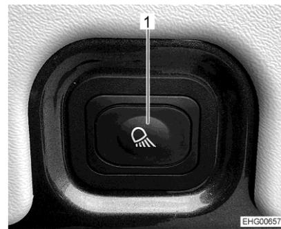
Fig. 33 Switch for lamp
