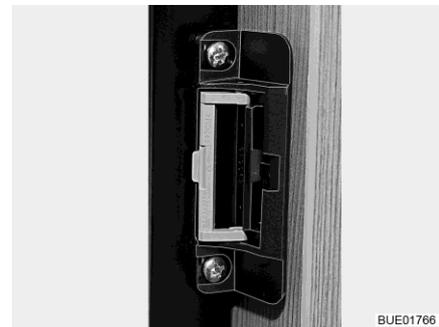
Fig. 64 Locking device in ventilation position
