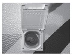
Fig. 80: Fresh water intake port
