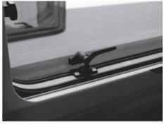
Fig. 104: Continuous ventilation
