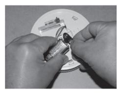
Fig. 101: Replacing the block battery
