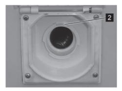
Fig. 91: Fresh water intake port, open
