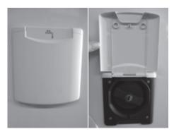
Fig. 23: Fresh water intake port
