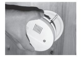
Fig. 100: Removing the housing
