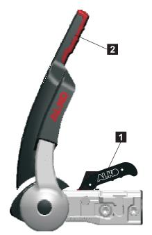
Fig. 5: Tow-ball coupling open
