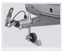
Fig. 147: Securing the support wheel
