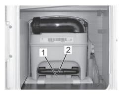
Fig. 133: Waste holding tank in the disposal shaft
