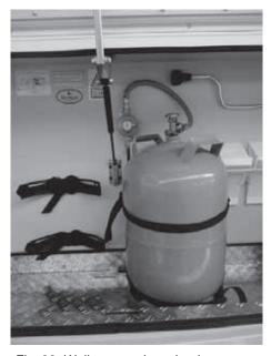
Fig. 98: Wall-mounted gas bottle
