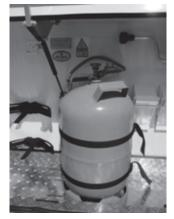
Fig. 96: Gas bottle with pressure reducing valve
