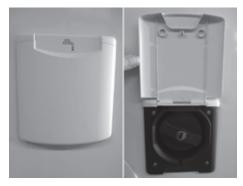
Fig. 89: Fresh water intake port
