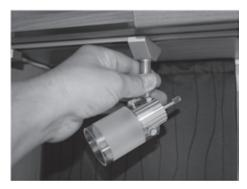
Fig. 131: Adjusting the LED spot light
