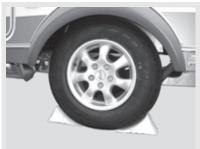
Fig. 148: Securing the vehicle
