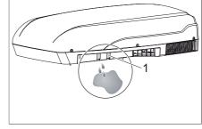
Fig. 176 Lint filter air conditioning unit
