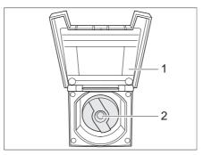
Fig. 152 Cap for the drinking water filler neck
