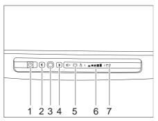
Fig. 146 Operating controls for the refrigerator (Thetford)
