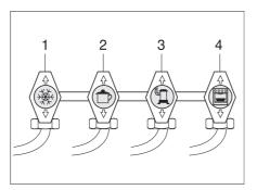
Fig. 88 Symbols for the gas isolator taps
