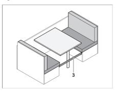
Fig. 69 Inserting the reinforcement panel
