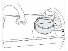
Fig. 120 Regulator for electrical floor warming unit
