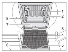
Fig. 43 Skylight with snap latch
