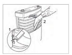
Fig. 111 Mounting the heater cover
