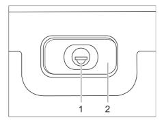
Fig. 31 Flap lock, rectangular, locked
