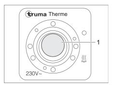
Fig. 134 Operating switch for water heater
