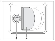
Fig. 29 Flap lock with recessed handle
