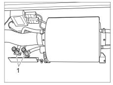
Fig. 135 Drain cock for water heater
