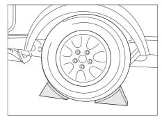
Fig. 186 Securing support wheel
