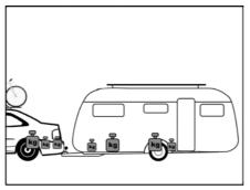
Fig. 4 Correct weight distribution
