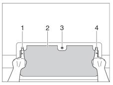
Fig. 32 Flap lock with buttons, locked
