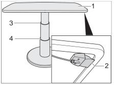
Fig. 59 Lift-off table for the round seating group
