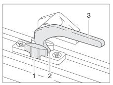
Fig. 40 Catch lever in the "continuous ventilation" position
