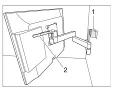
Fig. 62 Holder with jointed arm
