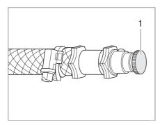
Fig. 173 Bleeding valve of hot-water heater
