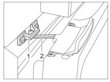
Fig. 148 Refrigerator door in ventilation position (Thetford)
