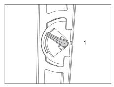
Fig. 22 Variant 1: Door lock of conversion door, inside, locked
