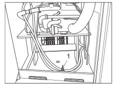
Fig. 133 Position of the drain cocks
