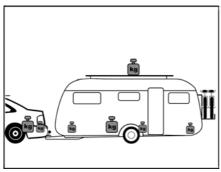
Fig. 3 Incorrect weight distribution
