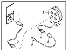
Fig. 98 Connection options for 240 V power connection
