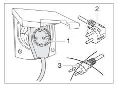
Fig. 99 Connecting an angled connector with socket
