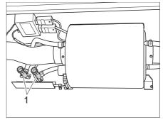
Fig. 131 Position of the drain cocks
