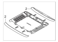
Fig. 174 Lint filter air conditioning unit
