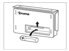
Fig. 110 Changing the batteries
