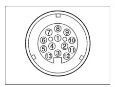
Fig. 104 Top view on socket towing vehicle (thirteen-pin system Jaeger to DIN EN 1648-1)
