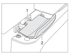
Fig. 147 Lock of refrigerator door, closed (Thetford)
