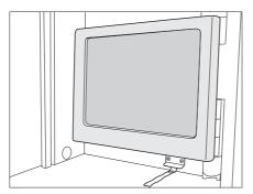
Fig. 7 Holder with jointed arm
