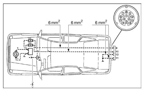
Fig. 105 Towing vehicle installation diagram
