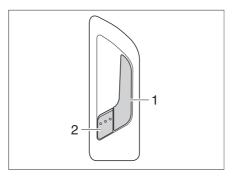
Fig. 25 Door lock of conversion door, inside
