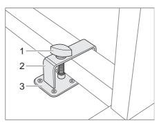
Fig. 55 Latch for swivel table with metal frame
