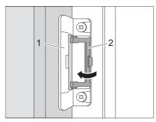
Fig. 150 Locking the ventilation position
