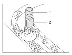
Fig. 130 Drain cocks for Truma boiler
