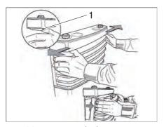
Fig. 109 Removing the heater cover
