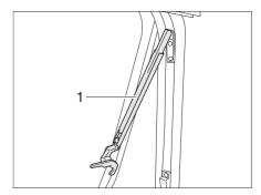
Fig. 39 Hinged window with automatic hinges, open
