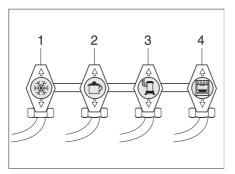
Fig. 106 Symbols for the gas isolator taps
