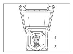
Fig. 89 External gas connection, gas isolator tap closed
