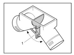
Fig. 115 Circulation fan, adjustment flap in central position
