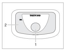
Fig. 158 Flush button/indicator lamp Thetford toilet
