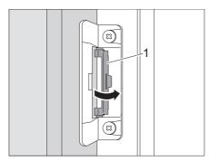
Fig. 151 Turning the latch back to the initial position
