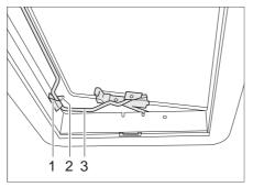
Fig. 50 Heki skylight in ventilation position 2
