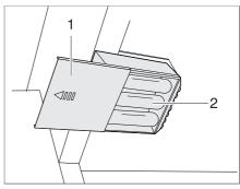
Fig. 183 Wardrobe light with LED, battery compartment opened
