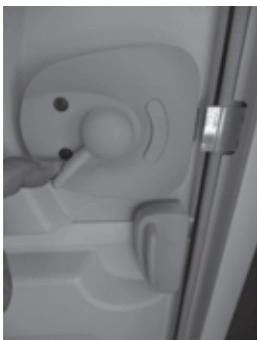
*Fig. 18: Lever down, open door*
