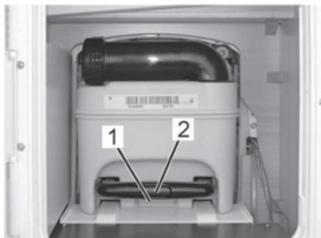
Fig. 133: Waste holding tank in the disposal shaft
