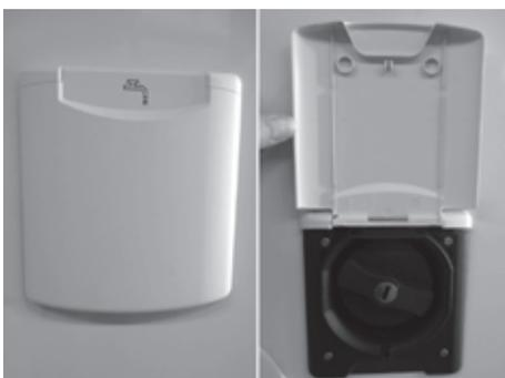
*Fig. 23: Fresh water intake port*
