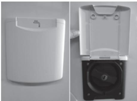
Fig. 89: Fresh water intake port
