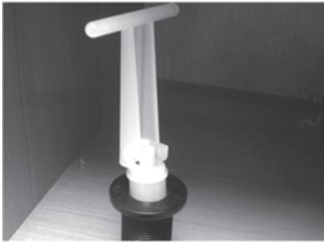
Fig. 92: Drain plug in fresh water tank, open (rocker lever straight)
