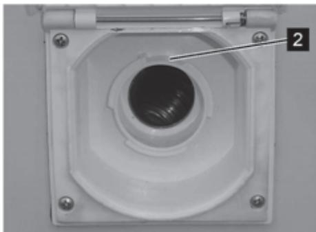
Fig. 91: Fresh water intake port, open
