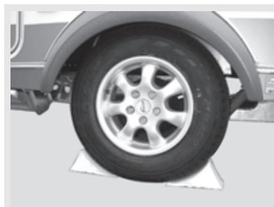
*Fig. 148: Securing the vehicle wheel*
