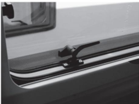
Fig. 104: Continuous ventilation
