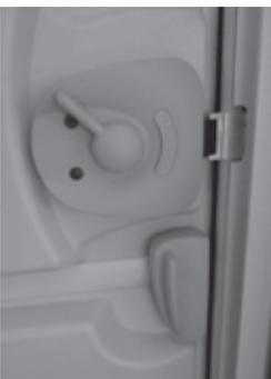
*Fig. 17: Lever up, door lock locked*
