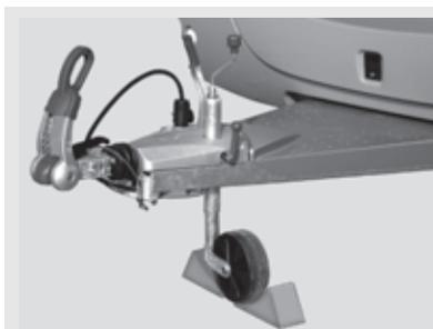
*Fig. 147: Securing the support wheel*
