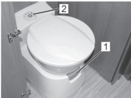
1. For flushing, pull the slide gate (1).
