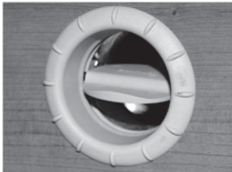
Fig. 77: Hot-air nozzle, open
