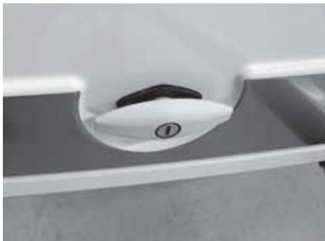
*Fig. 22: Gas locker lock*
