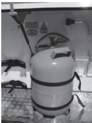
Fig. 96: Gas bottle with pressure reducing valve
