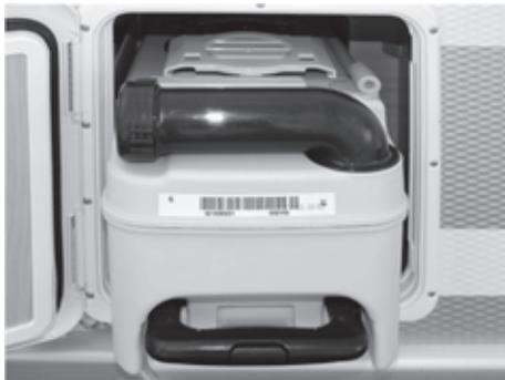
*Fig. 43: Waste holding tank*
