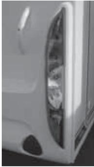
5. Place the glass housing on the reflector insert.
