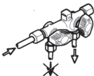
Fig. 75: Shut-off and release position
