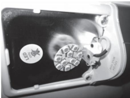
Fig. 151: Replacing LEDs
