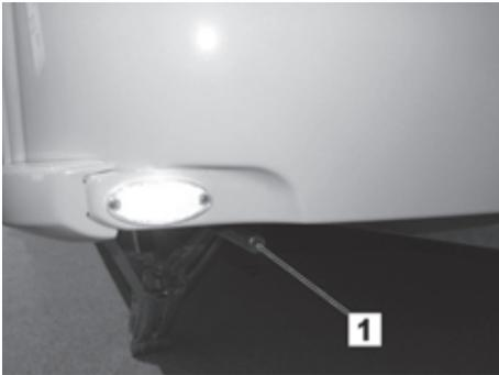
Fig. 10: Hexagon opening (1) for socket wrench
