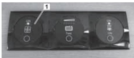
*Fig. 122: On-Off switch of the water heating system*
