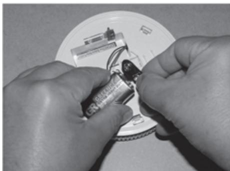
Fig. 101: Replacing the block battery
