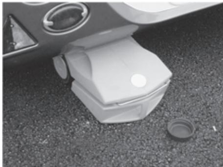
Fig. 94: Wheeled waste water tank
