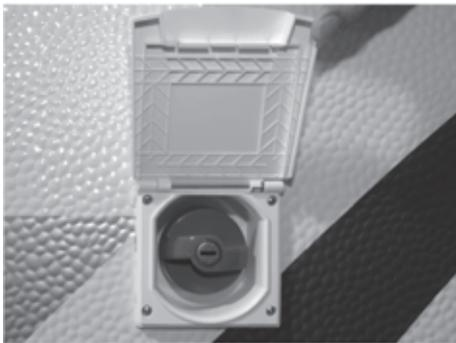
Fig. 80: Fresh water intake port
