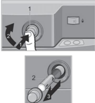
Fig. 145: Changing the batteries of the battery igniter (only if present)
