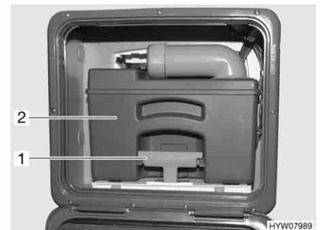
Fig. 196 Sewage tank (example)
