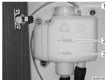
Fig. 213 Compensator reservoir without panel
