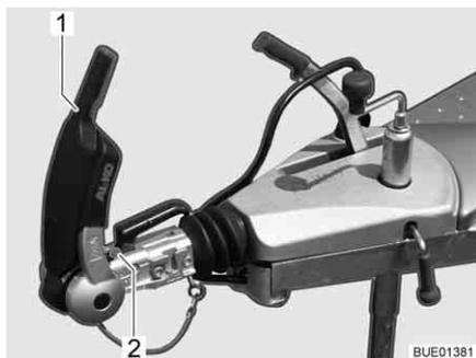
Fig. 210 Display friction pads, front and back
