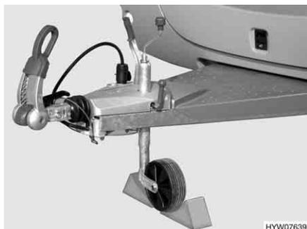
Fig. 230 Securing support wheel
