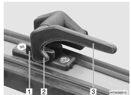
Fig. 57 Catch lever in "closed" position
