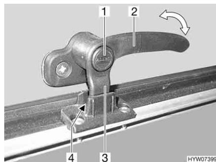
Fig. 60 Catch lever with safety knob in "continuous ventilation" position
