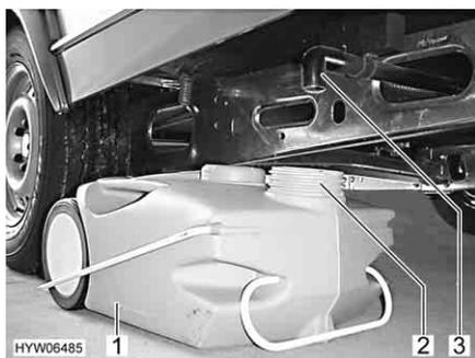
Fig. 25 Waste water tank, mobile
