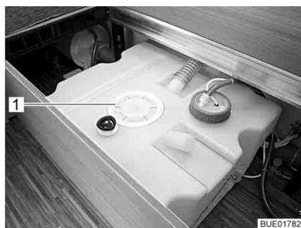
Fig. 207 Cleaning opening of the water tank (example)
