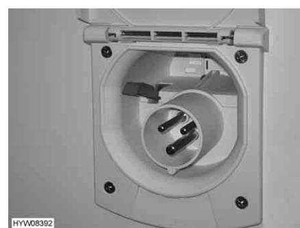
Fig. 125 230 V connection on vehicle
