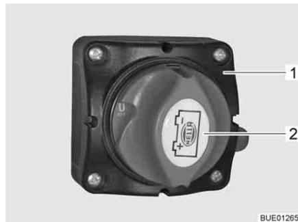
Fig. 118 Battery main switch, "OFF" position
