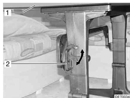
Fig. 73 Swivel table with plastic frame
