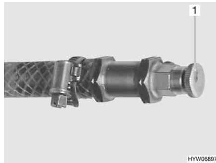
Fig. 214 Bleeding valve of hot-water heater
