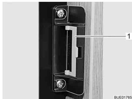
Fig. 186 Locking device in normal position
