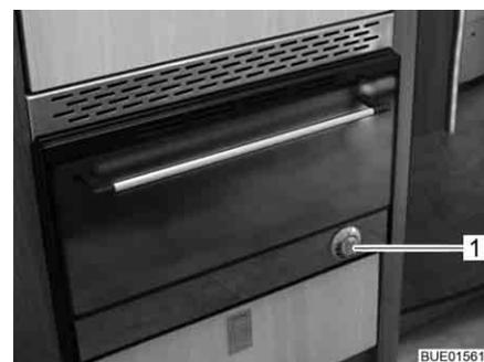
Fig. 170 Gas oven (Dometic)
