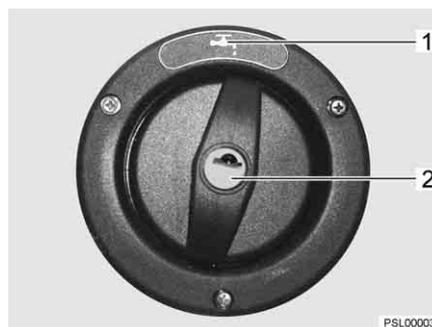
Fig. 38 Cap for the drinking water filler neck
