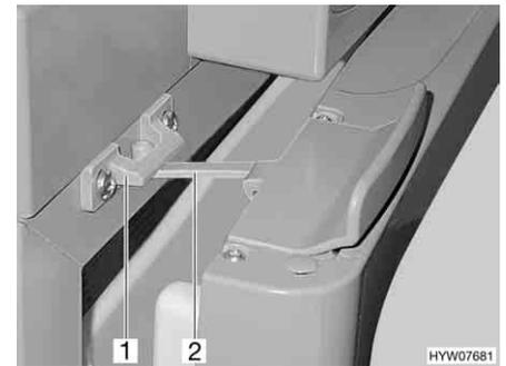
Fig. 185 Refrigerator door in ventilation position (Thetford)
