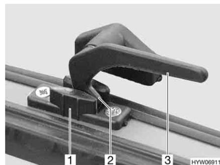
Fig. 61 Catch lever in "continuous ventilation" position
