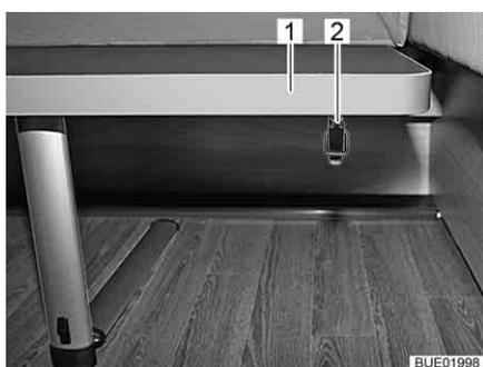
Fig. 16 Clamp fastener
