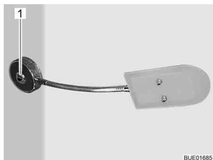
Fig. 47 Interior light, switch mounted directly on the lamp
