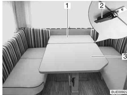
Fig. 74 Suspension table and swivel table
