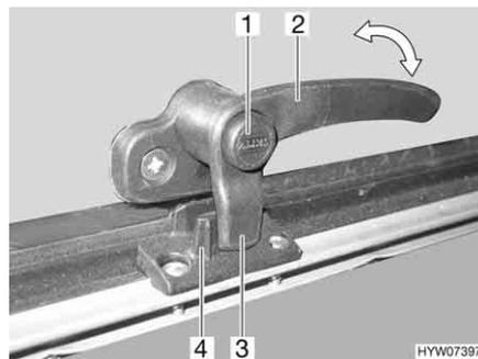
Fig. 56 Catch lever with safety knob in "closed" position
