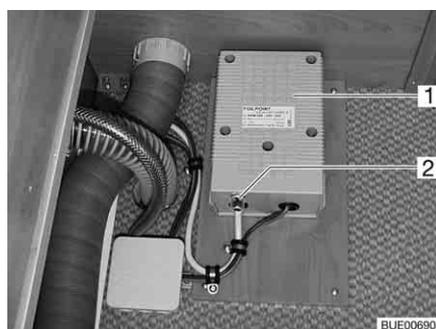
Fig. 154 Transformer for electrical floor warming unit
