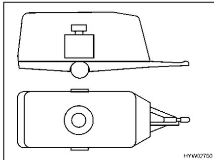
Fig. 9 Correct weight distribution
