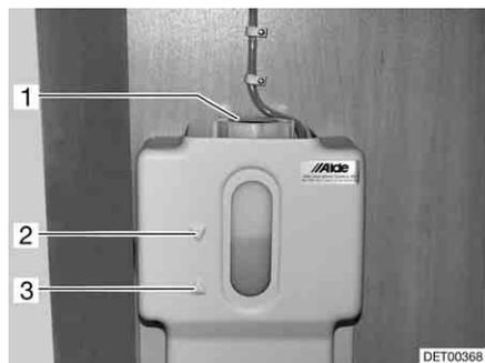
Fig. 212 Compensator reservoir with panel
