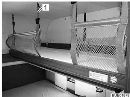
Fig. 90 Folding bed in cabinet with fitted safety net
