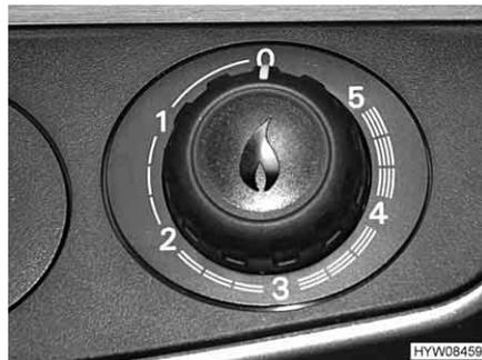
Fig. 143 Hot-air heater control knob
