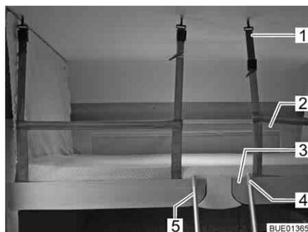
Fig. 85 Pull-down bed complete with applied safety net
