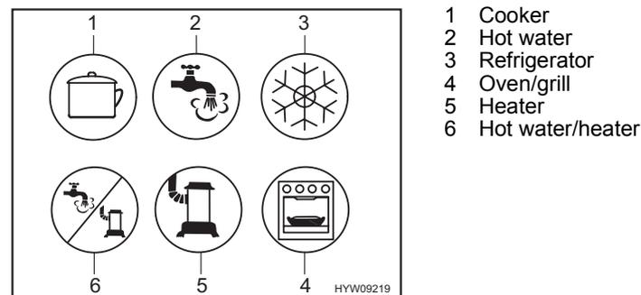
Fig. 137 Possible symbols for the gas isolator taps
