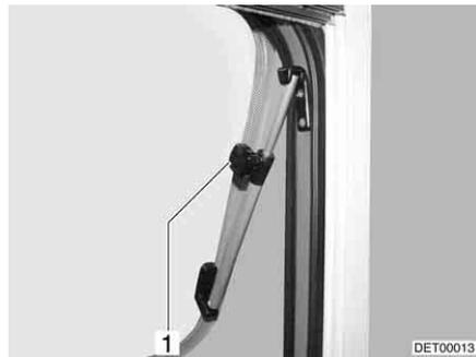
Fig. 58 Hinged window with rotary hinge
