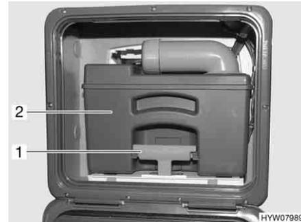
Fig. 206 Sewage tank (example)
