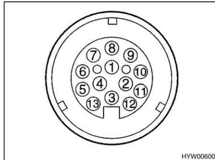
Fig. 131 Contact diagram of the thirteen-pin plug
