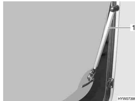
Fig. 59 Hinged window with automatic hinge
