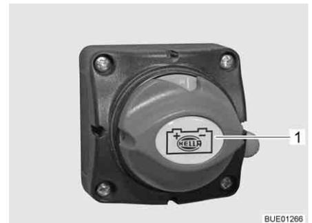
Fig. 119 Battery main switch, "ON" position
