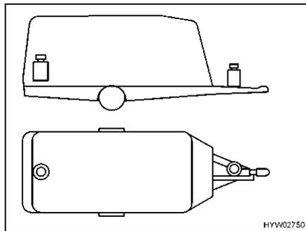
Fig. 8 Incorrect weight distribution
