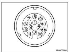
Fig. 132 Contact diagram of the thirteen-pin plug
