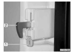
Fig. 174 Lock hook fixture
