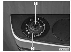
Fig. 141 Knob and rotary switch for fan control
