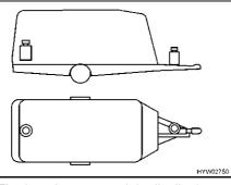
Fig. 8 Incorrect weight distribution
