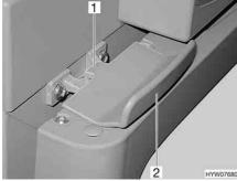
Fig. 177 Lock of refrigerator door, closed (Thetford)
