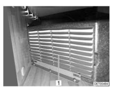
Fig. 200 Air conditioning unit (Truma)
