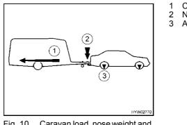
Fig. 10 Caravan load, nose weight and axle load
