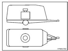
Fig. 9 Correct weight distribution
