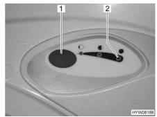
Fig. 196 Flush button/indicator lamp Thetford toilet
