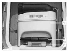
Fig. 187 Flap for sewage tank
