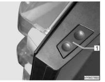
Fig. 173 Release button of the refrigerator door (Dometic 8 series)
