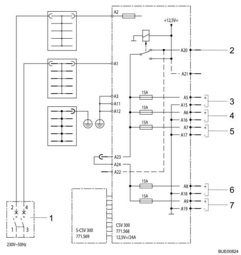
Fig. 136 Circuit diagram, interior (CSV 300)
