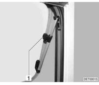
Fig. 59 Hinged window with rotary hinges
