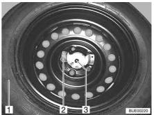
Fig. 229 Spare wheel fixture
