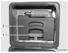
Fig. 197 Flap for the sewage tank
