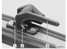
Fig. 62 Catch lever with safety knob in "closed" position
