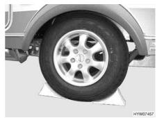
Fig. 223 Securing support wheel
