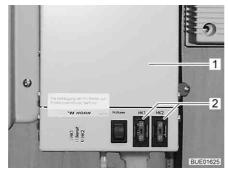
Fig. 130 Heater regulation for waste water pipes
