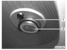
Fig. 211 Recessed halogen light
