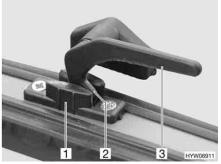
Fig. 66 Catch lever in the "continuous ventilation" position
