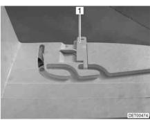
Fig. 72 Heki skylight in ventilation position
