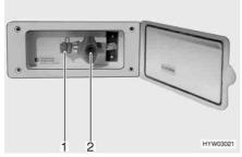
Fig. 116 External gas connection, gas isolator tap closed
