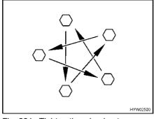
Fig. 221 Tighten the wheel nuts or wheel bolts cross-wise
