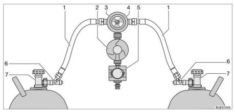
Fig. 117 Crash protection unit switching facility
