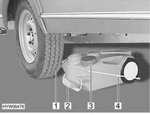
Fig. 184 Waste water tank, mobile
