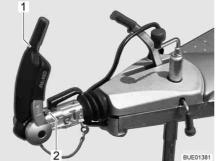
Fig. 203 Display friction pads, front and back
