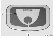
Fig. 193 Flush button/indicator lamp Thetford toilet
