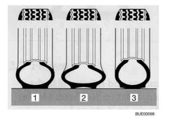
Fig. 234 Contact surface of the tyre
