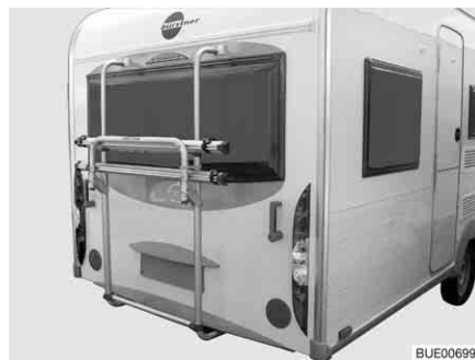
Fig. 13 Bike rack on the rear wall
