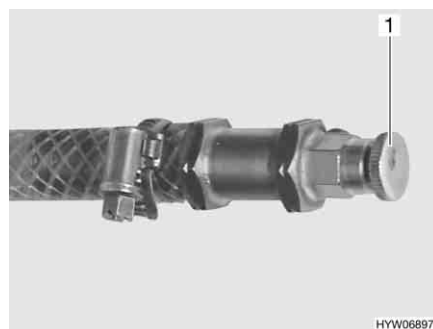
Fig. 195 Bleeding valve of hot-water heater
