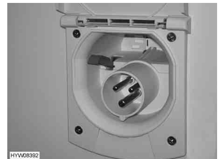
Fig. 95 230 V connection on vehicle
