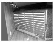
Fig. 206 Air conditioning unit (Truma)
