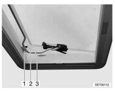
Fig. 63 Heki skylight in ventilation position 2
