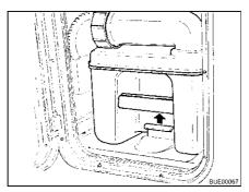
Fig. 171 Pulling the retaining clip
