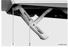
Fig. 17 Corner steady cranked down (variant 1)
