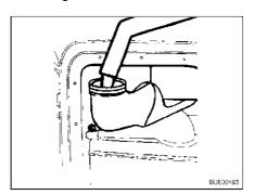
Fig. 188 Filling with fresh water
