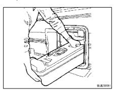
Fig. 172 Removing the Thetford cassette
