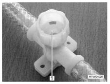
Fig. 144 Drain cock for hot water source
