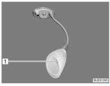
Fig. 223 Halogen spotlight (gooseneck)
