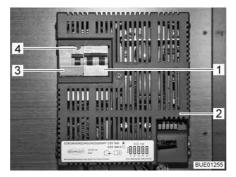
Fig. 115 230 V automatic circuit breaker and FI-switch (CSV 300)
