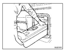
Fig. 191 Removing the Thetford cassette
