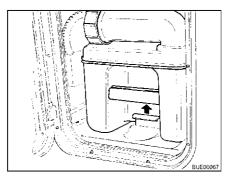
Fig. 190 Pulling the retaining clip
