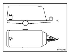
Fig. 6 Incorrect weight distribution
