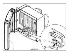
Fig. 125 Removing heater cover
