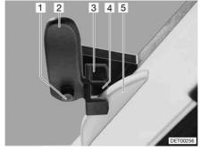
Fig. 62 Heki skylight in ventilation position 1
