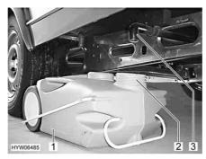
Fig. 20 Waste water tank, mobile
