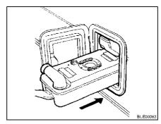
Fig. 175 Inserting the Thetford cassette
