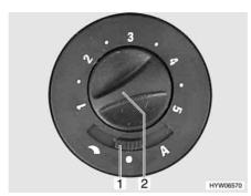
Fig. 128 Operating switch for circulation
