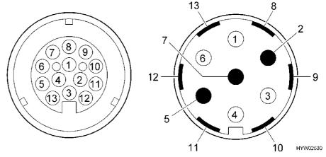
Fig. 116 Contact diagram of the thirteen-pin plug
