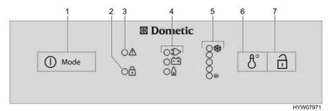
Fig. 153 Operating controls for the refrigerator (Dometic 8 series with MES)
