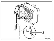
Fig. 127 Heater cover, retaining clips
