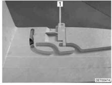
Fig. 60 Ventilation position locking mechanism
