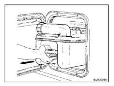
Fig. 183 Removing the Thetford cassette
