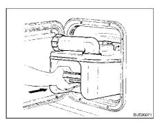
Fig. 202 Inserting the Thetford cassette
