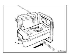
Fig. 194 Inserting the Thetford cassette
