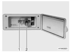
Fig. 102 External gas connection, gas isolator tap closed
