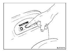
Fig. 181 Opening the sliding trap
