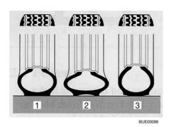
1 Correct tyre pressure2 Tyre pressure too low3 Tyre pressure too high
