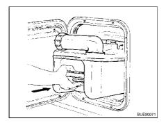
Fig. 186 Inserting the Thetford cassette
