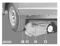
Fig. 168 Waste water tank, mobile
