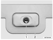
Fig. 28 Flap lock, rectangular, closed
