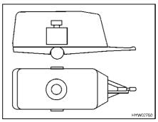
Fig. 7 Correct weight distribution
