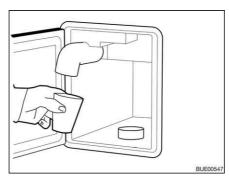
Fig. 204 Emptying the fresh water filler neck
