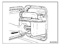
Fig. 199 Removing the Thetford cas-
