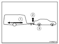
Fig. 8 Caravan load, nose weight and axle load
