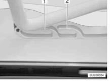
Fig. 59 Heki skylight in ventilation position
