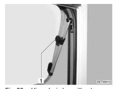
Fig. 50 Hinged window with rotary hinges, open
