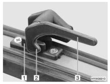
Fig. 49 Catch lever in "closed" position
