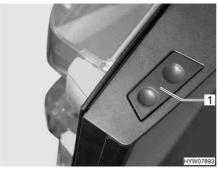
Fig. 158 Release button of the refrigerator door (Dometic 8 series)
