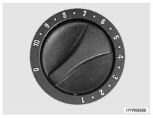
Fig. 124 Heater control knob
