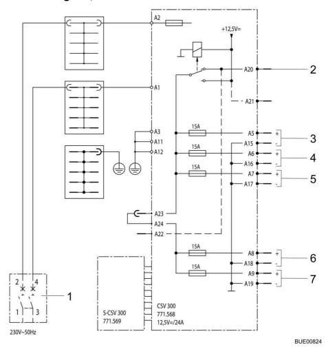
Fig. 120 Circuit diagram, interior (CSV 300)
