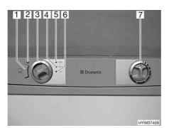
Fig. 152 Operating controls for the refrigerator (Dometic 7 series with FH)
