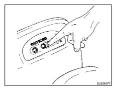
Fig. 182 Closing the sliding trap
