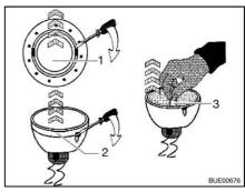
Fig. 217 Changing the halogen bulb
