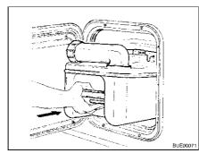
Fig. 169 Inserting the Thetford cassette
