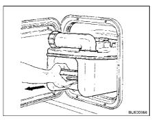
Fig. 166 Removing the Thetford cassette
