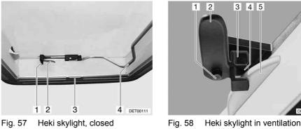
Fig. 58 Heki skylight in ventilation position 1
