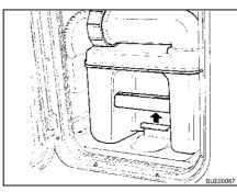
Fig. 154 Pulling the retaining clip
