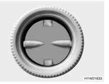
Fig. 107 Air outlet nozzle
