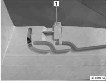
Fig. 55 Heki skylight in ventilation position
