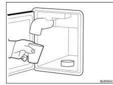
Fig. 187 Emptying the fresh water filler neck
