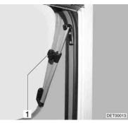
Fig. 45 Catch lever in "closed" position
