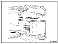
Fig. 185 Inserting the Thetford cassette
