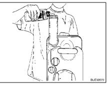
Fig. 157 Filling with sanitary liquid
