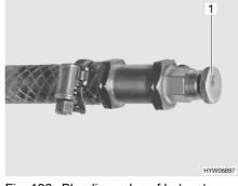
Fig. 196 Bleeding valve of hot-water heater
