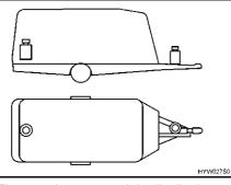
Fig. 7 Incorrect weight distribution
