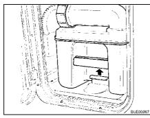
Fig. 173 Pulling the retaining clip
