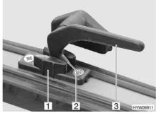
Fig. 50 Catch lever in the "continuous ventilation" position
