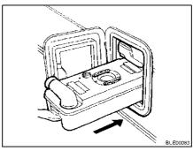
Fig. 177 Inserting the Thetford cassette
