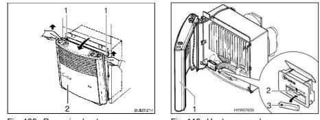
Fig. 109 Removing heater cover
