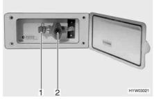
Fig. 86 External gas connection, gas isolator tap closed
