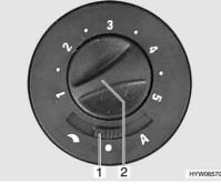
Fig. 112 Operating switch for circulation fan
