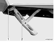
Fig. 18 Corner steady cranked down (variant 1)
