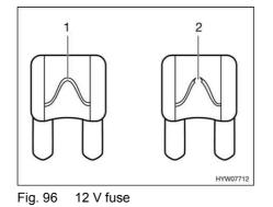
An intact 12 V fuse can be detected by the unbroken fuse element (Fig. 96,1). If the fuse element is broken (Fig. 96,2), change the fuse.
