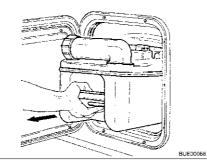
Fig. 182 Removing the Thetford cassette
