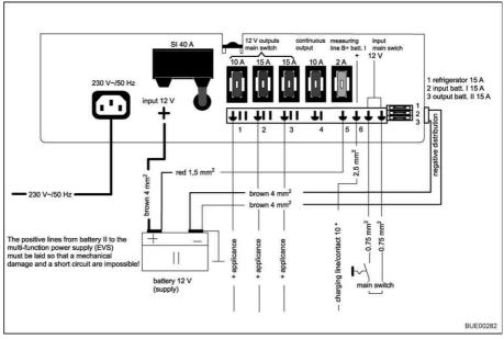
Fig. 93 Connection diagram 2
