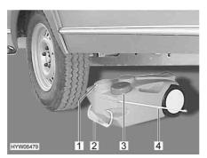
Fig. 151 Waste water tank, mobile
