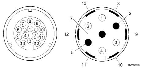
Fig. 100 Contact diagram of the thirteen-pin plug
