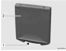
Fig. 31 Flap for the 230 V connection
