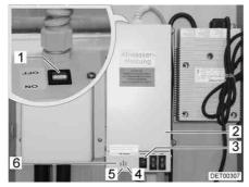
Fig. 116 Transformer with control unit
