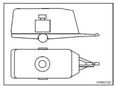
Fig. 8 Correct weight distribution
