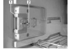
Fig. 144 Locking device in normal position
