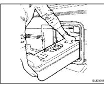
Fig. 155 Removing the Thetford cassette
