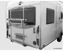
Fig. 11 Bike rack on the rear wall
