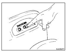
Fig. 165 Closing the sliding trap
