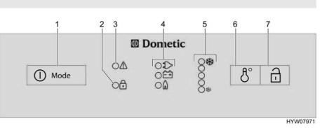
Fig. 137 Operating controls for the refrigerator (Dometic 8 series with MES)
