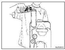
Fig. 176 Filling with sanitary liquid
