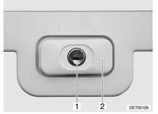
Fig. 29 Flap lock, rectangular, closed
