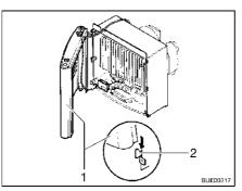
Fig. 111 Heater cover, retaining clips
