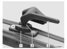
Fig. 47 Catch lever in the "continuous ventilation" position
