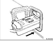
Fig. 158 Inserting the Thetford cassette
