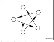
Fig. 207 Tighten the wheel nuts or wheel bolts cross-wise
