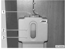
Fig. 195 Compensator reservoir hotwater heater
