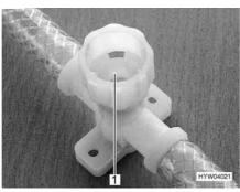
Fig. 124 Drain cock for hot water source
