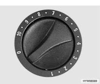
Fig. 108 Heater control knob
