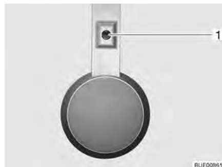
Fig. 45 Toilet compartment lighting, light switch directly on the lamp
