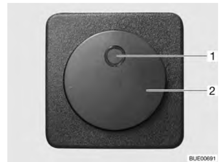
Fig. 124 Switch for electrical floor warming unit
