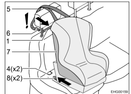
Fig. 4 Fixing with Isofix
