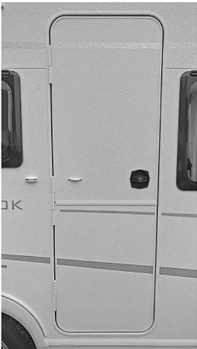
The two-piece entrance door can be locked from the outside with a twist lock that can also be locked from the inside.
