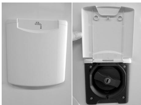
Fig. 96: Fresh water intake port
