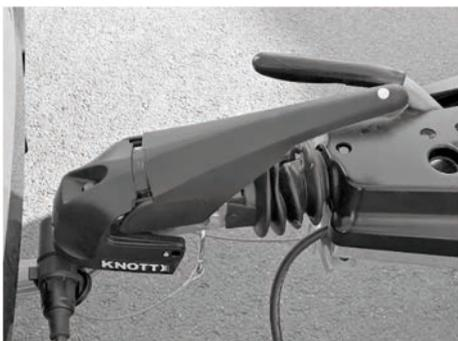
Fig. 10: Tow-ball coupling closed, stabilisation activated
