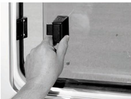
*Fig. 115: Sliding windows***Opening sliding windows**
