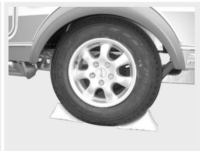
*Fig. 158: Securing the vehicle wheel*
