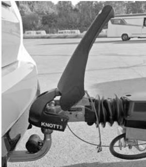
Fig. 13: Tow-ball coupling opened, stabilisation deactivated
