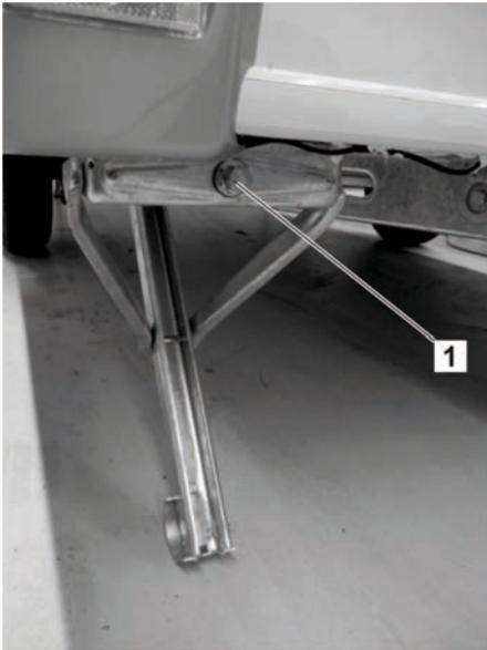
Fig. 15: Hexagonal bolt (1) for socket wrench
