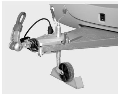
*Fig. 157: Securing the support wheel*
