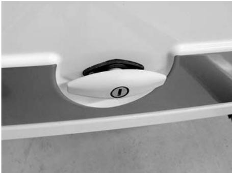
Fig. 31: Gas locker lock
