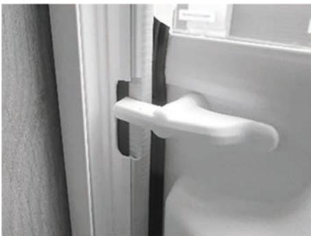
*Fig. 28: Door split, locking handle locked*
