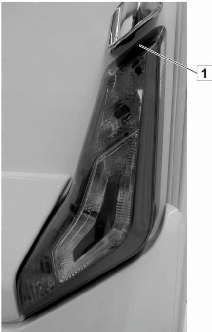
Fig. 167: Undoing the hybrid light
