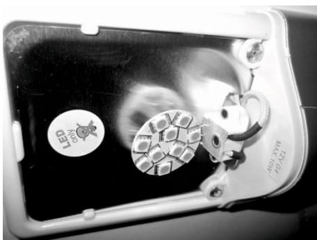
Fig. 161: Replacing LEDs
