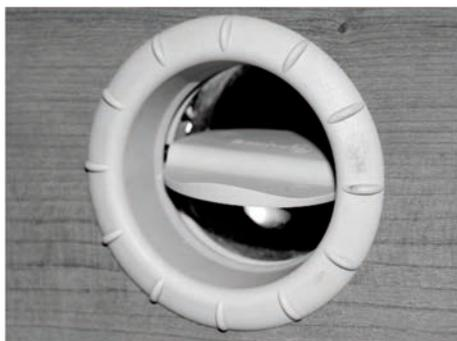
Fig. 84: Hot-air nozzle, open
