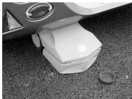
Fig. 101: Wheeled waste water tank
