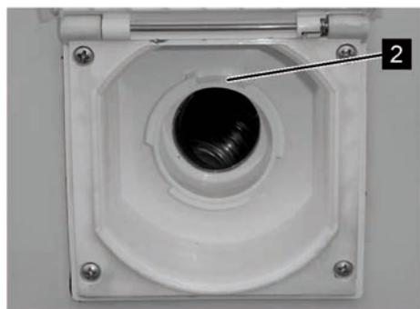
Fig. 98: Fresh water intake port, open
