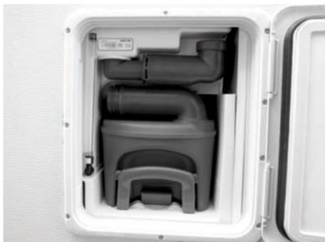
*Fig. 53: Holding tank with flushing water intake port*
