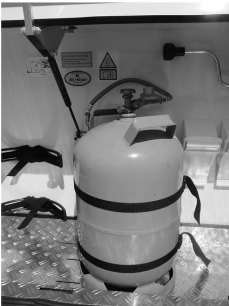
Fig. 76: Open gas locker
