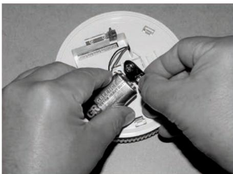
Fig. 111: Replacing the block battery
