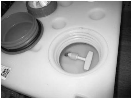
Fig. 99: Drain plug in the fresh water tank
