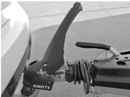
Fig. 9: Tow-ball coupling closed, stabilisation deactivated
