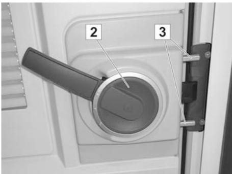
Fig. 22: Door closed and secured
