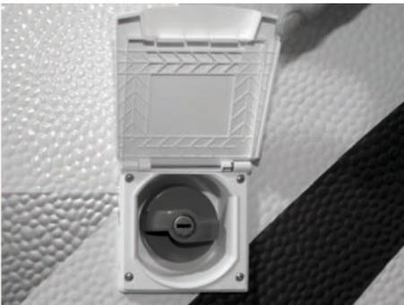
Fig. 87: Fresh water intake port
