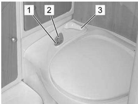
1. Before flushing, open the slide gate of the waste holding tank. Pull the lever (3) forward.
