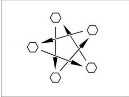
Fig. 156: Always tighten tyre nuts and bolts crosswise
