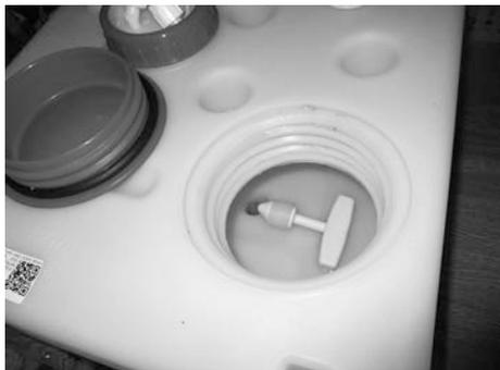
Fig. 91: Drain plug in the fresh water tank
