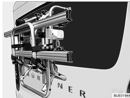
Fig. 1 Bike rack, folded upwards
