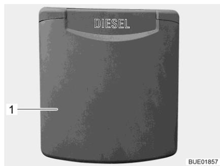
Fig. 38 Fuel filler neck external flap
