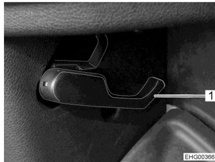
Fig. 35 Release lever for the bonnet (inside the vehicle)
