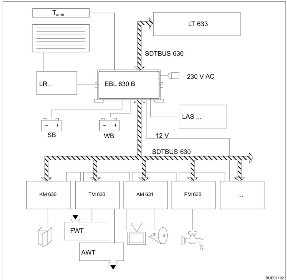
Fig. 119 Block diagram for energy supply of transformer/rectifier EBL 630
