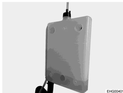
Fig. 156 Compensator reservoir
