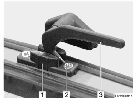
Fig. 83 Catch lever in "continuous ventilation" position
