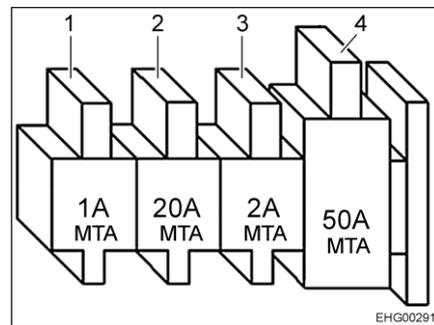
Fig. 114 Fuses (living area battery with charging booster)
