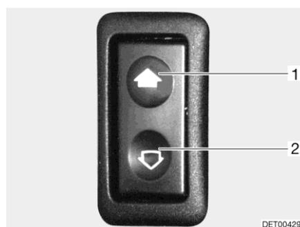
Fig. 25 Switch for electrical window winder
