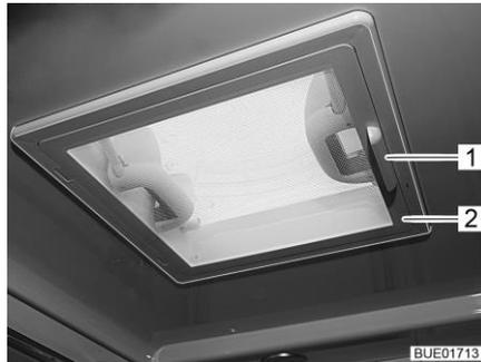
Fig. 91 Skylight with snap latch
