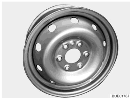
Fig. 169 Steel wheel rim (standard)
