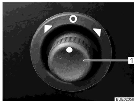
Fig. 27 External mirror adjustment switch
