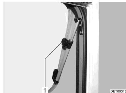
Fig. 80 Hinged window with rotary hinge
