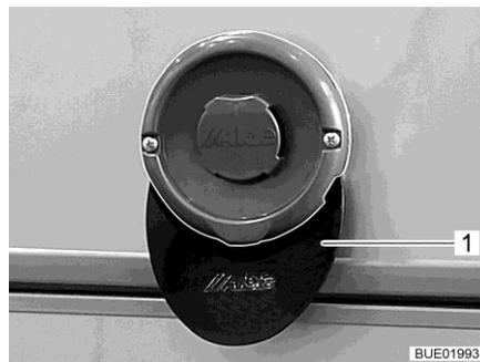
Fig. 133 Flue shield
