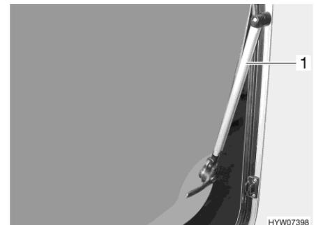
Fig. 81 Hinged window with automatic hinge
