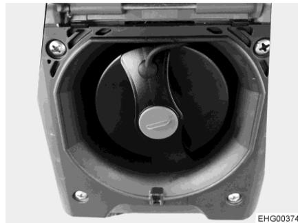
Fig. 59 Cap for the drinking water filler neck
