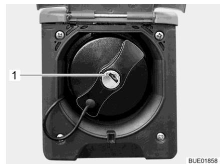
Fig. 39 Cap for the fuel filler neck
