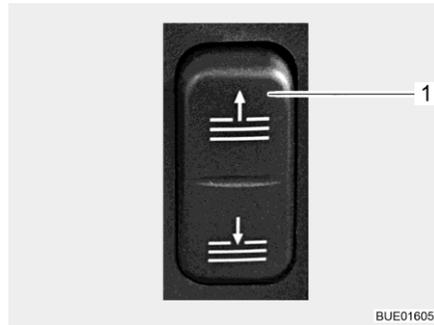
Fig. 32 Switch (electric operation of the Roman shade)
