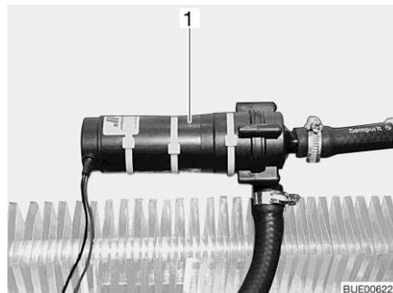
Fig. 128 Auxiliary circulating pump
