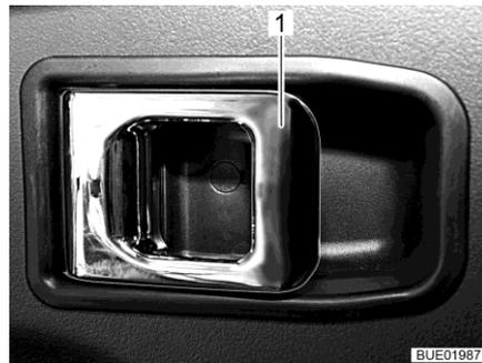
Fig. 50 Door lock (driver's door, inside)
