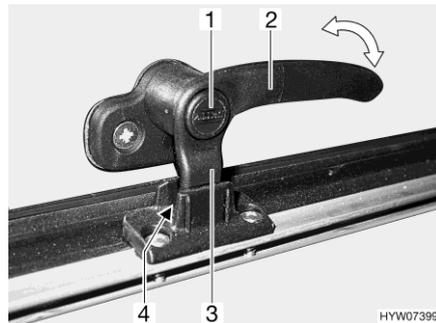
Fig. 82 Catch lever with safety knob in "continuous ventilation" position
