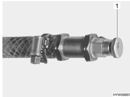
Fig. 157 Bleeding valve of hot-water heater
