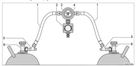
Fig. 40 Gas bottle switching facility with CPU
