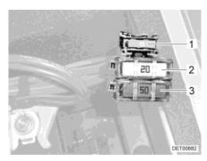
Fig. 50 Fuses on the starter battery
