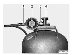
Fig. 43 Gas bottle connection
