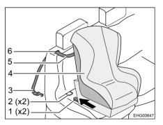
Fig. 7 Fastening with top tether
