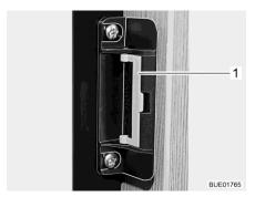
Fig. 63 Locking device in normal position
