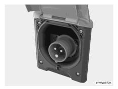
Fig. 48 230 V connection on the vehicle (CEE socket outlet)
