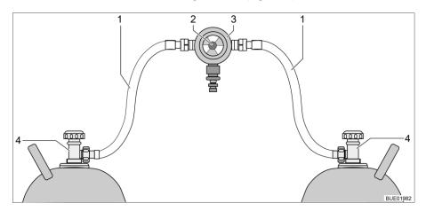
Fig. 39 Gas bottle switching facility
