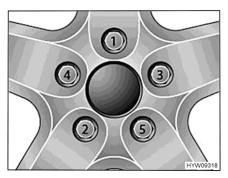
Fig. 82 Tightening the wheel nuts or wheel bolts cross-wise
