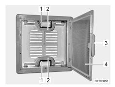
Fig. 20 Skylight with snap latch
