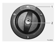
Fig. 66 Cap for the drinking water filler neck
