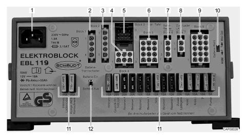
Fig. 45 Transformer/rectifier (EBL 119)
