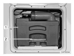
Fig. 78 Flap for the sewage tank
