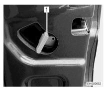
Fig. 10 Handle for opening the rear doors
