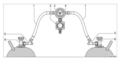
Fig. 4 Gas regulator with CPU and hose break guard
