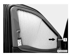
Fig. 18 Side window with folding blind
