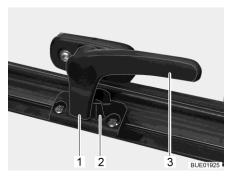
Fig. 12 Catch lever in "closed" position
