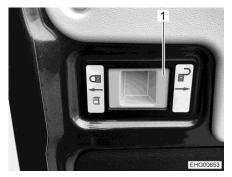
Fig. 11 Handle to release the limitation
