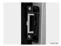
Fig. 64 Locking device in ventilation position
