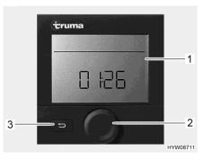
Fig. 55 Operating unit (hot-air heater and boiler)
