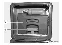
Fig. 304 Sewage tank (example)
