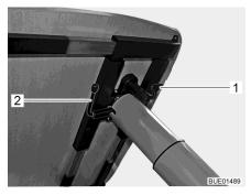
Fig. 132 Adjustment of lift-off table
