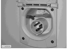
Fig. 208 230 V connection on the vehicle (without service unit)
