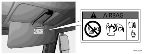
Fig. 21 Warning notice on child restraint system (front passenger's seat sun visor)
