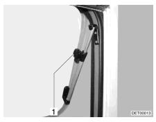
Fig. 99 Hinged window with rotary hinge
