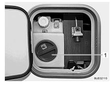
Fig. 307 Cleaning opening of the water tank (service unit)
