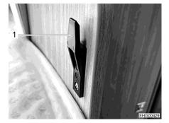
Fig. 188 Fall out protection (window)
