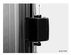
Fig. 104 Sliding window, unlocked
