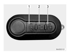
Fig. 50 Multifunctional remote control (3 buttons)
