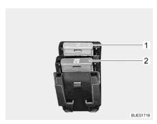
Fig. 215 Fuses for the pull-down bed
