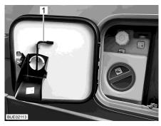
Fig. 286 Service flap with square spanner
