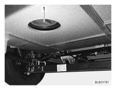
Fig. 308 Cleaning opening (waste water tank)
