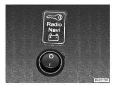
Fig. 202 Selector switch for power supply
