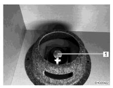
Fig. 86 Active docking station on shelf above the driver's cabin
