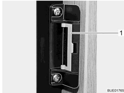
Fig. 244 Locking device in normal position
