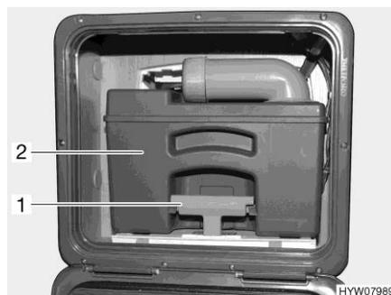
Fig. 278 Sewage tank (example)
