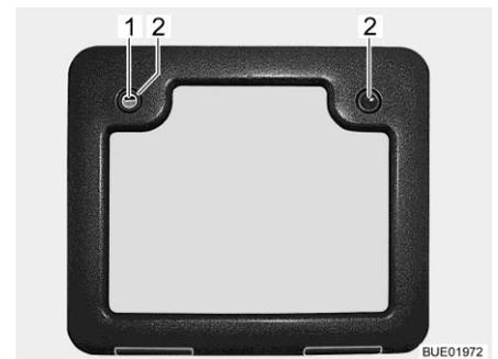
Fig. 79 Service flap push-button lock (alternative)
