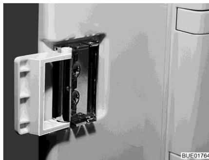
Fig. 248 Locking device in ventilation position
