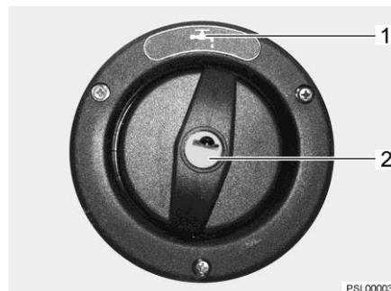
Fig. 81 Cap for the drinking water filler neck
