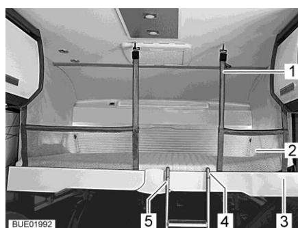
Fig. 139 Pull-down bed complete with applied safety net
