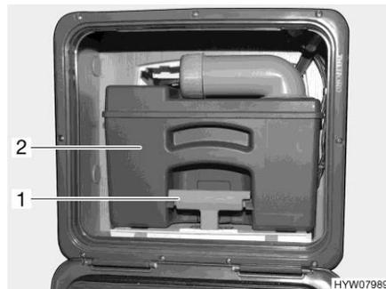
Fig. 269 Sewage tank (example)
