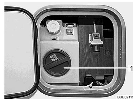
Fig. 281 Cleaning opening of the water tank (service unit)
