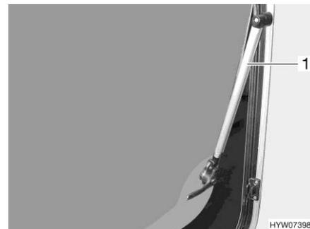
Fig. 112 Hinged window with automatic hinge
