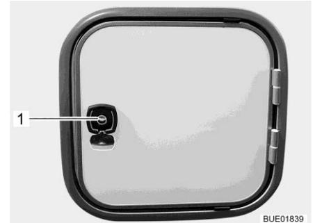
Fig. 277 Flap for sewage tank (alternative)
