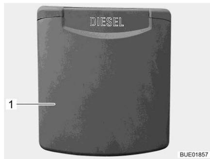
Fig. 54 Fuel filler neck external flap
