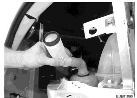
Fig. 53 Filler neck in filling position
