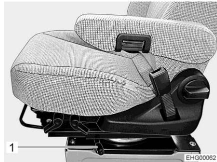
Fig. 22 Release lever for rotating
