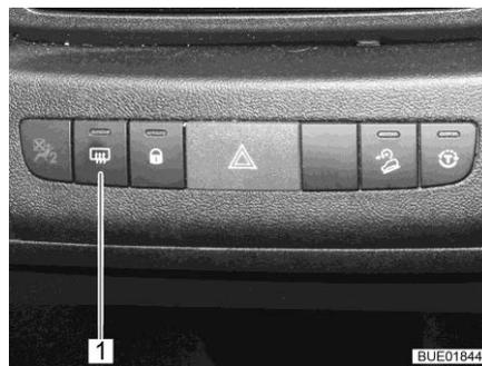
Fig. 41 External mirror heater switch
