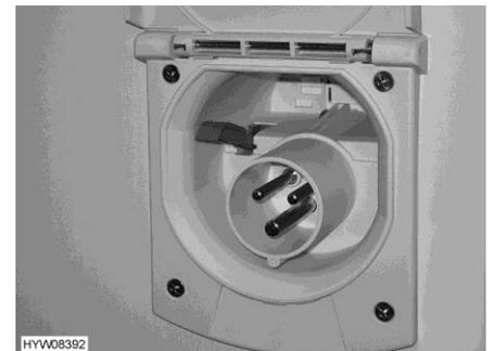
Fig. 189 230 V connection on the vehicle (without service unit)
